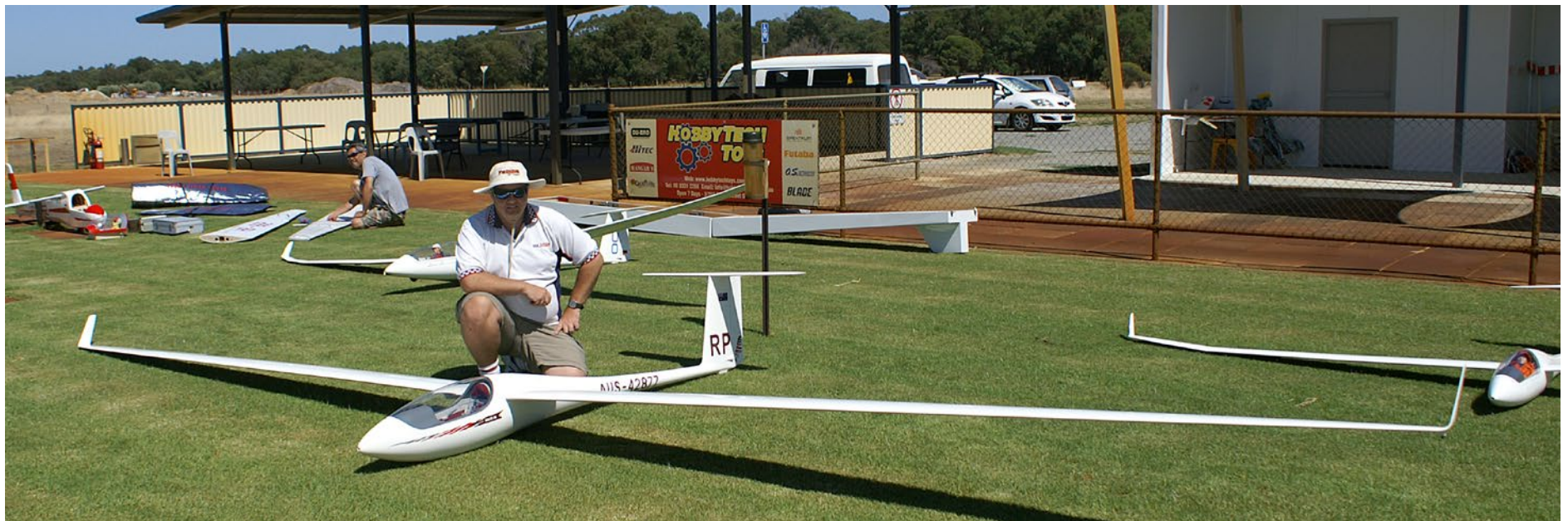
IMAC Elite Comp' pilot and part time "glider guider" Roman Pasznicki and his 7m Let Models ASH 31MI with Up&Go self-launch system, Futaba 18MZ 2.4ghz radio system. < http://www.letmodel.cz/gallery-ash31.htm >
