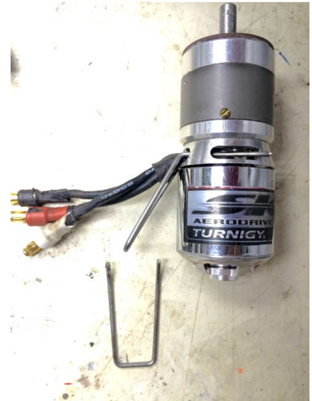
A piece of 0.047" music wire bent into a "U" shape. The two legs fit into the front cooling slots of the motor and go all the way through and out the bottom slots.
