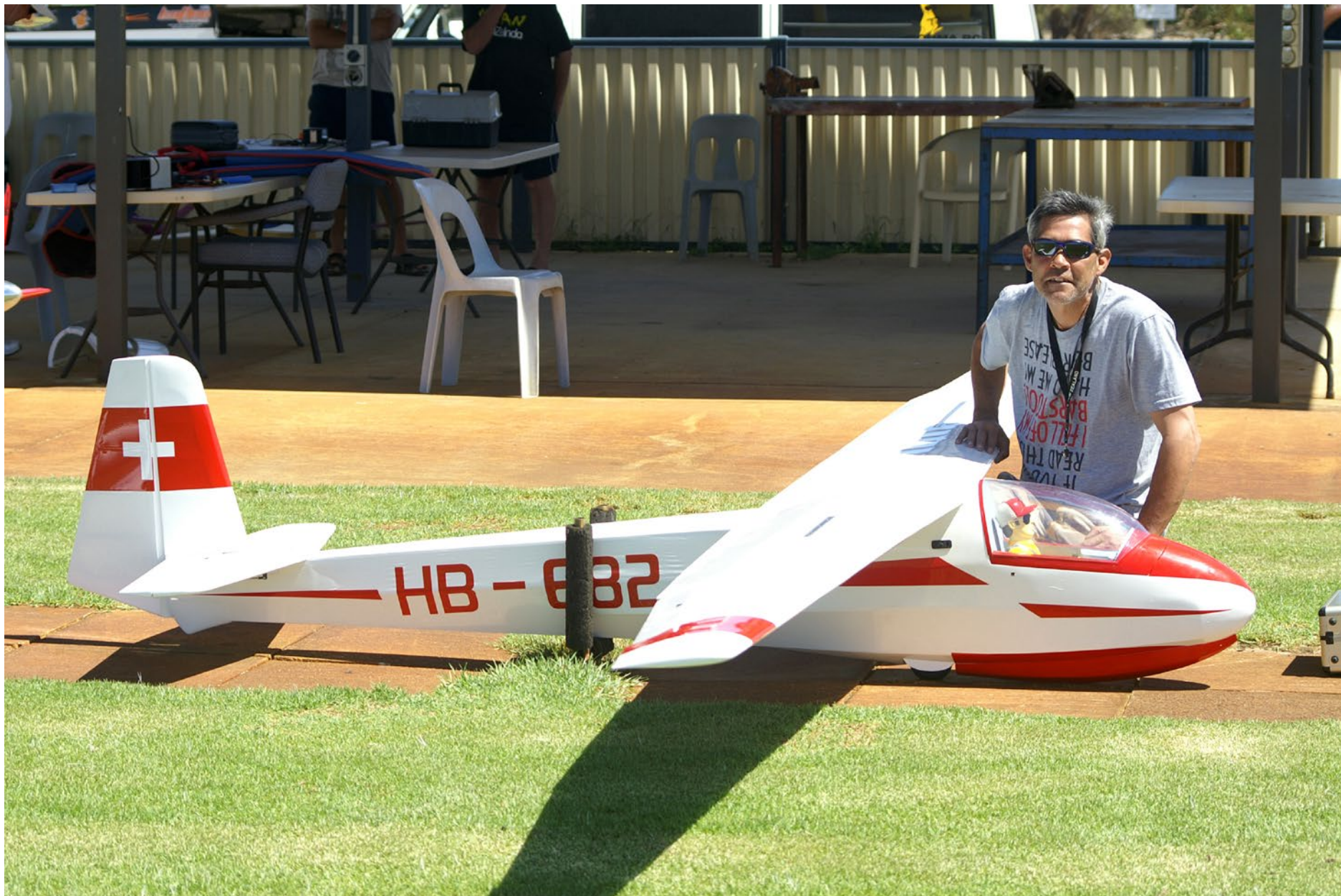
Malcolm "Kiwi" Woodbury, Phoenix Models Ka8b Wingspan: 6000mm (236.2 in) - Length: 2873mm (113.1 in) - Wing type: HQ airfoils JR 10x radio system with 8 Hitec servos. Unfortunately, a programming issue grounded the Ka8 and the model did not fly
