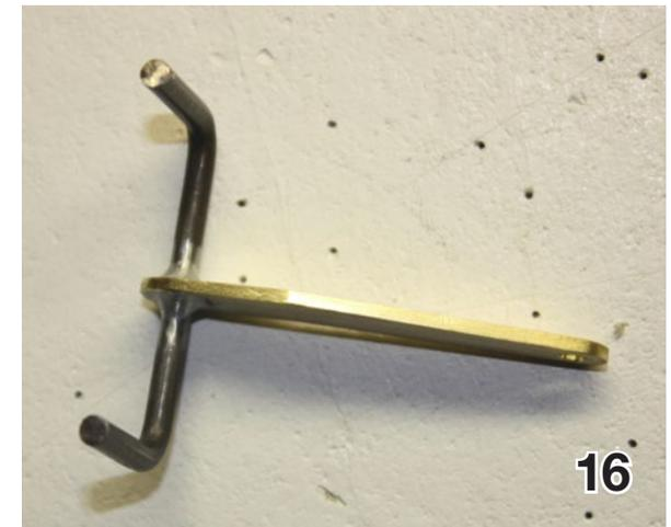
The elevator leading edge piece must also be notched to allow the control horn assembly to fit flush with the aft surface of the leading edge. I used a razor blade, X-Acto, and small file to do this. It might have been easier to make this notch before I glued on all the elevator ribs! Check the fit of the control horn assembly and block and glue into place with 15 minute epoxy. See pix 17-21.
