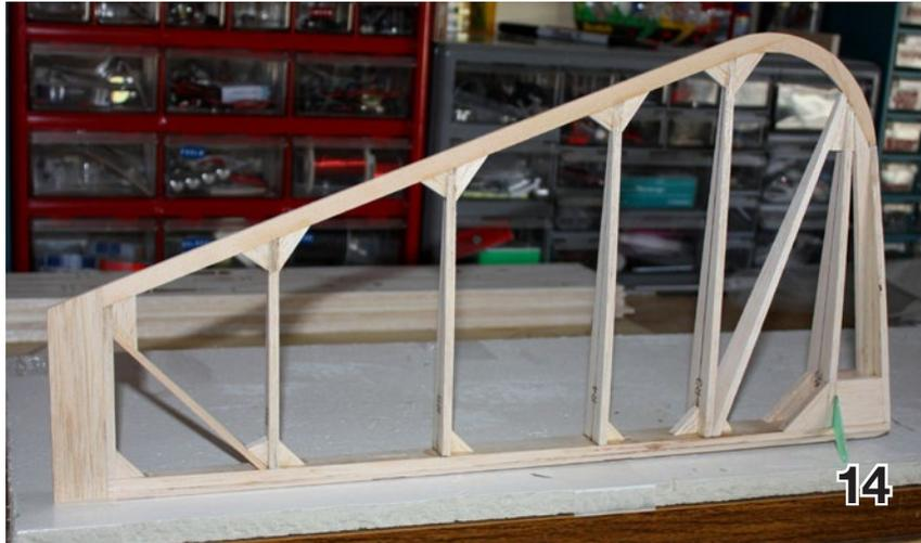
Draw a centerline on the LE, mark the locations of the hinge slots, and cut the slots.
