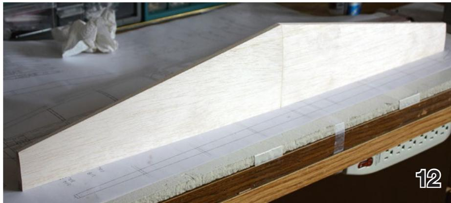
This completes the basic construction of the horizontal stab. The elevator is next.
