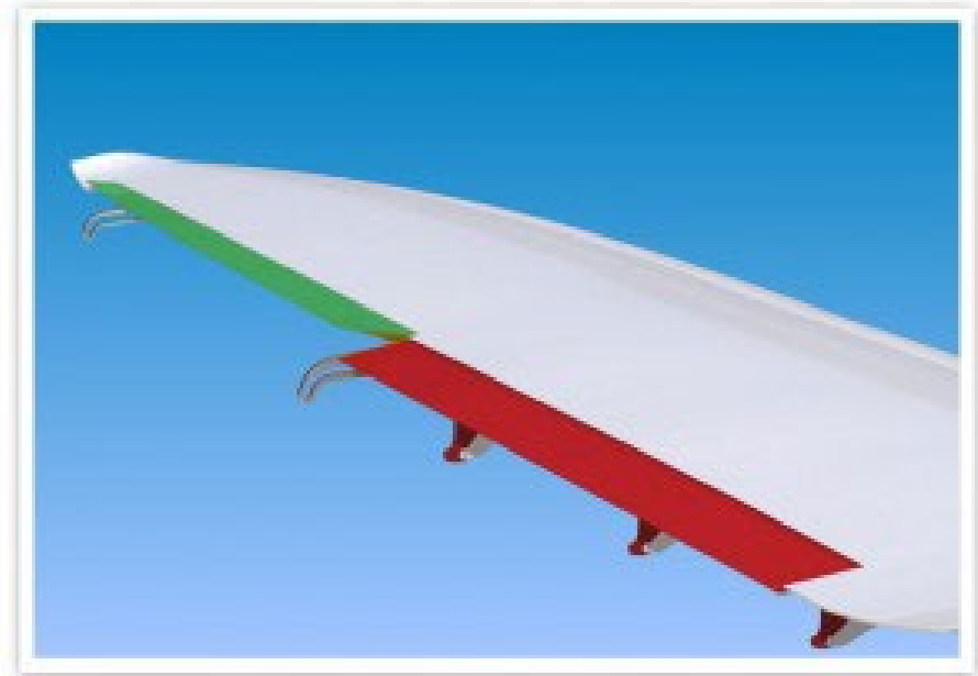
Left wing – upper aileron panel (green) and lower auxiliary flap (yellow) panels comprising the Lam Aileron deflected upward together as a unit for a left turn at cruise with the conventional main flap (red) in its stowed or neutral position on the left wing.
