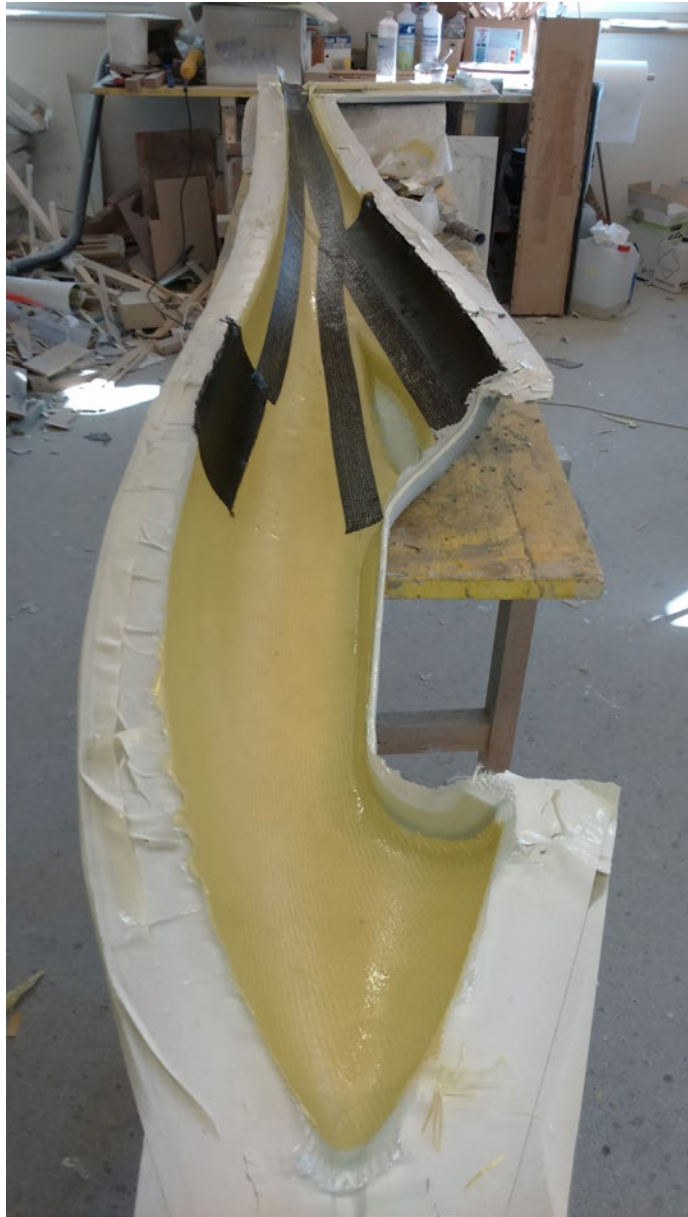
Lay-up of Kevlar with carbon fiber reinforcements in place.
