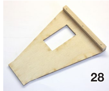
26 - 31. Removable tow hook servo mount. A thin coat of 5 minute epoxy helps Velcro stick better. The 1/4" sq. basswood rail is drilled for 4-40 and attached with CA and #2 screws. Hitec HS-485HB servo is installed. Views of tow hook servo mount installed into the fuselage.
