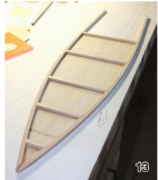
13. Another view of the installed longerons and cross pieces on the bottom of the cockpit floor.
