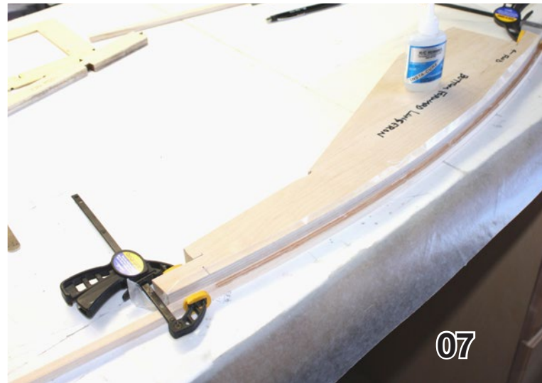
07. Longeron and 1/64" ply pieces clamped to form and glued with CA.
