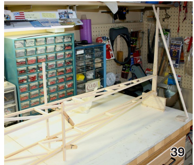
38. Fin post brace to maintain alignment. You can't see it here but there is a centerline drawn down the fin post that is used for alignment.
