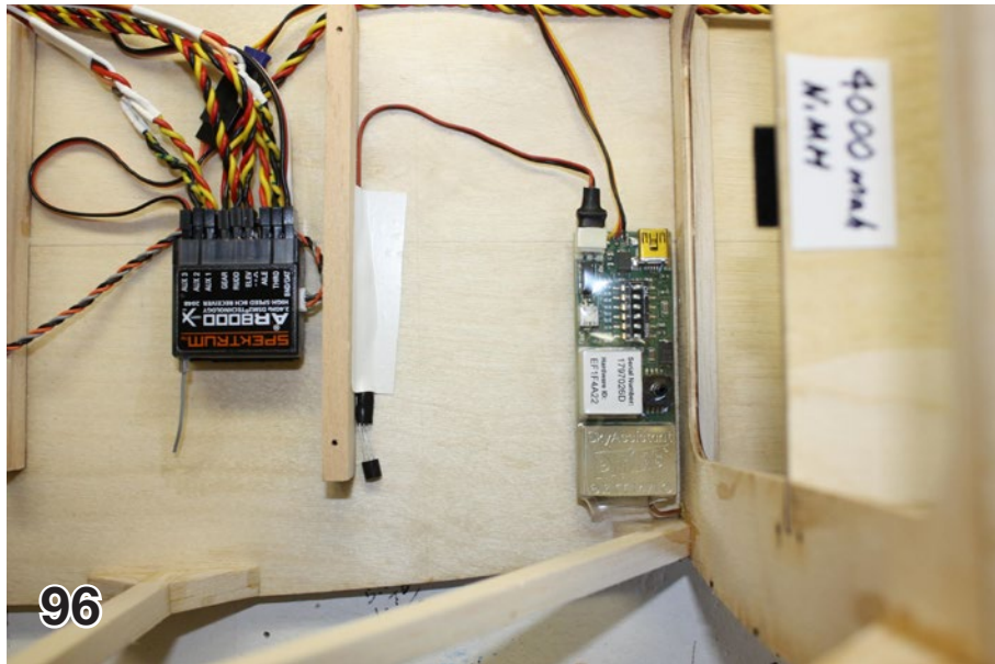
96. Sky Assistant vario/telemetry unit mounted against aft side of former F3.
