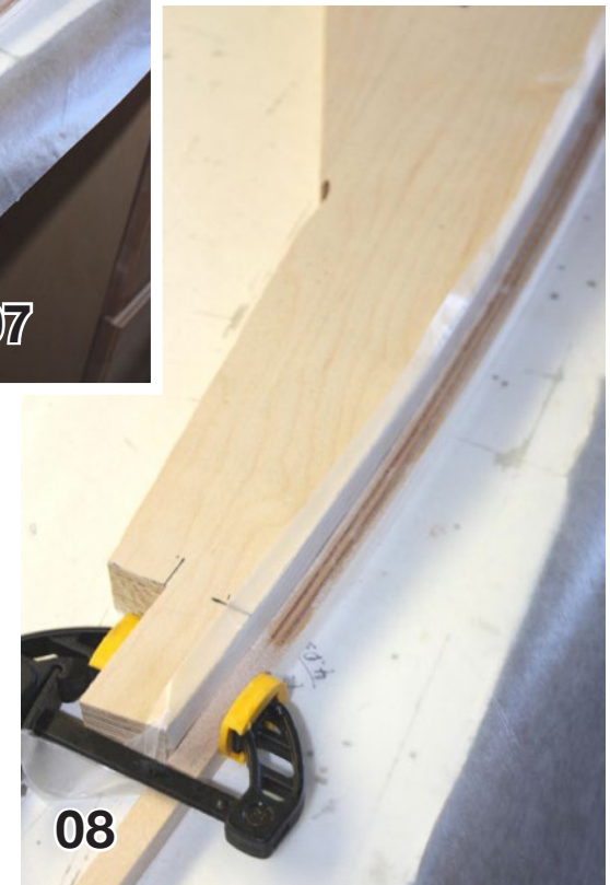
08. A closer view of the glued longeron laminations.
