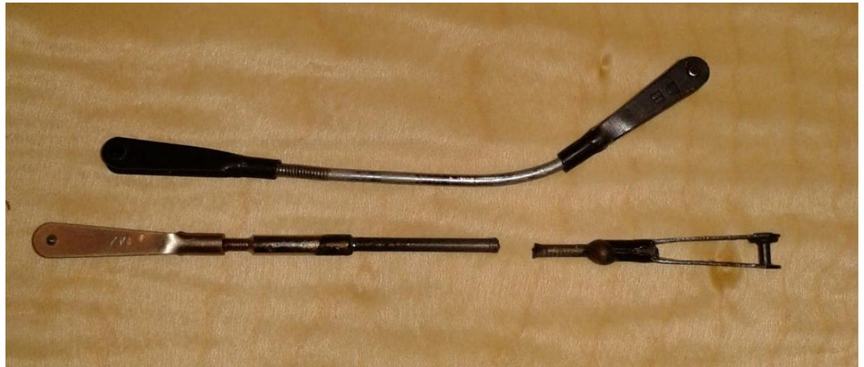
*Bent and broken clevis rods.*
