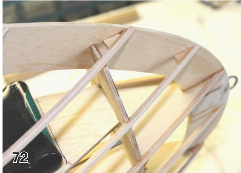
Use the plan templates to cut the 1/2" balsa contour blocks, and the 1/8" thick X 1/8" wide ply pieces that go underneath the contour blocks (to reinforce the thin edge after sanding). Sand the aft ends of the contour blocks to match the angle of F3A and CA the blocks into place.
