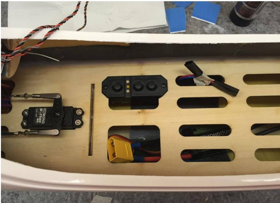
*Upper left: I made a small shelf for the receiver mostly to get it above the carbon strengthening that is around the middle of the fuselage.*
