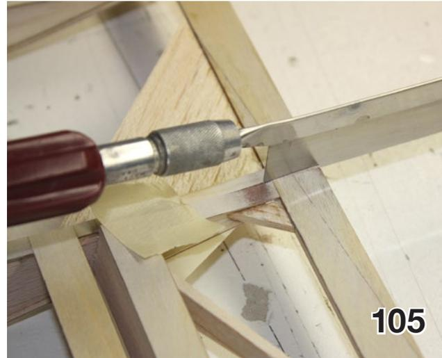
Use a razor saw to cut through the remainder of each rib from the bottom side. See pic 104.
