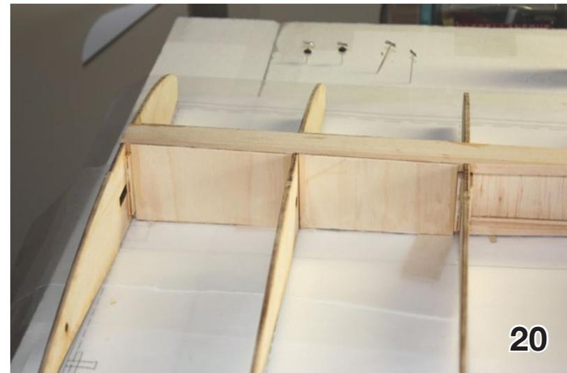
18. Right wing with upper spar cap glued into place.
