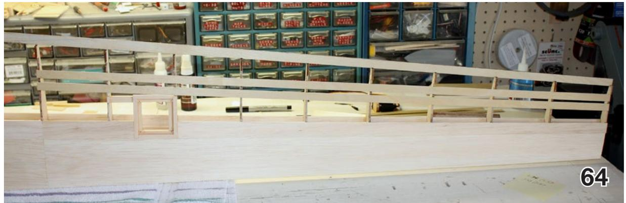
62. The aileron hinge line is drawn on top of ribs 12 - 21 with a fine Sharpie and long straightedge.
