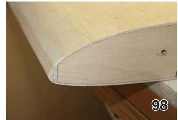
Also look at the gap and sand the root end of the wing and/or the fuselage center section to get a decent fit. You might even find it necessary to add some pieces of thin plywood and sand them down to get a nice fit. See pic 101.
