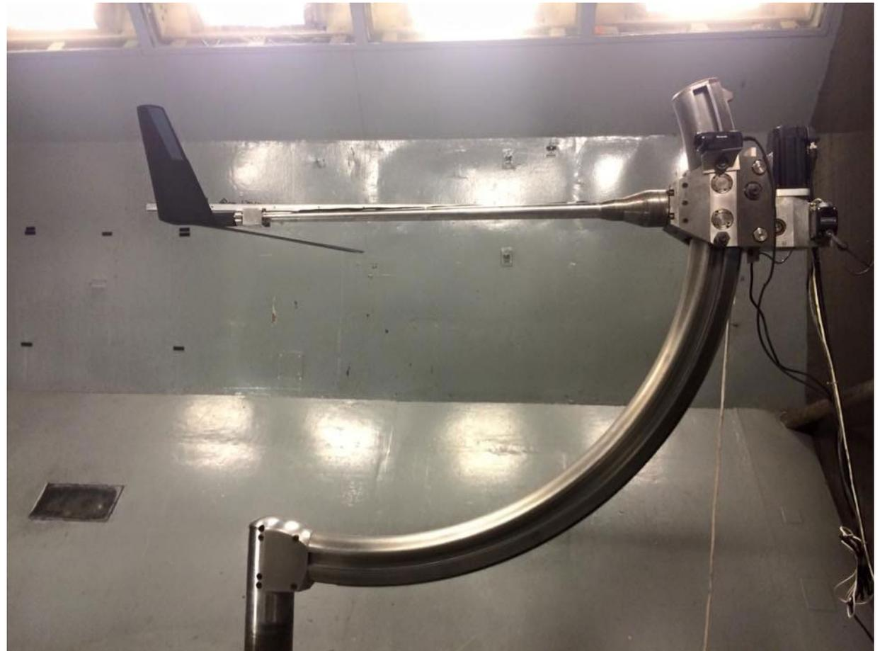
A PRANDTL 'wing with semicircular tip elevons in the NASA Langley 12 foot wind tunnel.
