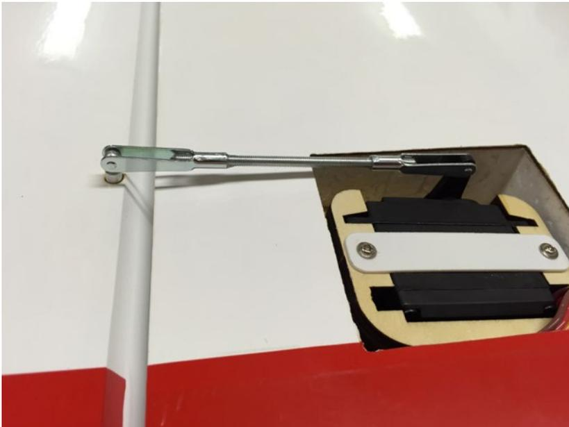
*Staufenbiel wants you to use Z-bends with the included linkage but I found some of them to be too brittle and besides I like my links to be solid above certain sizes. So I replaced the included rods for 3mm threaded rods with clevis on both ends adding a carbon tube over the elevator linkage due to its length.*
