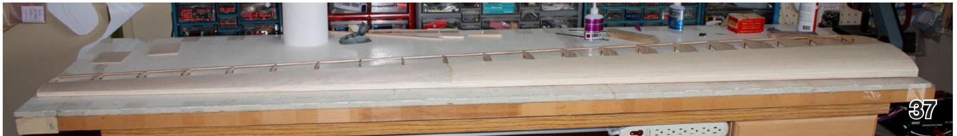
Before gluing the top D-tube sheeting, the entire wing needs to be pinned down.
