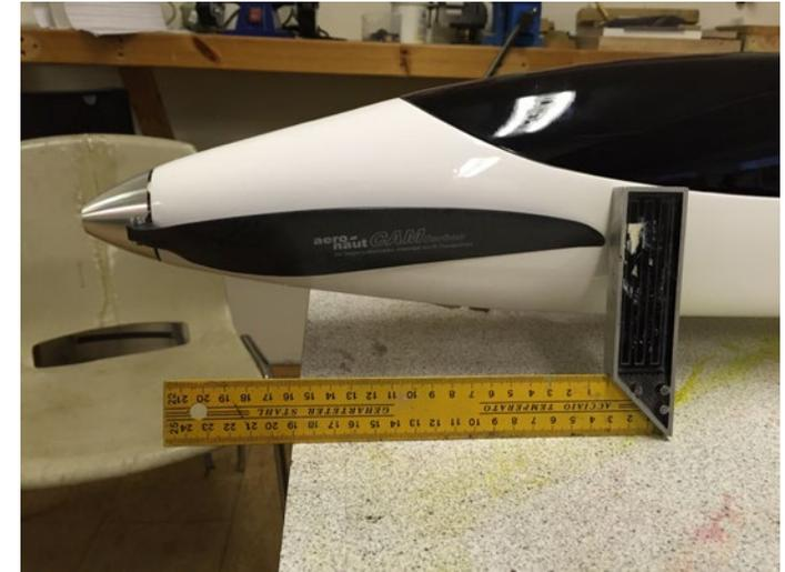
*Left: The first kits were supplied with a Aeronaut Cam prop that isn't up to the RPM's and were replaced by Staufenbiel's own product.*
