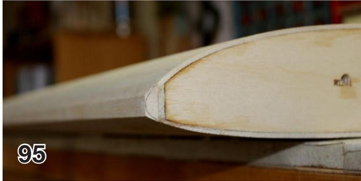
CA a small piece of scrap 5/16" square balsa onto rib 1 at the bottom of the connector hole, and then CA the connector shell into rib 1 so it is flush with the root side of the rib. See pix 92 - 94.
