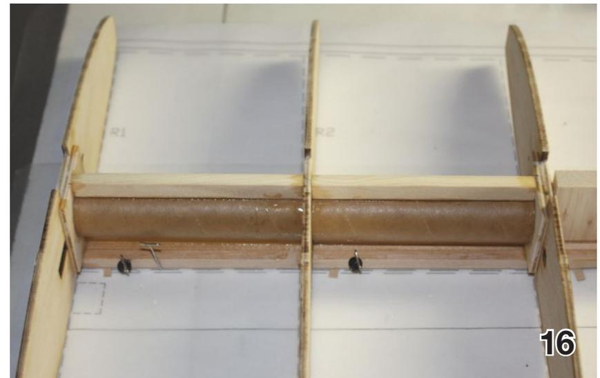
Cut the wing socket tube to length and glue in place with 15 minute epoxy. It should be glued to ribs 1, 2, and 3, and to the top edge of the 1/4 wide spruce pieces. See pic 15.
