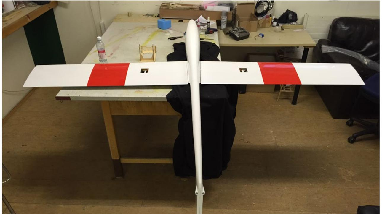
*The wing comes in four parts, divided at the aileron/flaps and flaps/fuselage. The flaps could have a nice career as barn doors!*
