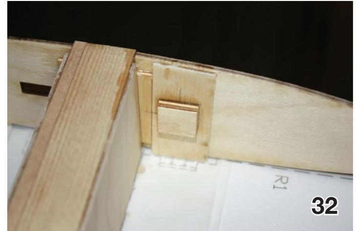
32. The 1/16" plywood cap glued onto the 1/8" plywood doublers.
