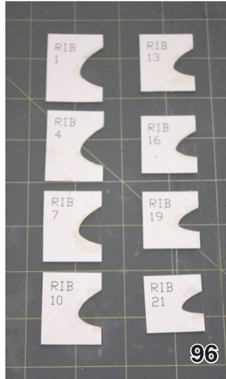
Use a razor plane and sanding blocks to shape the leading edge, checking often with the sanding templates as you progress. See pix 97-98.
