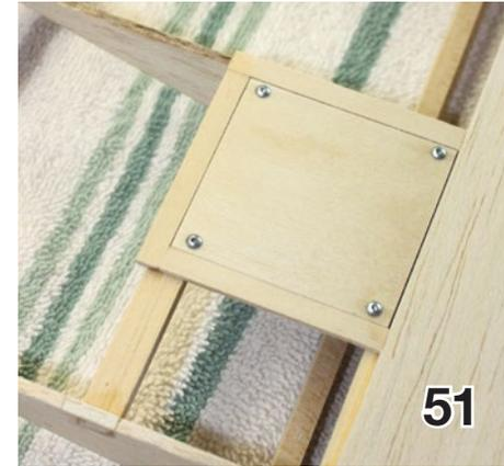
Cut and fit 3/32" plywood doors for the spoiler and aileron servo mounting frames.
