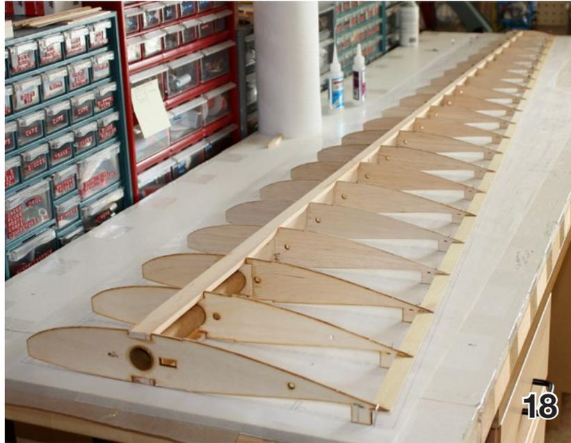
Fit check the upper spar cap again and sand the top of any webs if needed.
