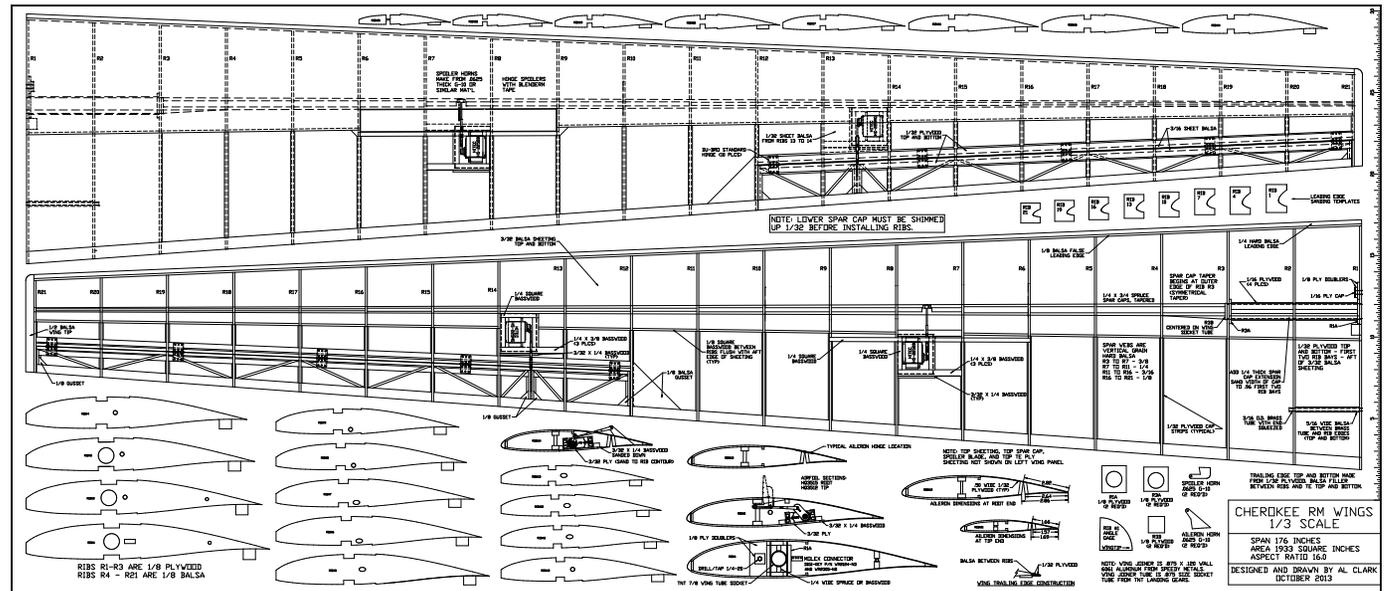
Trim the length of the joined spar caps to about 1/8" longer than required; the excess will be trimmed off at the tip when construction is almost done.
