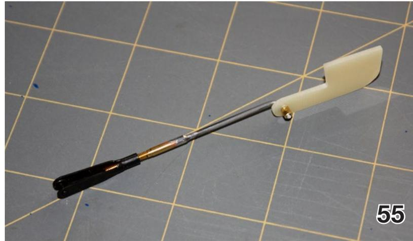
Copy the spoiler and aileron horn shapes off the plan and glue the templates to the G-10 with rubber cement. Cut the horns out a bit oversize and sand to final shape.
