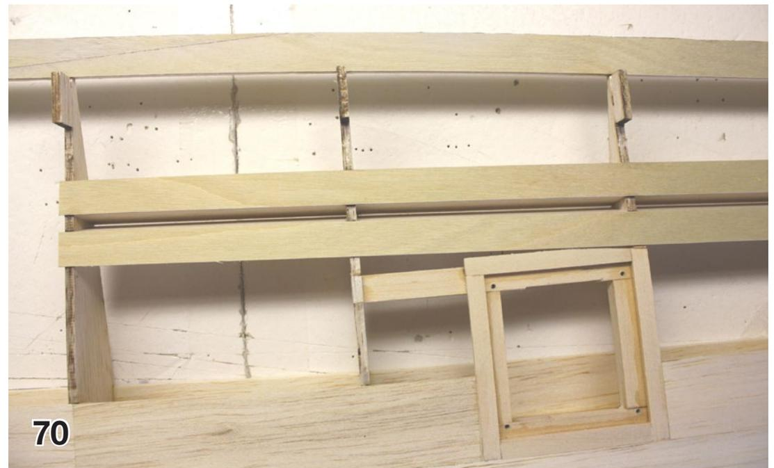
67. Aft (aileron face) webs being glued into place. machinist ruller used to get 1/64" spacing from front webs.
