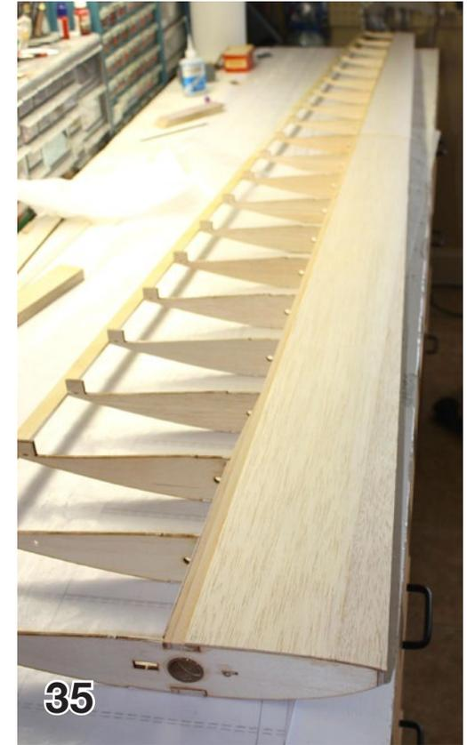
marks, and CA the entire edge of the sheet to the spar cap.
