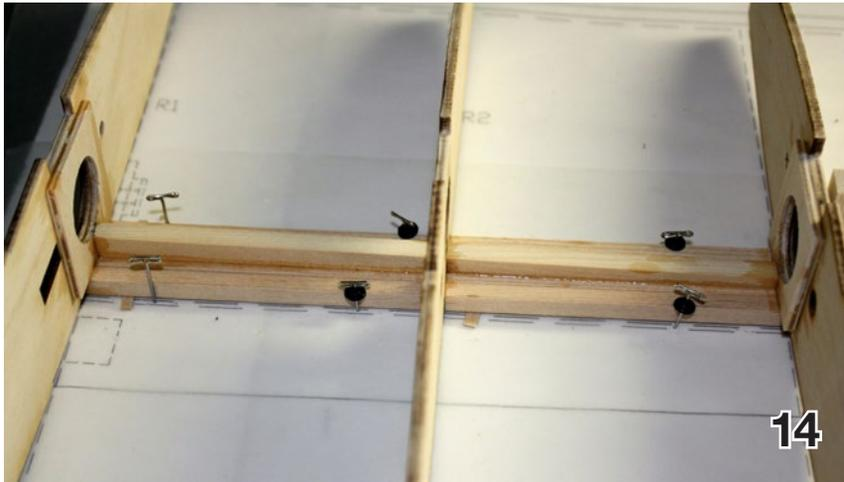
Sight down the trailing edge and adjust its position at rib #11 so it is straight. Go back and double check the position at rib #1 and rib #21 and CA the trailing edge at ribs #1 and #21.
