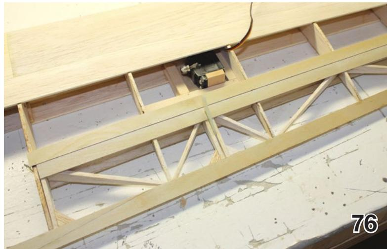
75 and 76. These photos show the aileron diagonals in place. Unfortunately, the 1/32" plywood pieces were already in place when the photos were shot. The hinge slots (See pix 79 and 80.) were also created before the 1/32" plywood pieces were glued on.
