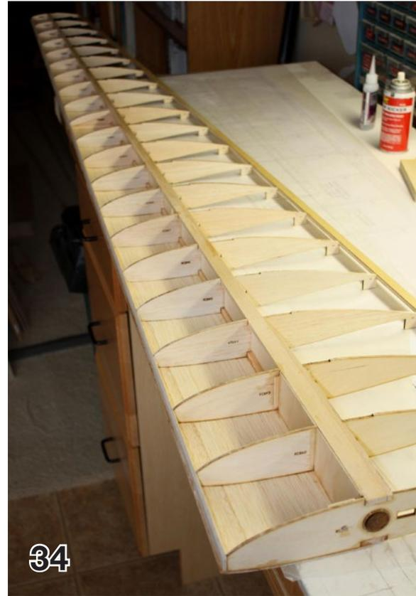
D-tube sheeting to fit. The inboard piece will need some additional 3/32" sheet added to make it wide enough. Leave 1/8" extra on the root end, leading edge, and tip end.
