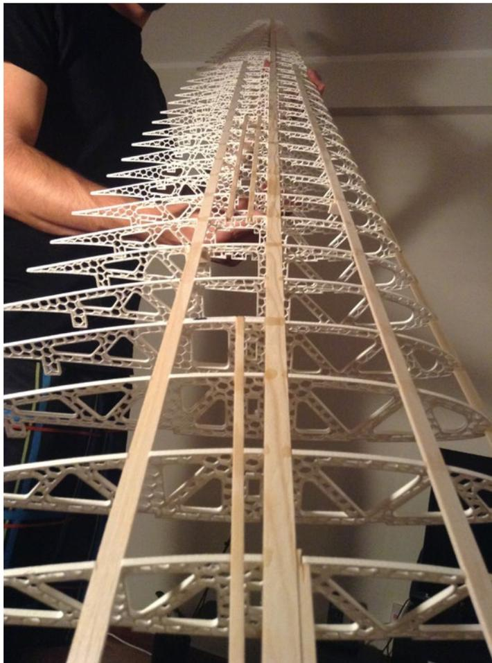
Being the owner of a 3-D printer for quite a while, I have been doing a lot of small things like servo trays, dummy engines, pilot heads (photo below), bits and pieces. But this time I decided to use the printer on a large scale, so I've been printing ribs and frames for the Jilles Smits' 4.7m KA6E (photo at left).
