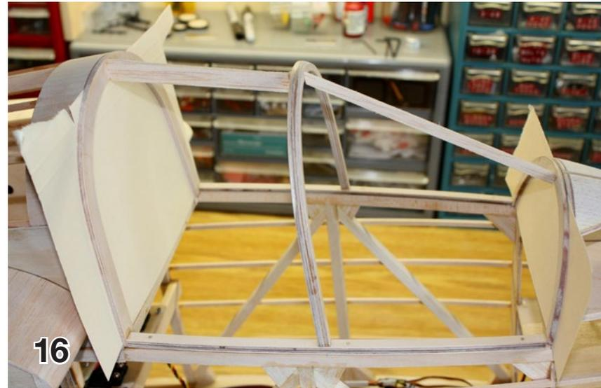
Again using the taped sanding block, bevel the aft half of C2, bevel C3, and bevel C1.
