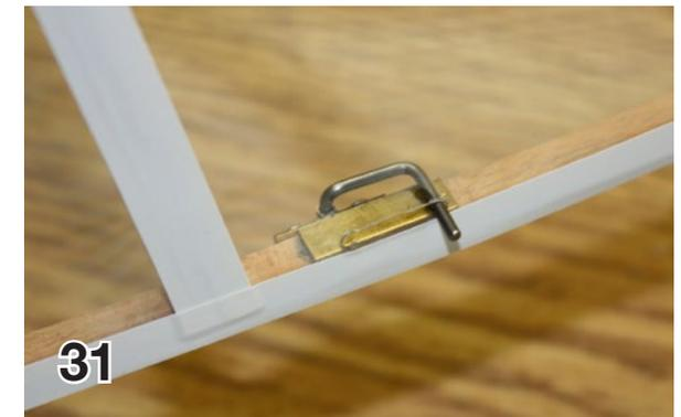
30 - 32: The latches are mounted on the canopy side rail with cut off #2 sheet metal screws. These photos show the right side latch in the open position.
