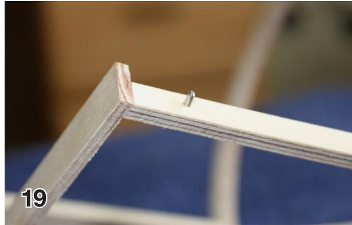
Make six pins, each 5/16" inch long, from 1/16" dia. music wire. One end of each pin should be rounded off nicely. Use a small hammer and tap the pins into the canopy side rails so they are flush with the top – later the pins can be CA'd into place. See pix 18 - 19.
