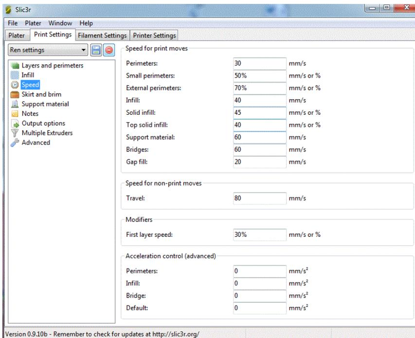
The slicer parameters that I am using are shown in the three screen grabs on this page.
