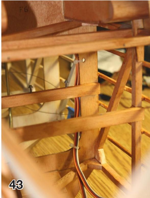
The wiring harnesses coming from the wing roots need to be tied down with two tie-wraps which use the holes provided in former F6. See pic 43.
