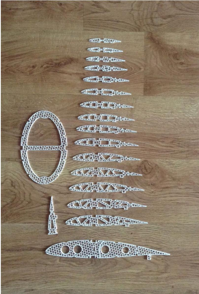
The printing time is quite high, around 30 minutes for a 29 cm rib, but this is mainly because the printer nozzle diameter is 0.35mm, which is good for detailed objects but not necessary for this particular job. The nozzle could be changed and that would reduce the printing time in half.
