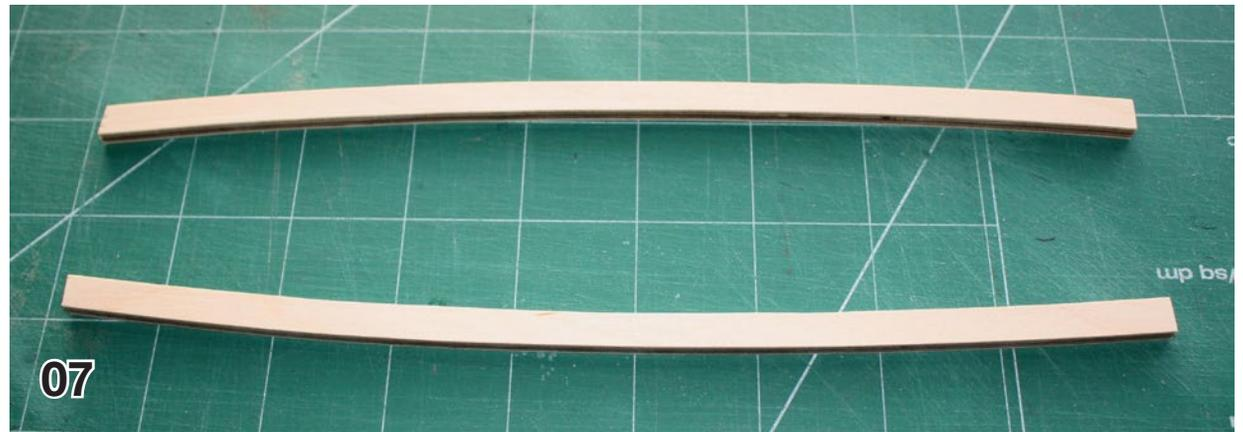
Laminate the two C2 formers together with CA+ or 5 minute epoxy. Pic 8 shows C1, one of the C2 formers, and C3.
