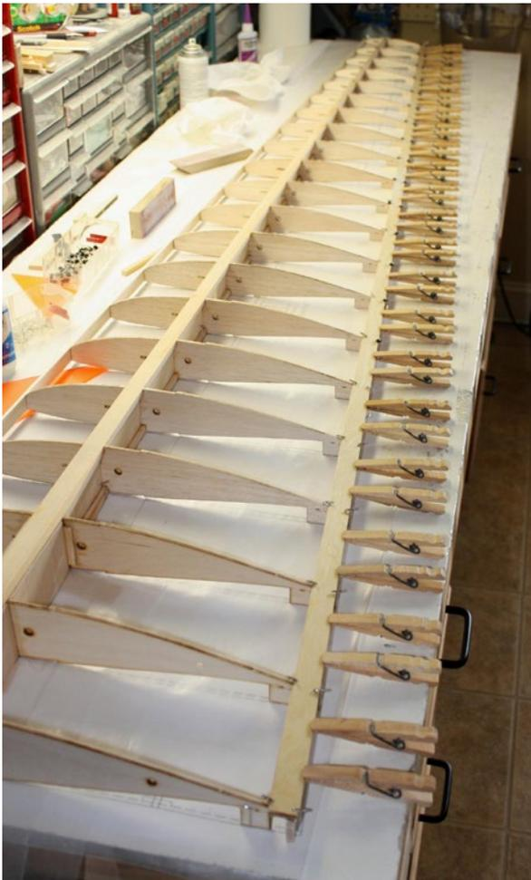
Those of you who have been following Al Clark's 1:3 scale Cherokee RM build may have noticed his use of a number of modified clothes pins to help hold the wing trailing edge as the glue cured. Al used 40 of these clamps during the construction of the right wing.
