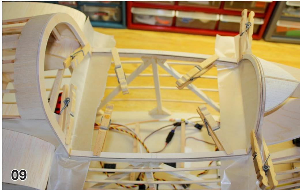
Make up a spacer from scrap balsa to maintain the proper distance between C3 and C2 at the top and tack glue it into place.
