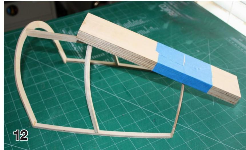
Now the edges of the canopy formers need to be sanded/beveled so they will contact the inside of the plastic that will cover the canopy frame.
