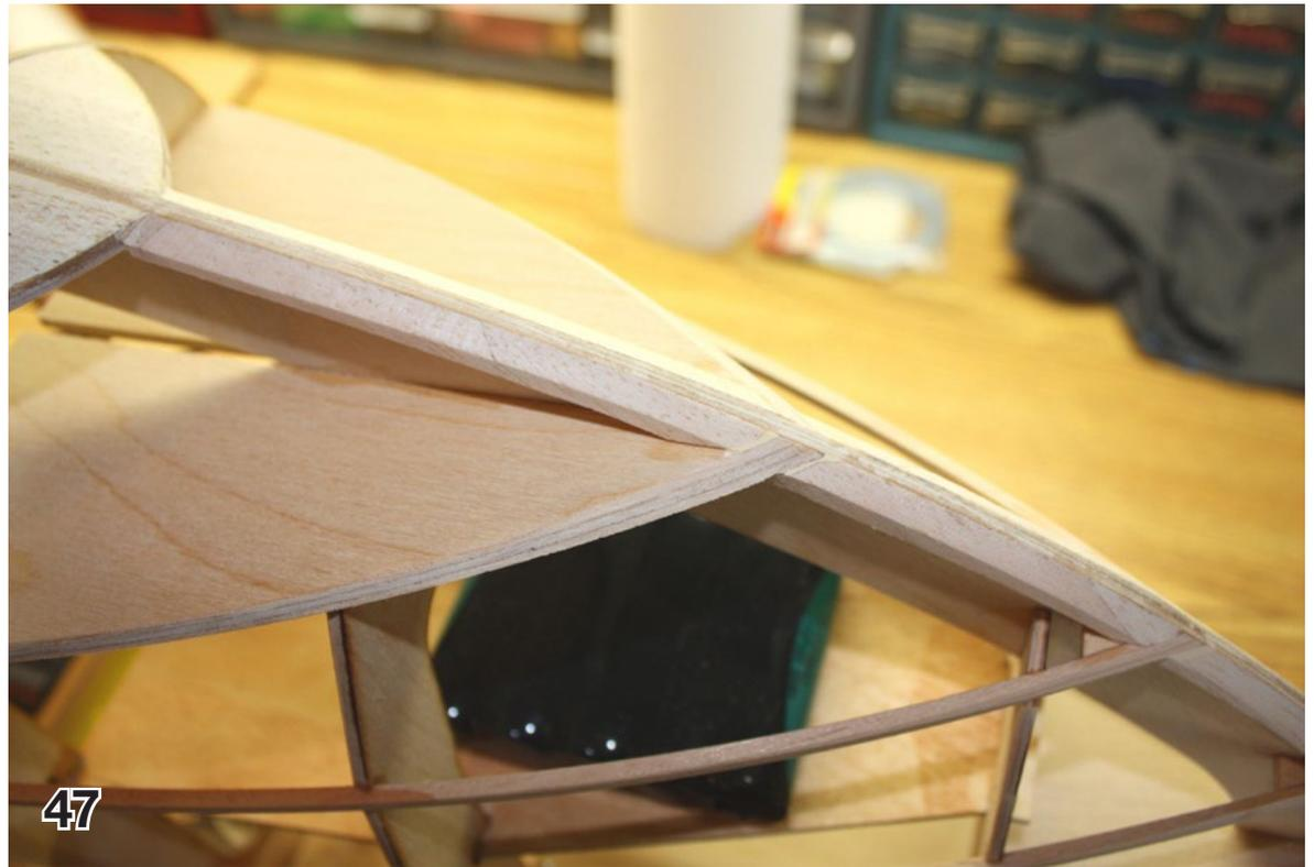
The upper keel is only 1/8" wide and that is not much for the covering to grab onto, so I added some balsa on each side of the keel that has a surface 3/16" wide for additional covering grip.
