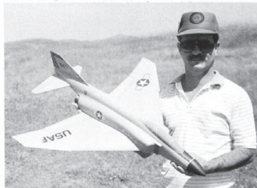
Eric Clutton offers this unique F-4 Phantom kit. Good stuff! The fuselage is vacuum-formed plastic; the wings are blue foam. The builder must furnish wood and hardware.
