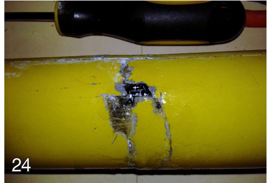
25. Ran the balloon in to the right spot and blew it up gently. Then blew hard to pop it and pulled it out. I did it again with a surgical glove since I ran out of balloons. I left it in until the epoxy got tacky and then blew till it popped and pulled it out.
