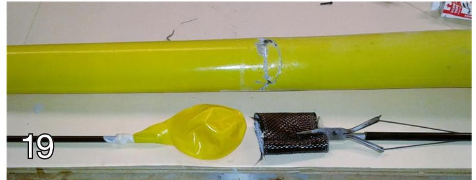
Here's how I used it to repair an Aquila XL fuselage:
