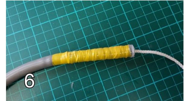
(6) Wrap the length of the wire wrap with insulation tape to cover all exposed wire wrap. Do this on all ends and the bungee rubbers have now been completed.
