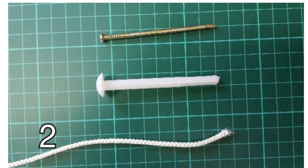
(4a) Prepare nylon anchor by sanding or Dremel the ends so they are close to the size of the outside diameter of the rubber tube.
