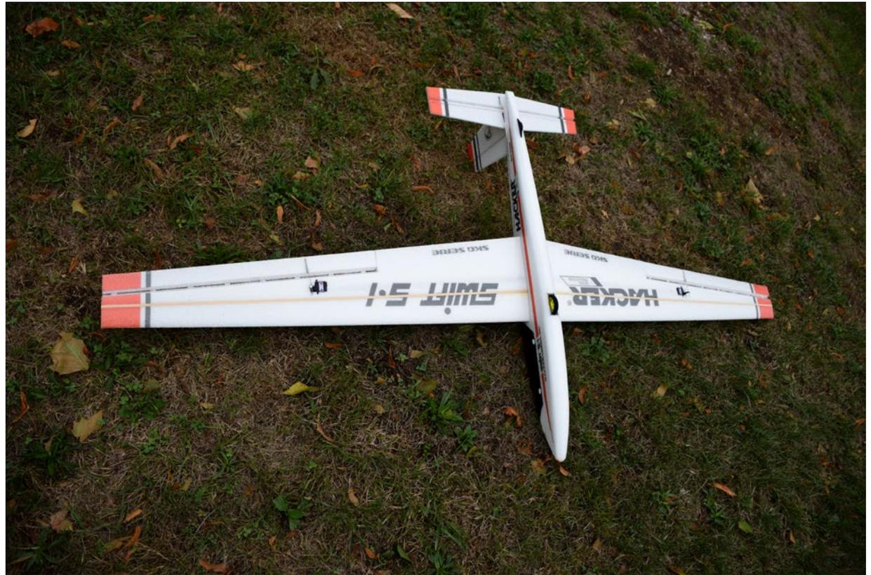
inverted flight is no problem. The vertical maneuvers like reversals, looping, suffer from lack of amplitude due to the low weight of the machine, nothing abnormal.
