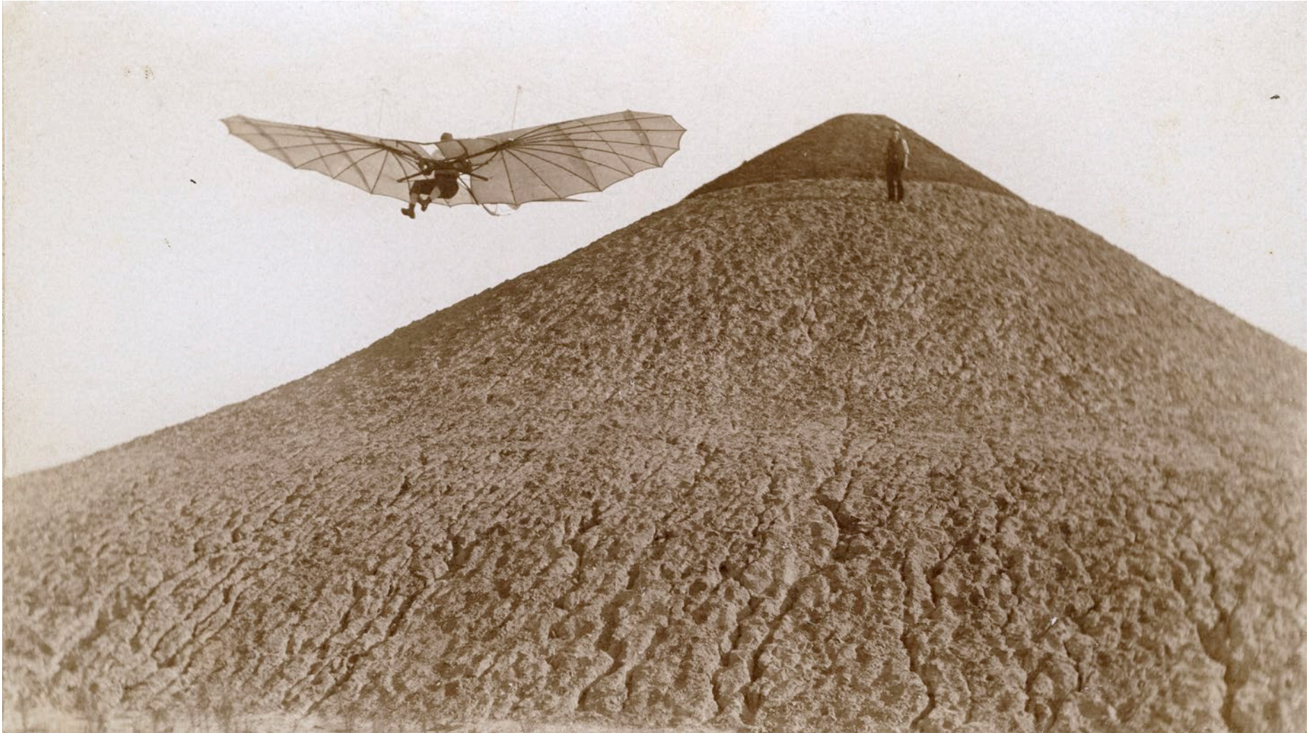
Lilienthal in flight during 1894. The image shows Otto Lilienthal flying from the Fliegeberg near Berlin. He constructed it specifically for launching gliders; it is thus one of the first artificial airfields. Ottomar Anschütz, a pioneer in photography, took the photograph. Credit: Otto-Lilienthal-Museum Anklam.
