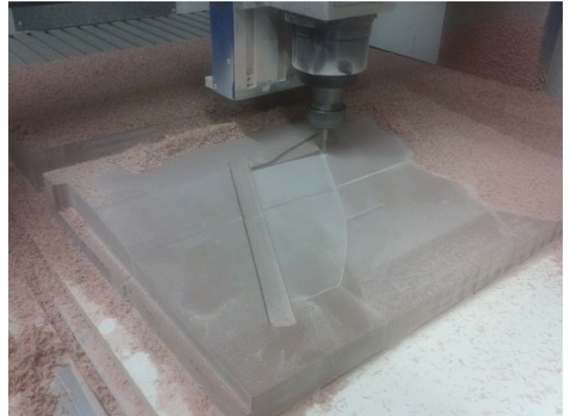
Winglet mold being milled
