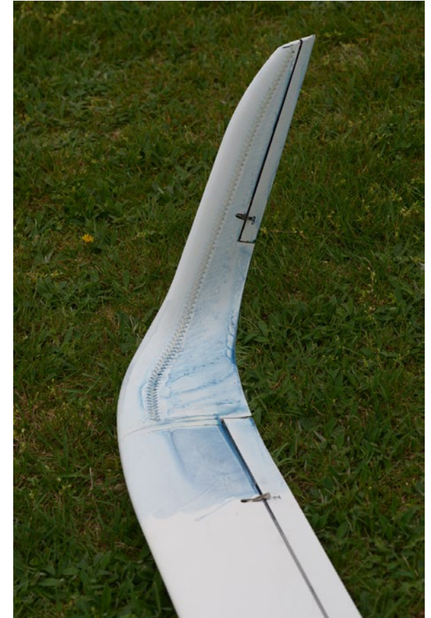
Paint is used to determine the airflow over the wing-winglet junction
