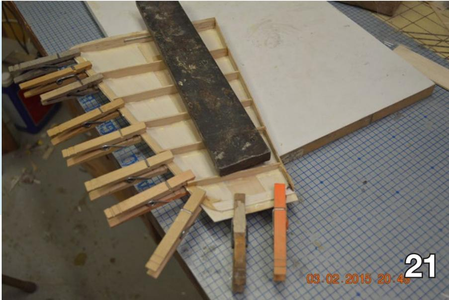
Trim the rib blanks to slightly higher than the spar and carefully sand in the fin taper on the sanding board (Photo 19). The frame is very fragile at this point so carefully sand the ribs by pulling them across the sanding board.
