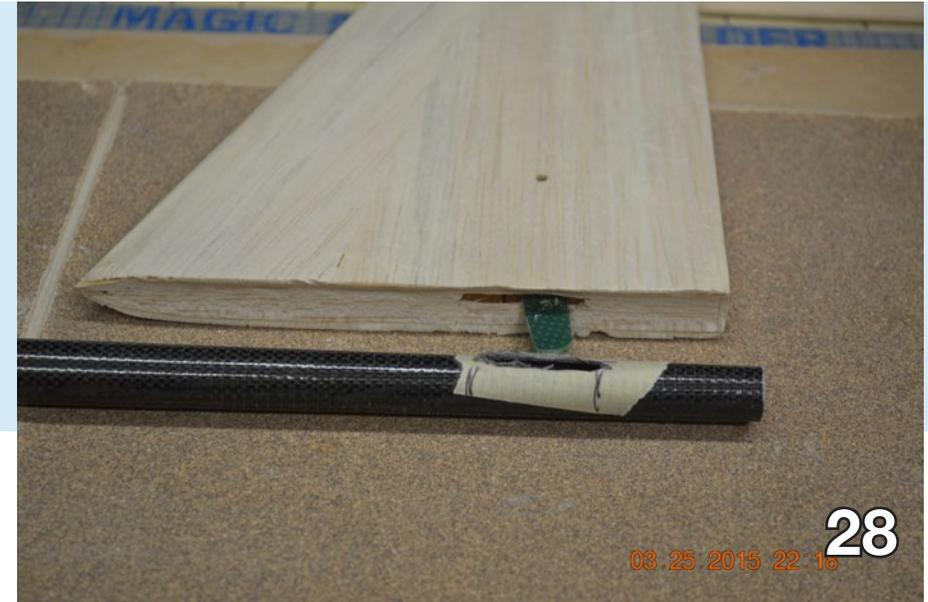
The rib blanks are beveled 60 degrees on the Miter Cut and slotted on the band saw for the trailing edge. Rib blanks are ½" wide and 4 inches long. The trailing edge is ½" wide and 12 inches long while the leading edge is ¾" wide and 12 inches long. Photo 23 shows all rudder parts ready for assembly.
