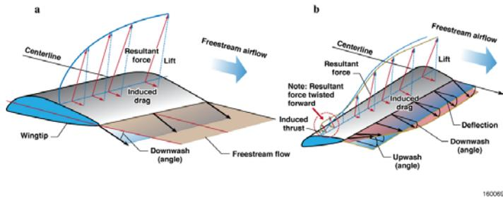
Figure 2. Prandtl's elliptical and bell spanloads explained.
