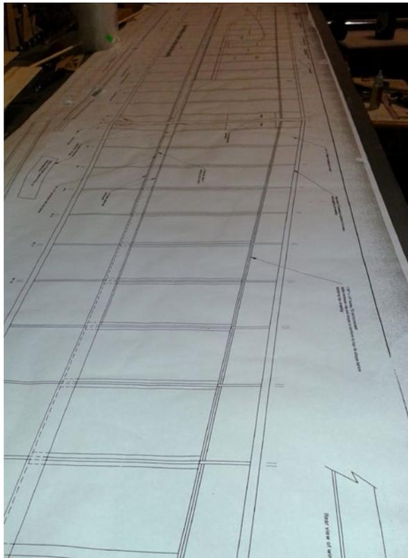
(4) Carpet Shield is good for permanent covering of plans. You can also use Duck Peel and Stick.
