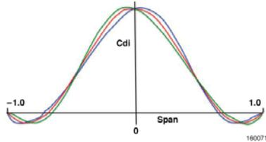
Figure 4. Effect of sideslip on bell spanload with twist (0 and +/- 5 deg).
