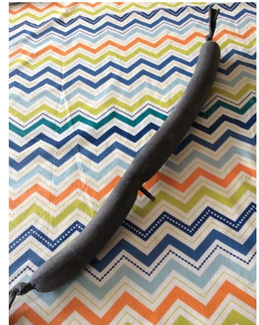
Here is a new tool I made to hold a patch inside a fuselage or similar repairs. Made from a bicycle tire tube.
