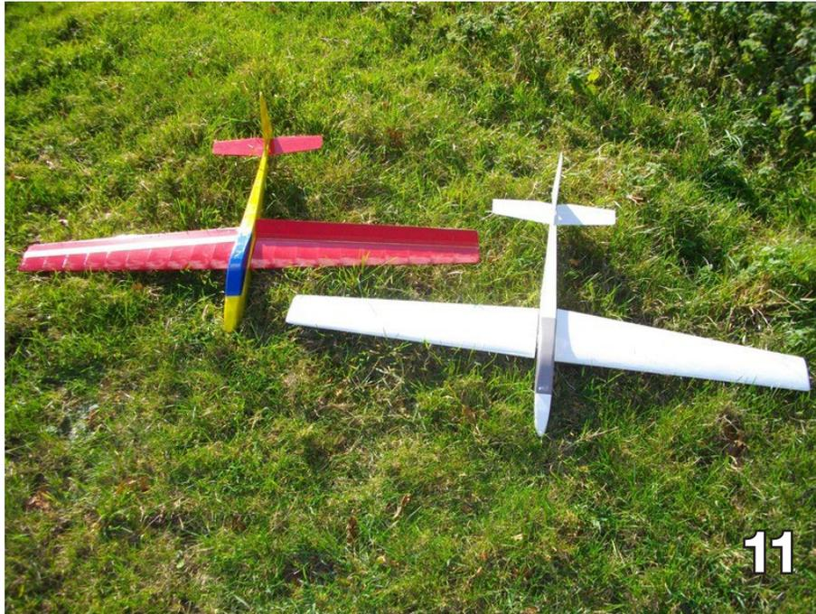
Photo 11: (L) Aileron version, (R) pivot wing version
