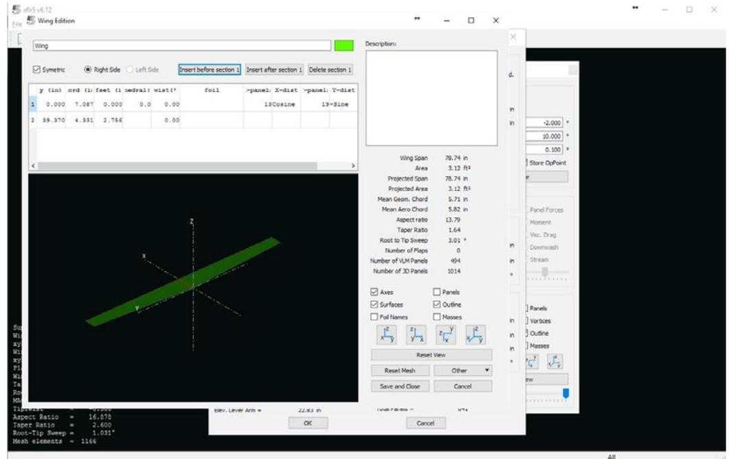
Each flight mode is set up as a different plane. I recommend doing this so you can compare polars across flight modes.
