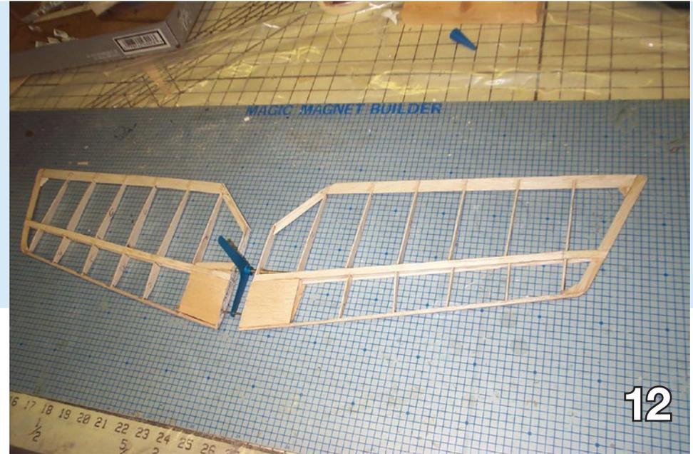
When satisfied with the alignment, epoxy the other stab pivot wire tube and the forward stab wire in place.
