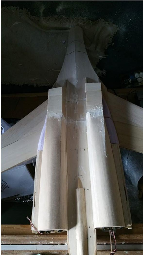
14. (Left) The build progresses nicely - lots of filler splattered here and there, a few filling blocks of pink foam squeezed in, and the sanding has started in earnest. It's all going quite well at the moment, so may even see some glass fibre applied before the year is out, which will be nice. It's all going quite well at the moment, so may even see some glass fibre applied before the year is out, which will be nice.
