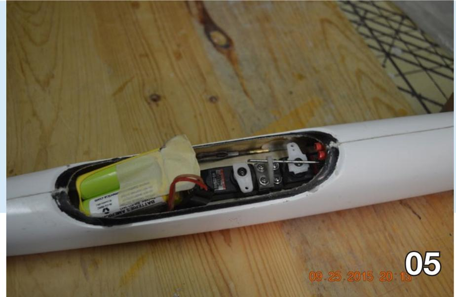
Splicing a female servo connector in the negative power lead let me use a shorting plug in the socket to connect the battery. I also use the center pin in the socket to charge the battery through an adapter made by splicing two servo leads salvaged from deceased servos to connect the charger. See the wiring diagram at right and Photo 6.
