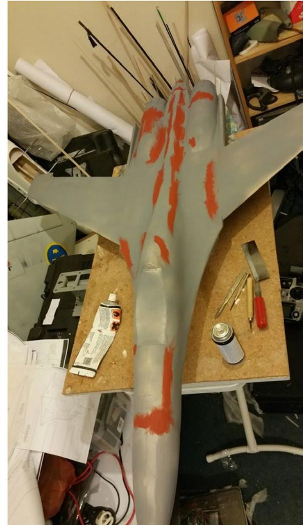
29. I then reinforced the underside of the hatch with some 1/64th" ply, added some mounting blocks inside the fus, then re-attached the hatch with servo screws. I rolled her back over, and went at it with a strong light and the red stopper / glazing putty.
