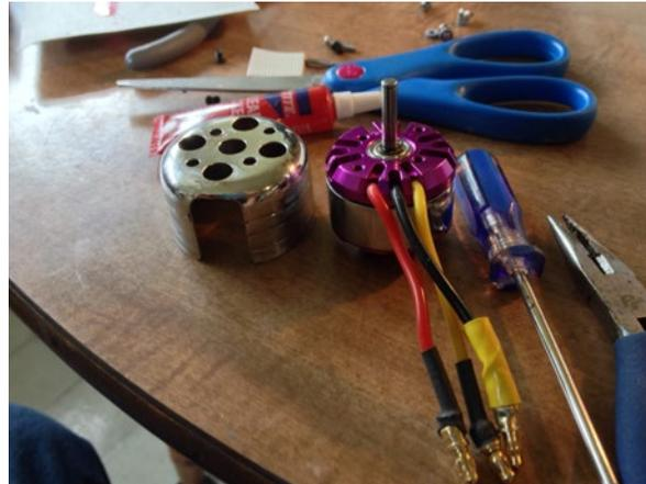
8: Milled cap & motor. I salvaged this motor from a 3D plane I shouldn't have got at an RC swap meet which came with a bad speed controller. The groove at the end of the shaft shows its shaft had been reversed.
