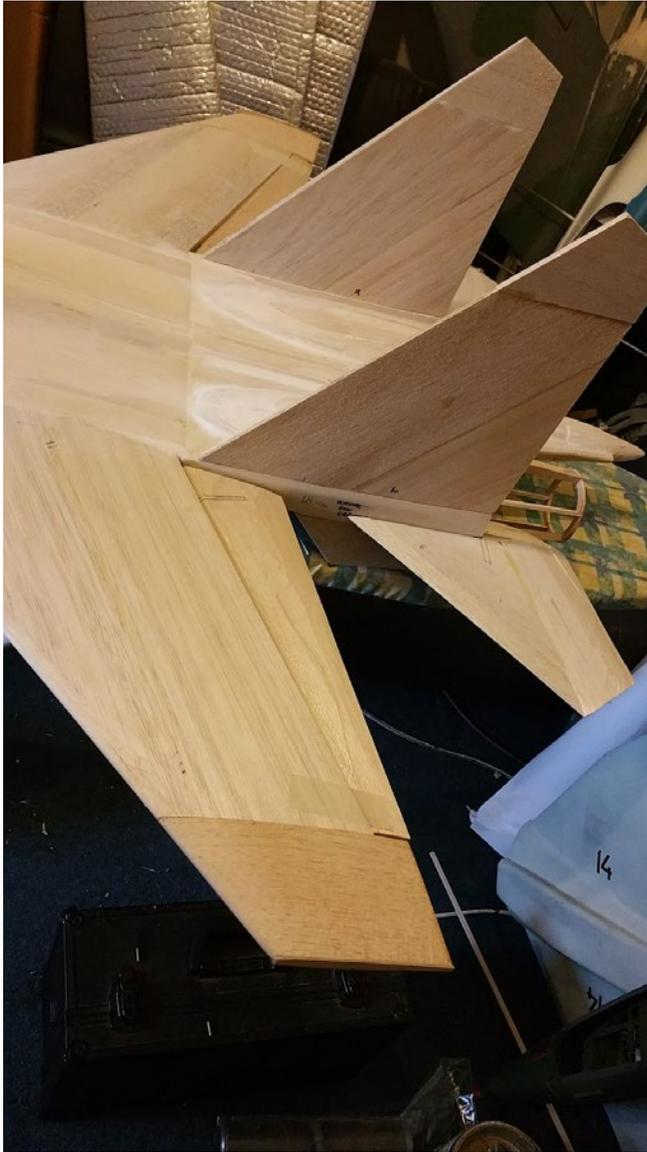
24. The wing tips have had the 1/16th inch ply end plates added to stiffen things up, and also hold the removable missile rails.
