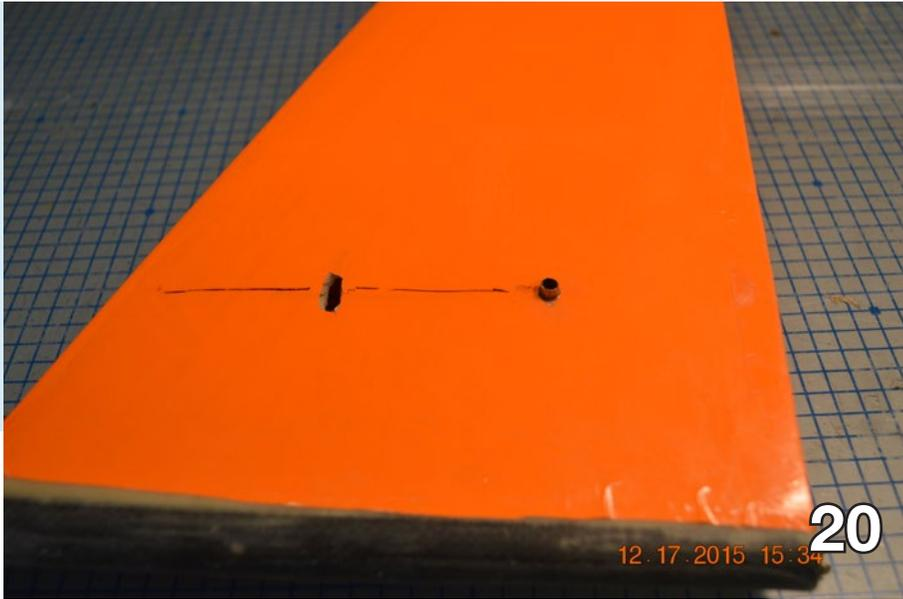
The stab pivot bearing is 5/32 inch brass tubing and should extend about 1/16 inch outside the fin to provide a gluing surface (Photo 20). Add a 1/8 inch soft balsa rib to the stab root with a 5/32 hole for the stab bearing and sand to match the fin contour.
