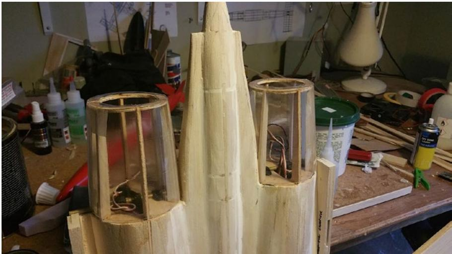
17. (Top above) The nose section I was quite worried about - it needed packing to obtain the correct angle but I still wasn't all that sure until the epoxy set. Anyway, I am happy with the way it turned out, and so I filled the joint with car body filler. I have a bit more to do there to blend it, but it's coming along.
