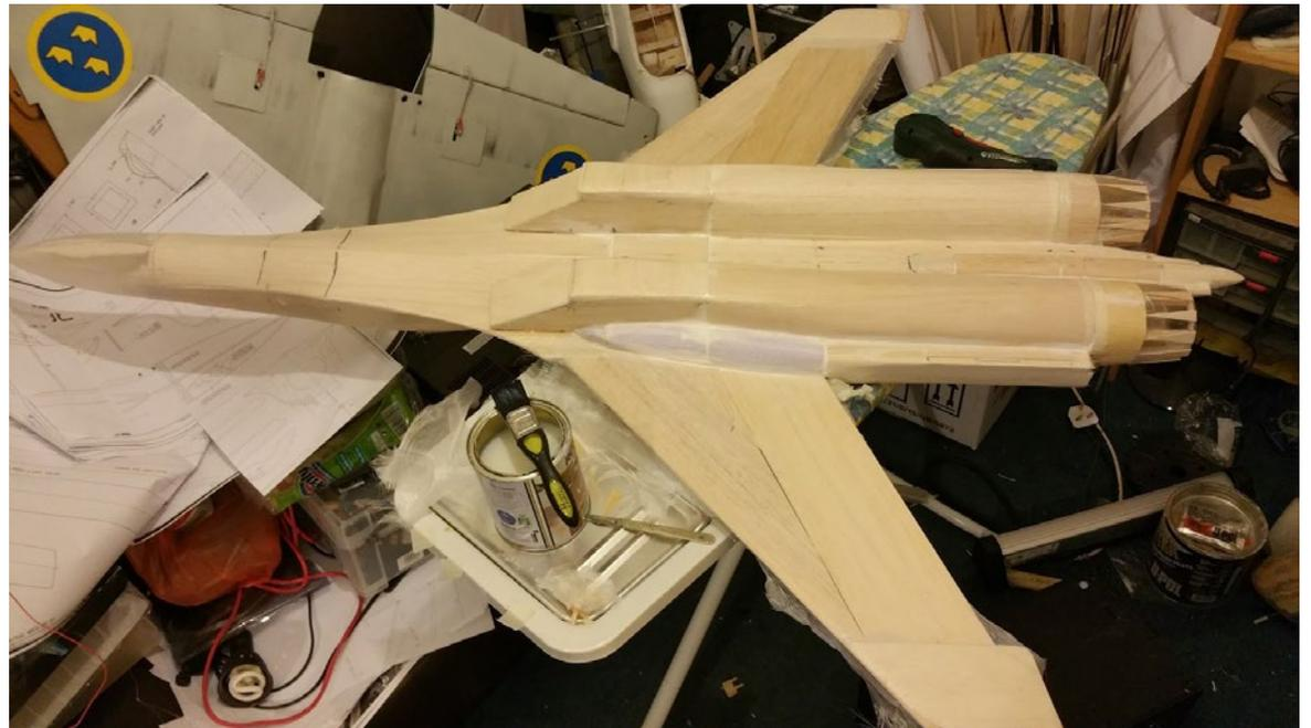
26. Well, it's hard to see here, but that's the underside of the airframe all glassed. I'm using Ronseal diamond-hard WBPC varnish, and some fairly light (no idea on weight) cloth. I really like glassing - it's so quick!
