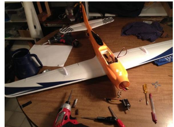
4. Destination: A Durafly EFX Racer I picked up at a swap meet. Durafly models have a hard skin over their foam, a step up from packing tape for strength and smoothness.
