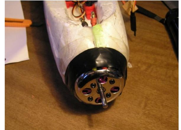
9: Martini cap and motor installed in EasyGlider Electric.
