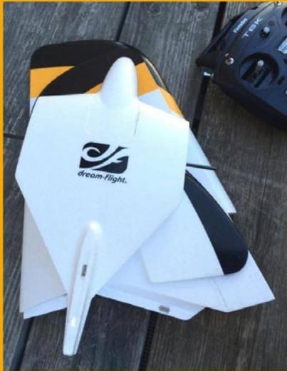
Modular Design - a clever interlocking design allows for easy transport to any location. Replacement parts are available to service your Weasel-TREK.
