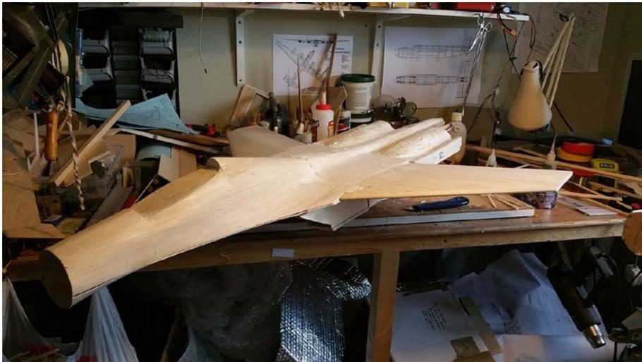
12. The Flanker now has top and bottom planking complete, the only extras needed are the..bulging..cheek...things under the roots of the wings. These will be carved from pink foam.
