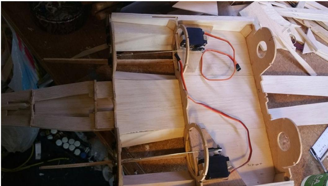
6. Here is a picture of the separate all-flying-tail servos installed in the underside of the tail section of the Su27.
