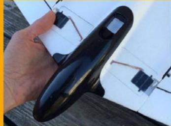
A rugged factory-installed ABS belly skid is ready for those rougher touchdowns.
