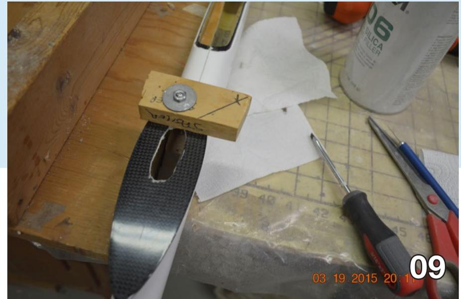
nut to clamp the T-nut to the pylon until the epoxy cures.
