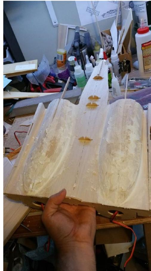
8. Some shaping has started on the engine tops now too. Heavy duty carving, then splattered with lightweight filler, as usual.
