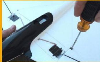
With a quick turn of the screwdriver, the Weasel-TREK's wings can be secured or removed in seconds.
