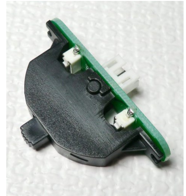
The Taranis trim switch assembly. Swapping out the internal mechanism for a good one is not difficult and takes only a few minutes.
