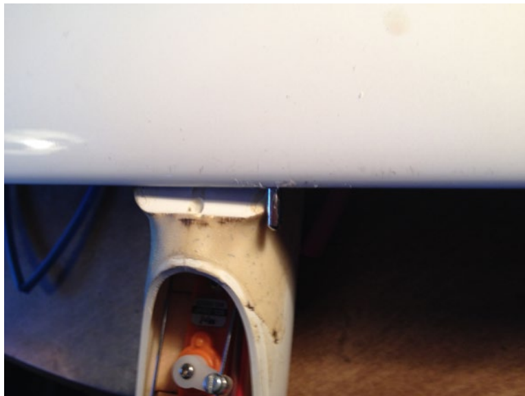
4. The wing pin had slipped out. Also.
