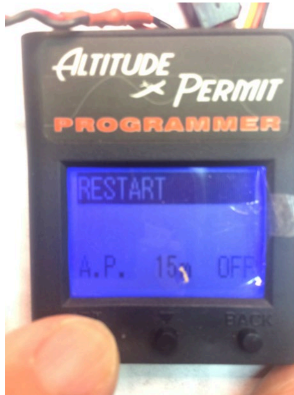
(2) In the SETUP A.P. menu, choose the RESTART option. The bottom line displays "A.P. 15m OFF."
