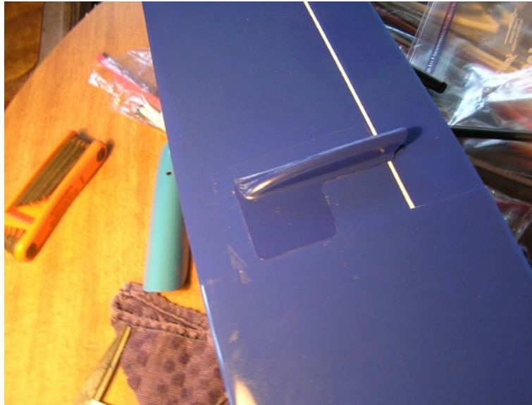
1: The Mini-Elephant pushrod fairing that hid slipping linkages.
