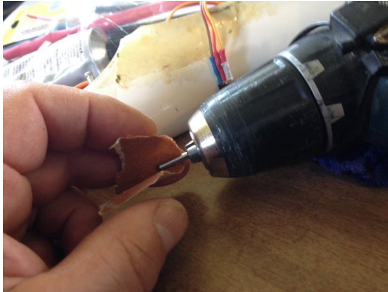
3. Roughing up metal surfaces gives tooth for glue.
