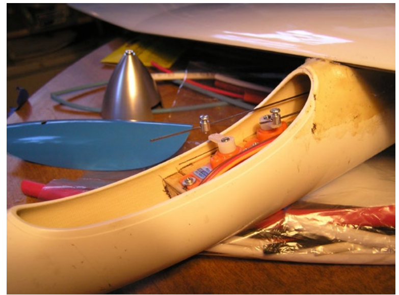
8. The Mini-E/Z connectors were installed without keepers. Better to fix now rather than post-crash.
