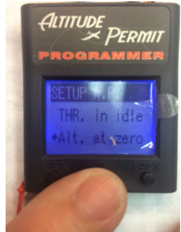
(3) A.P. means Altitude Permit, and allows the motor to be restarted. Here the throttle is at idle (zeroed) and the altitude is set at zero.
