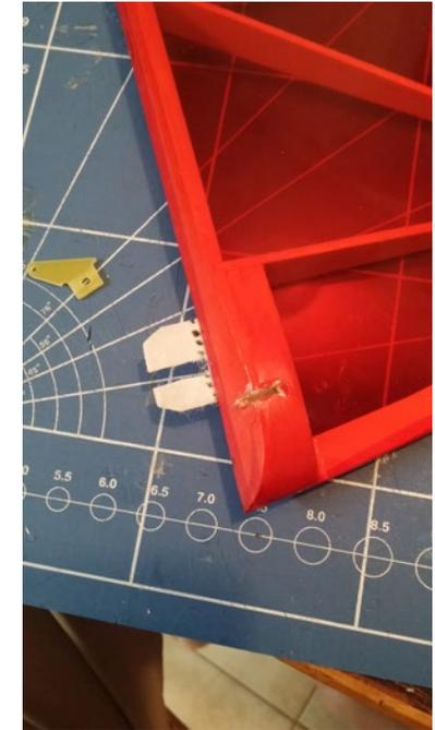
debonder, but the fumes would ruin the covering. Or I could cut into the boom. Naaah. I decided to slice a wedge into the bottom CA hinge.
