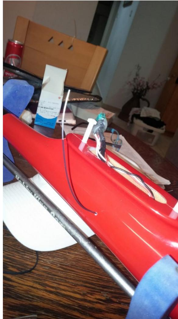
And while I had the fuselage belly up on the table, I also applied a few strips of fibertape, to give some protection against the rough landing areas we have. The last bit of work was assembling everything ready for flight, and see how
