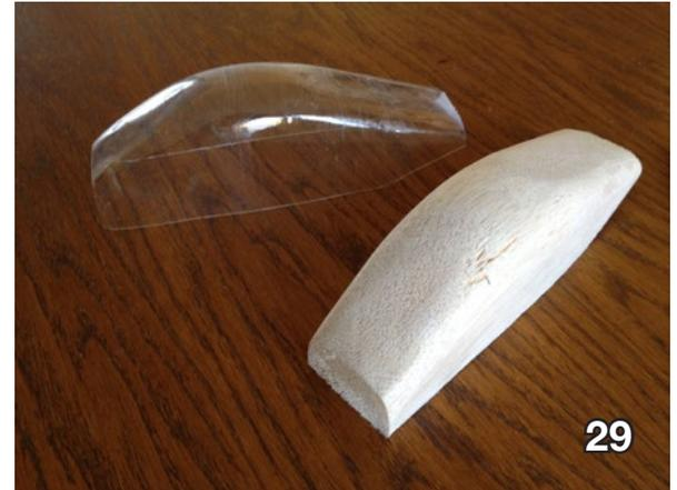
Photo 27: Everything is painfully sanded to the final shape, making sure of its symmetry and that it fits nicely on the fuselage.
