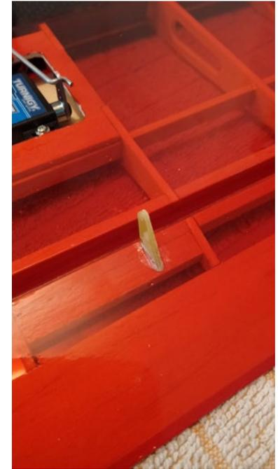
cavity was almost filled I inserted the control horn, and pushed it firmly into place, making sure it was straight.
