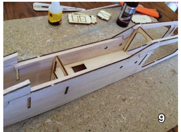
Photos 1 - 5: The fuselage sides are cut in 2mm balsa, and 5x5mm balsa strips are glued all around the edges. (See plan.)
