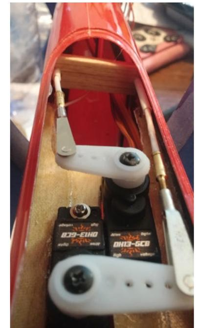
After measuring a few times (with both rudder and elevator surfaces attached) I cut the pushrods down, rough sanded the plastic sleeve, and used 5 minute epoxy to glue the pushrods to the clevis holder.
