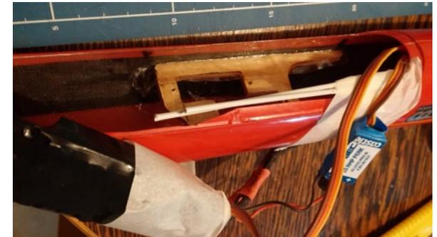
I now realized that the opening I cut for the servos was not exactly in the middle! So I had to cut down one arm by one hole. \*Hmph\*. Not the end of the world, but annoying.
