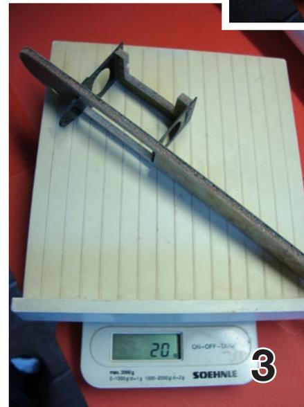
1. Gino innovated when it came to placing the elevator servo in his Tangent Modelltechnik ASH 26, moving it from the cockpit area to the vertical fin. This allowed a direct elevator drive. Here you see the various parts used in this modification.
