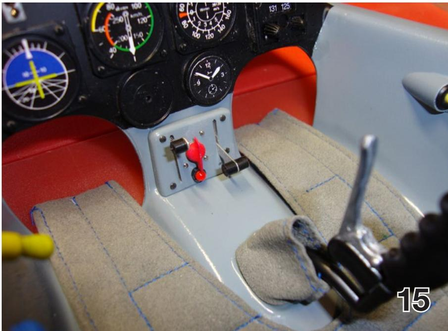
13 - 15. These photos show the cockpit details of Gino's Tangent Modelltechnik ASH 26. Gino assembled some of the cockpit interior with readily available retail parts, like the instruments and the microphone, but most of the pieces were made or assembled from small parts - pins, LEDs, etc. The seat upholstery was sewn by Gino's wife. All it needs now is a realistic pilot!
