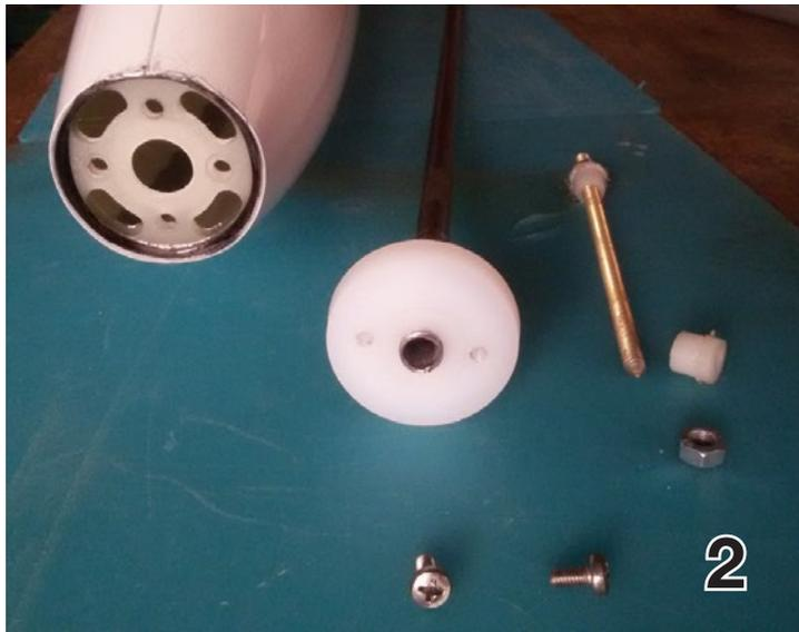
2. In order to get the thrust line set up properly, a simple alignment tool is constructed. Precut the nose so it's 1 - 2 mm longer than the final size. A PVC pattern is then forced into the fuselage. It will hold the motor frame in place while the epoxy cures. Note the tube extending back from the center of the PVC pattern. See also Photo 4.
