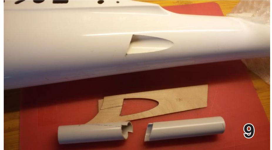
8 and 9. A plywood template was used on a PVC tube to achieve the proper contour for the exhaust opening. The left piece in Photo 8 shows the penciled outline as well as the notches which allow the forward portion of the outlet to be inset in the fuselage. The finished outlet is shown in Photo 9.
