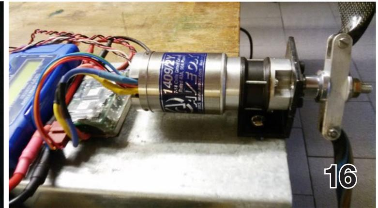
15. Here's the setup for measuring the thrust of the power unit with different batteries and propellers.
