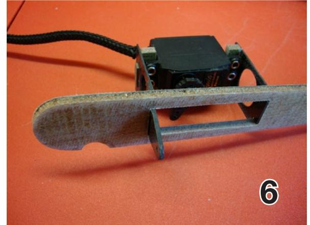
4. The four parts are glued together, creating rigid lightweight framework.
