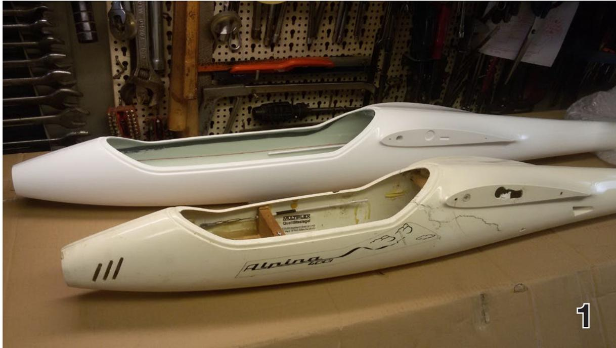
1. The new Tangent “long nose” fuselage, shown at the back, is no longer an ARF product; it requires more handmade items than before. The older fuselage, front, has the nose cutout for the motor mount, and ready made air inlet and outlet. The latter is under the wing trailing edge,
