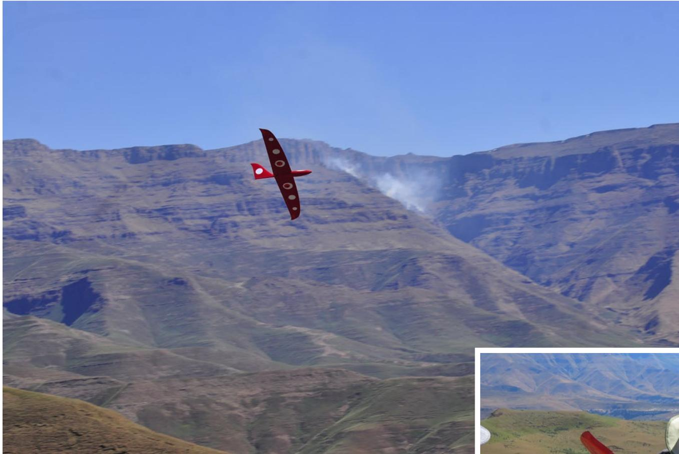
*Above: Evan Shaw's "Dotty," an own-design 'wing, made from old F3B glider wing tips glued together, mounted on an old fuselage front-end with a glassed foam fin. Piet Rheeders*
