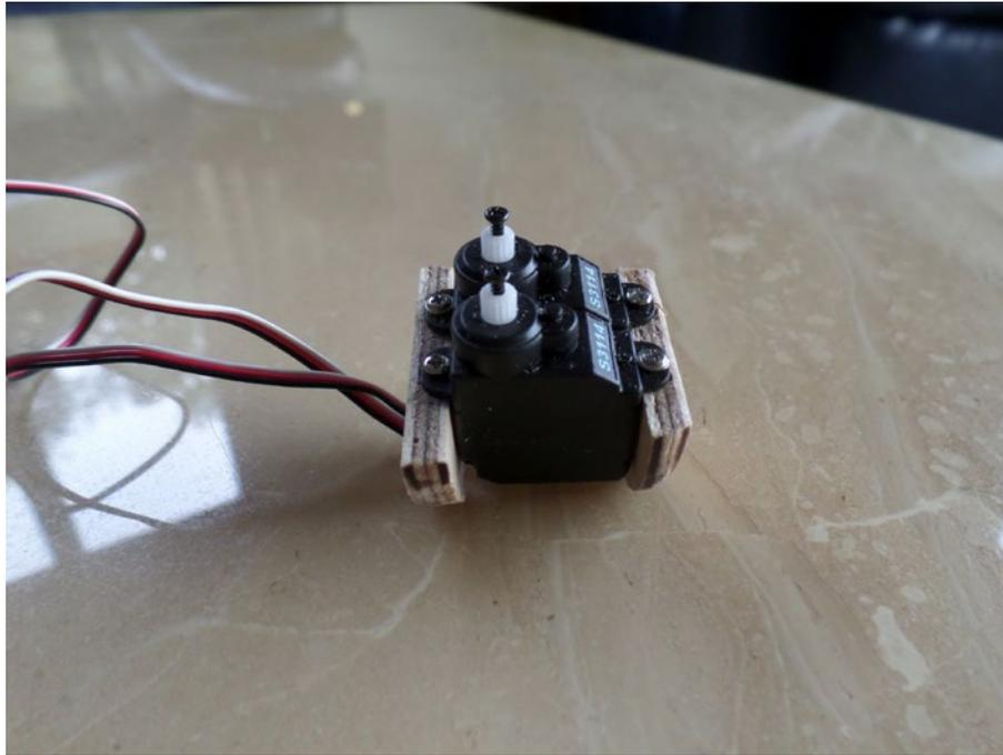
*Rudder and elevator servos mounted to bulkhead to be glued into fuselage*
