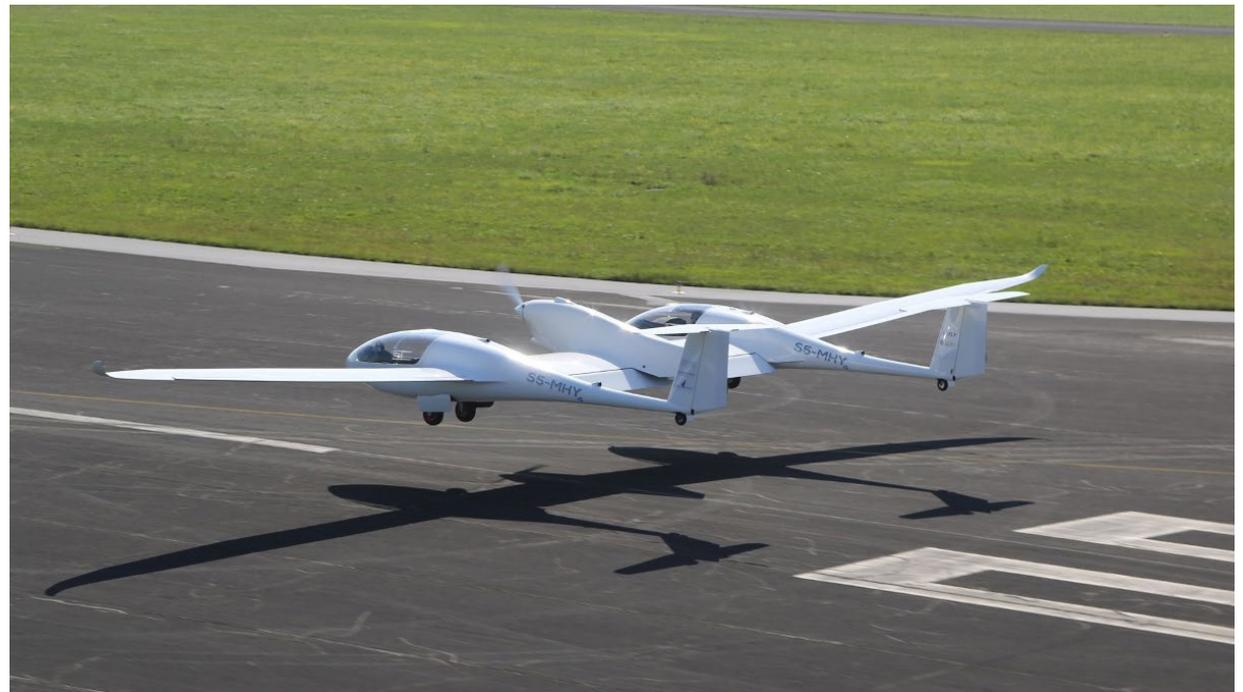
propel the aircraft. A high-performance lithium battery covers peak power loads during take-off and when climbing. If the hydrogen required for the fuel cell is generated via electrolysis using power
