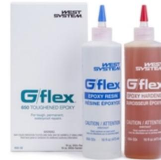
We've used West System 105 resin and West System 206 slow hardener or West System 209 extra slow hardener for vacuum bagging processes. One of the newer West System products is G/Flex. This is a two part system which uses a clear resin and a brown colored hardener. Its main advantage is that it remains flexible after hardening, making a good option for mounting servo frames in wings and mounting plates in fuselages. And it does have significantly greater adhesion than regular epoxy, too.
