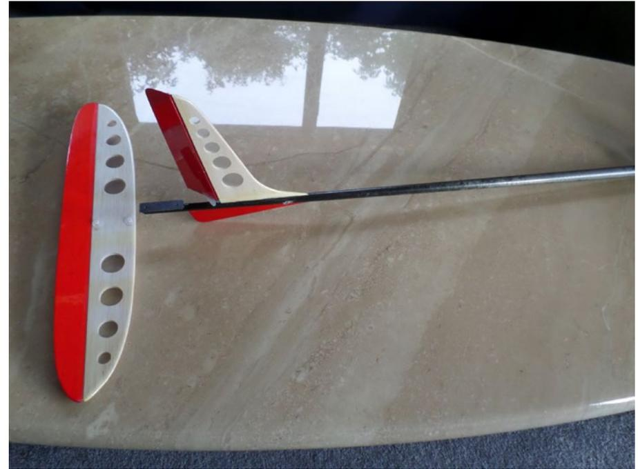
*Rudder already fitted and showing elevator and elevator mount*
