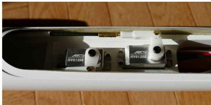
Above: The MPjet threaded coupler are glued and pinched on the snake rod
