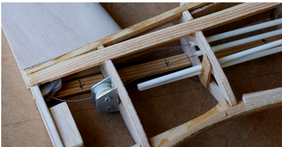
Fuselage assembly, pulley system in the tail
