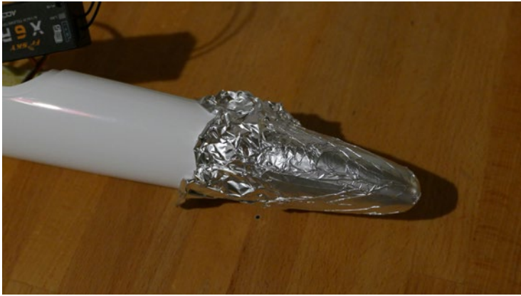
Preparing the mold for the balance lead
