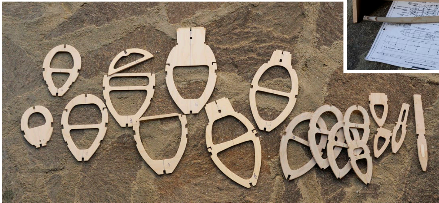
Fuselage lower keel and bulkheads
