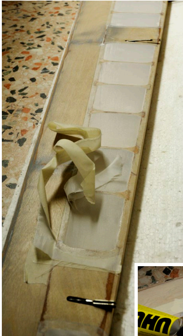
Covering the wing and horizontal tail
