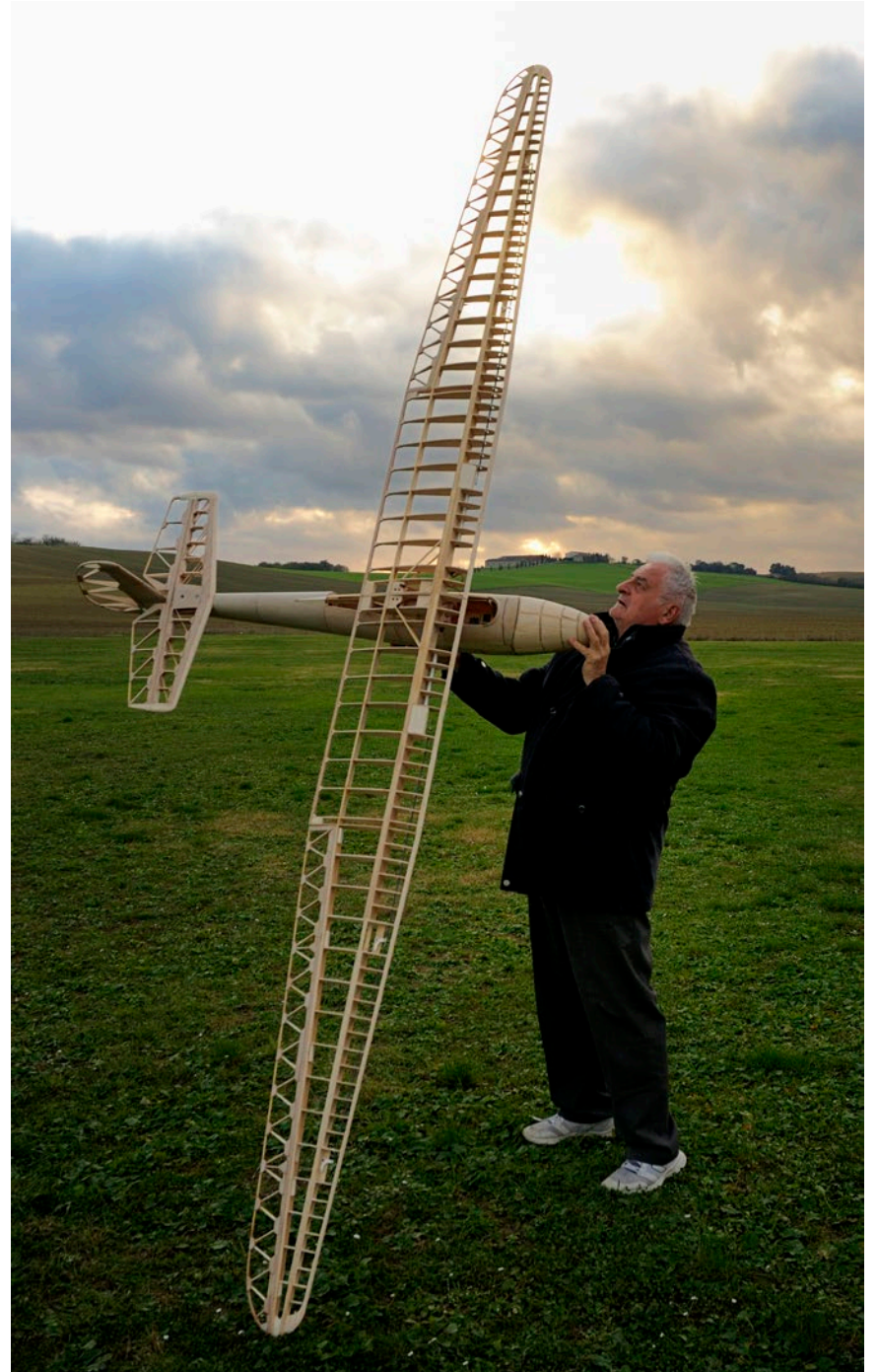
Completed skeleton ready for covering.
