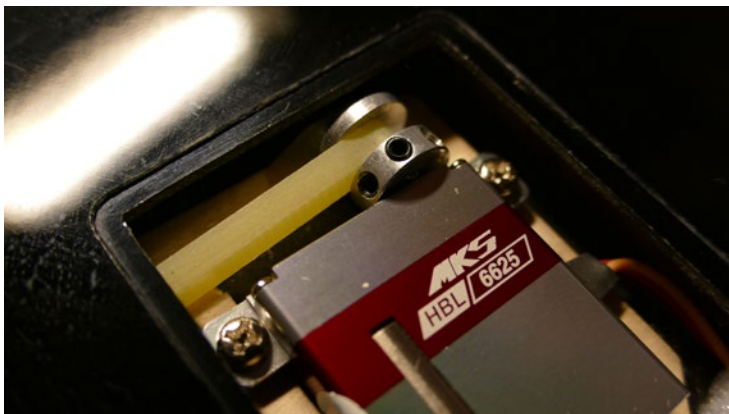
Left: The counter bearing makes the installation very tight and slop free For more information on this system, please see < http://planet-soaring.blogspot.com/2012/07/rdh-and-fu-fix-external-bearing-kits.html > < http://www.sloperacer.co.uk/_content/hardware.asp > < http://www.sloperacer.co.uk/_content/externalbearingkits.asp >
