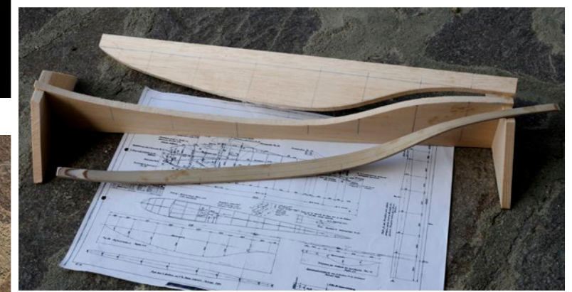
Fuselage lower keel and bulkheads
