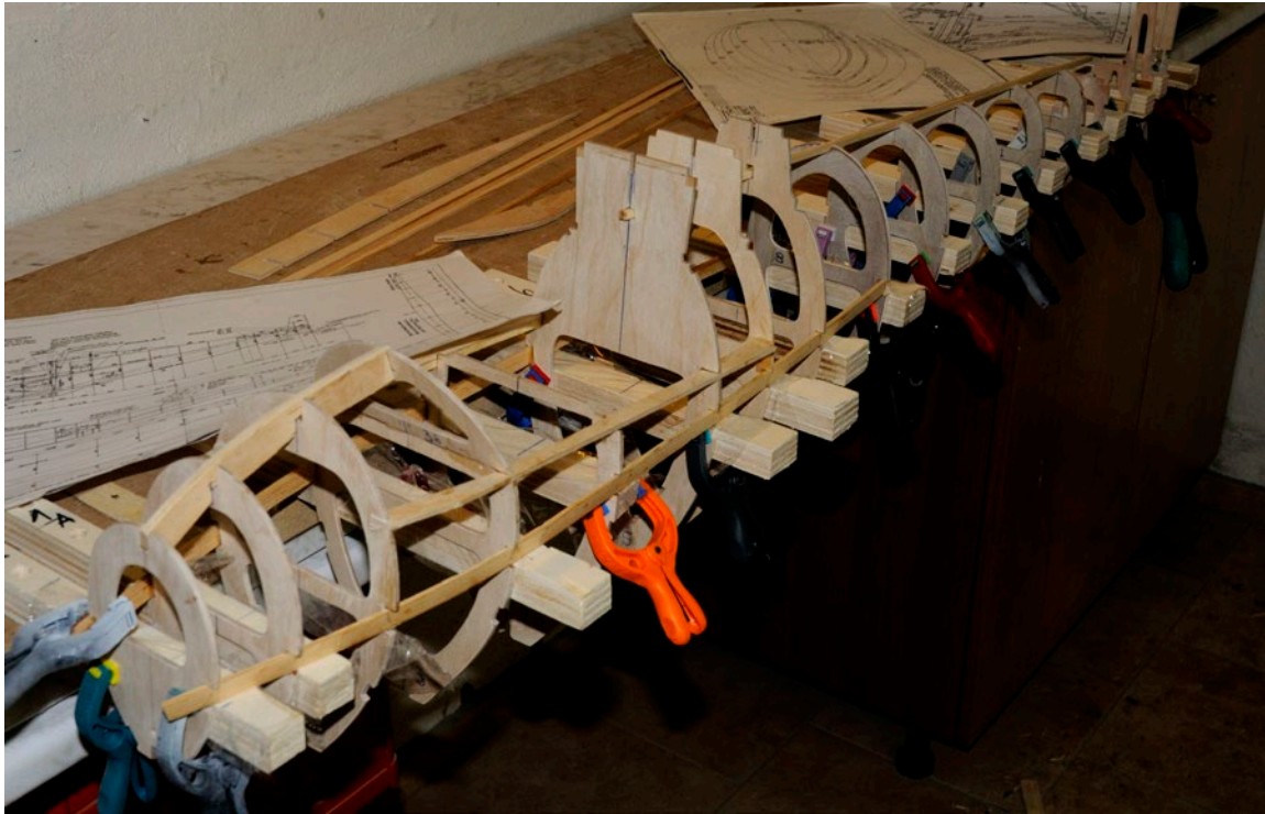
Fuselage assembly, pulley system in the tail
