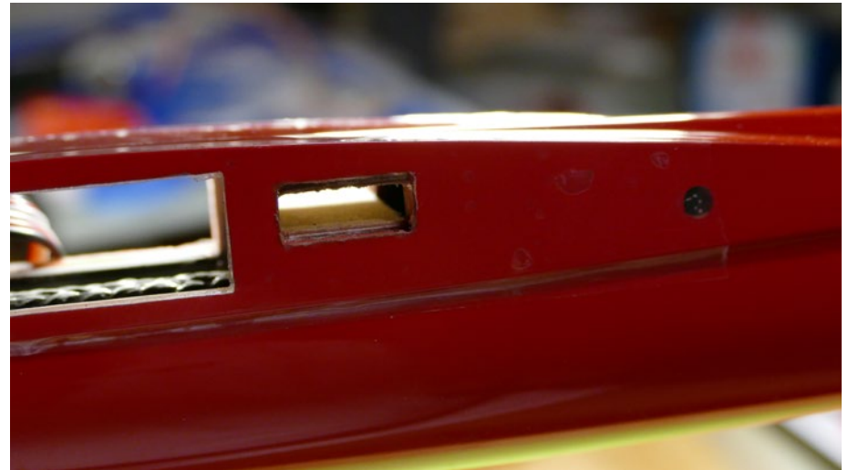
The wood plate installed in the fuselage to host the 6-pin plugs
