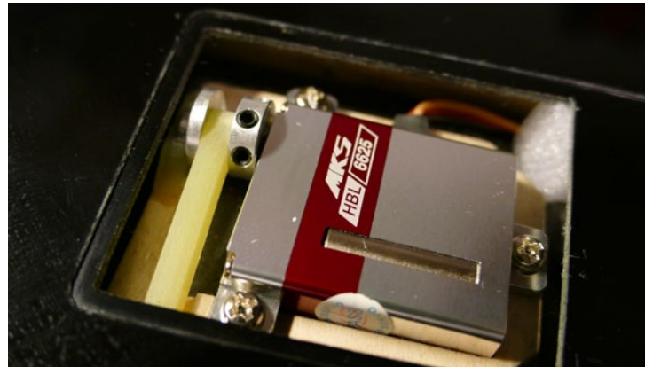
Far left: The two MKS HBL6625 servos in their servo frames
