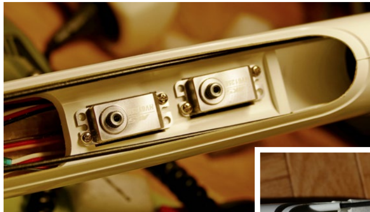
Left: The two elevator servos in place
