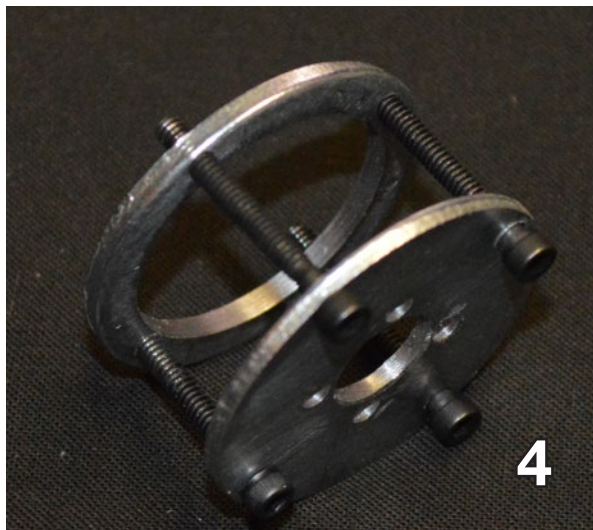
Completed motor mount.
