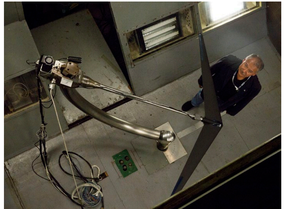
Al Bowers and the wind tunnel configuration used for researching a model of the Prandtl-d are seen from above. Photo credited to David C. Bowman at < https://www.nasa.gov/feature/new-wing-shape-tested-in-wind-tunnel >.
