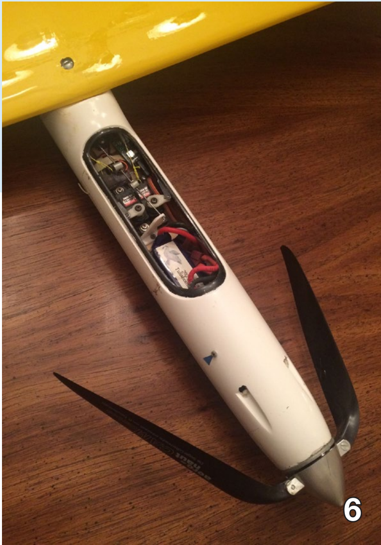
The servo tray in place. Notice the spoiler activation system which is driven by a single servo and is entirely adjustable.
