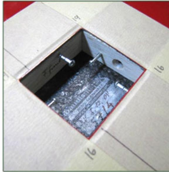
The blocks are in. The screws are temporary handles to help position the pieces accurately. Holes for the servo wiring and a linkage slot are cut into the blocks before installation.
