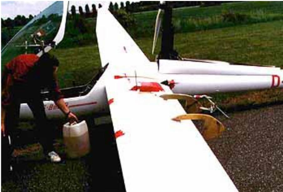
*Measurement of the Airfoil-Drag of a DG-800B*
