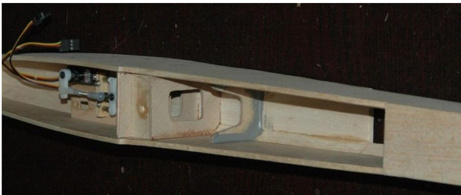
Figure F5: Mid-fuselage bulkhead installation
