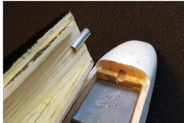
Figure F19: Hatch cover retaining pin
