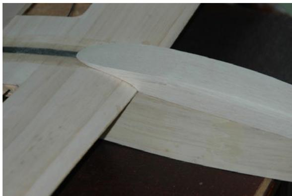
Figure F17: Hatch cover rough shaped
