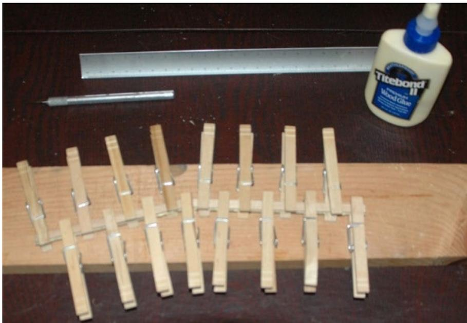
Figure W1: Laminating the tip joiner
