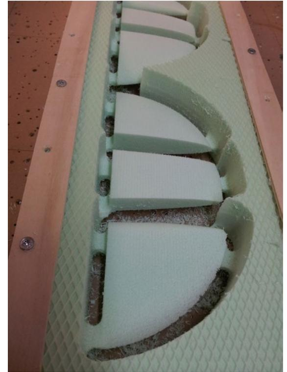
*Wings finishing is milled three-dimensionally from Styrodur*
