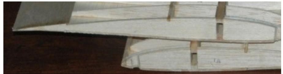
*Figure W14: Wing mounting bolt notches at the front of the root ribs*
