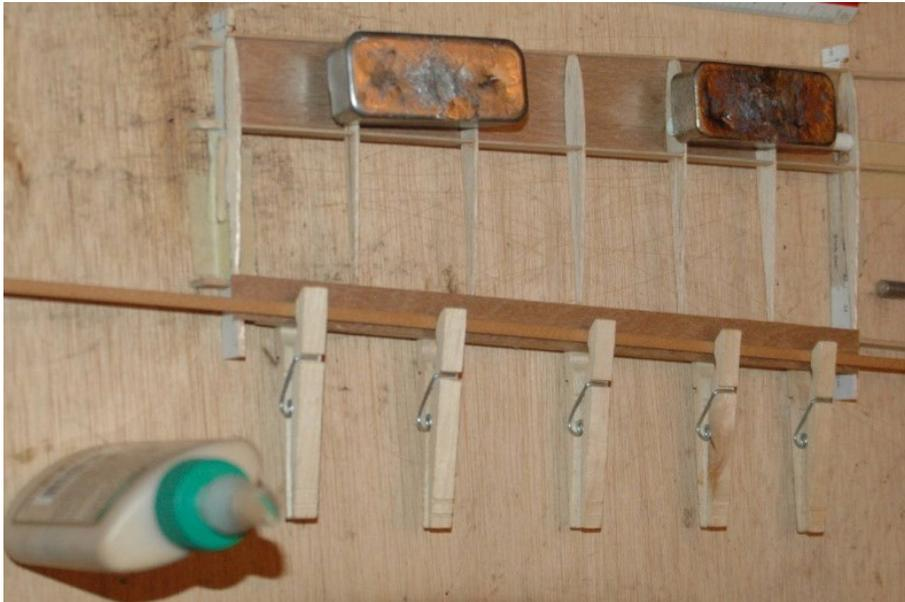
Figure T5: Closing the stab trailing edge
