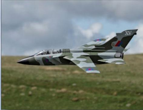
Front cover: Steve McLaren's Panavia Tornado GR1, built from the Andy Conway PSS plans. Model spans 40" and has an AUW of ~3lb. Hand painted finish in the colour of RAF 15 Sqn the model is regularly flown with wingstores to great effect! Model is seen here soon after launch at the Bwlch, South Wales, May 2016. Photo by Phil Cooke – PSSA – more info at <<http://www.pssaonline.co.uk>>.
