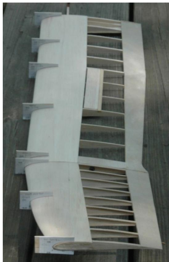
*Figure W25: Wing with lots of leading edge templates*
