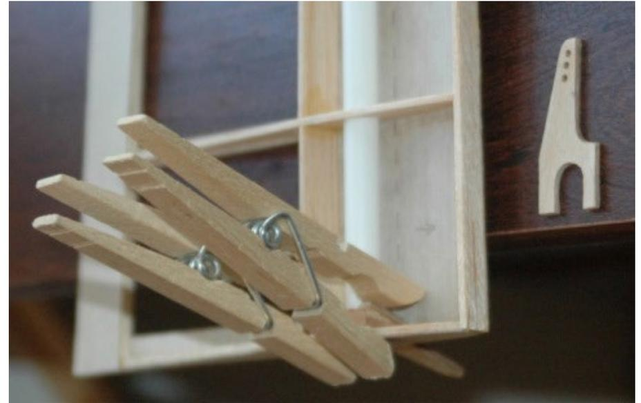
*Figure T3: Control horn installation*
