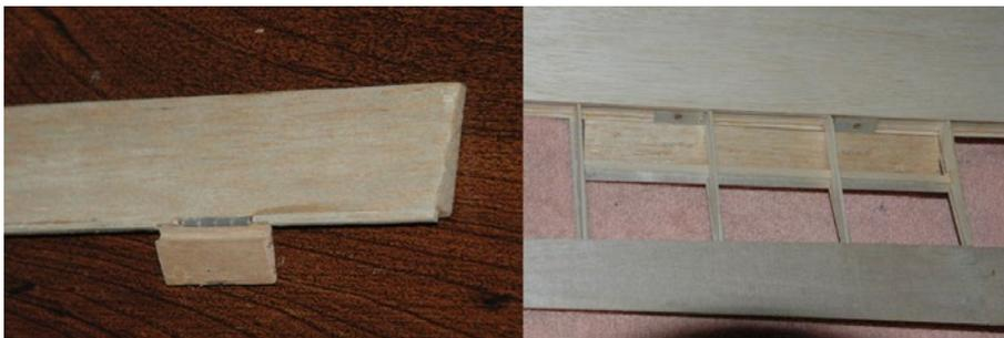
Figure W19: Spoiler installation details
