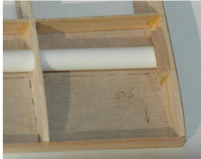
Figure T1: Tail root rib with control horn wedge.
