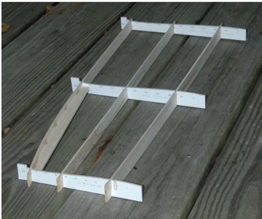
Figure W21: Tip panel jig
