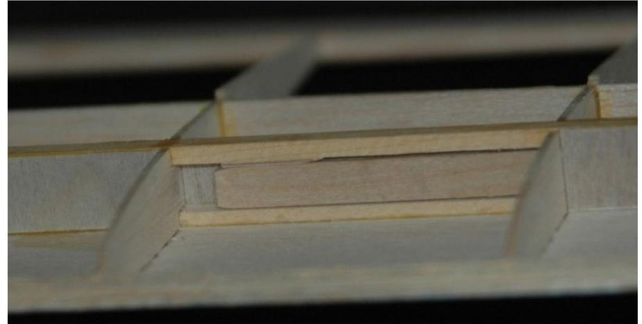
*Figure W13: Tip joiner spacer wedge installed*
