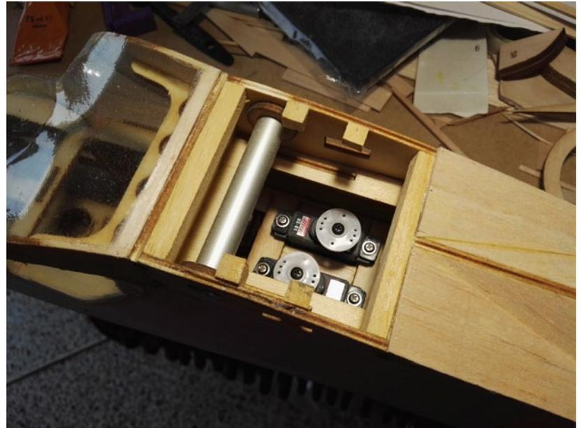
the rudder I decided to use the classic pull-pull cables, while for elevator I preferred to use the same method already used on my Grunau Baby. A small threaded rod hinged to a rigid wooden dowel coming from the servo and secured to the hole in the elevator through two M3 nuts.
