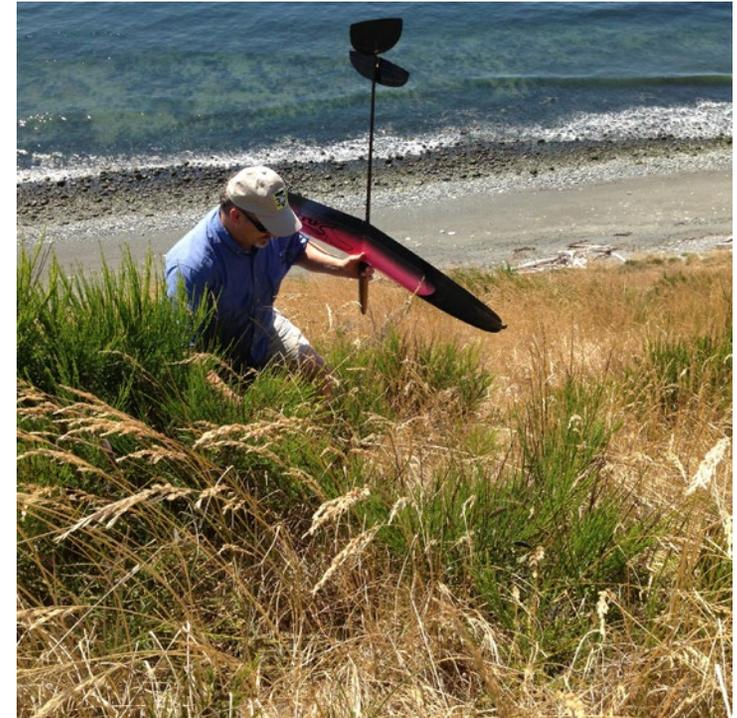
About then the air decides the glaciers were right. The wind sheers straight from the north. Zero slope lift. Steve does some fine discus launches until his Snipe catches a wingtip in the grass, ground loops, and cracks the support of the vertical stab. Easily fixable, but not here. Whidbey Island has played catch-and-release with us, released back to Seattle.
