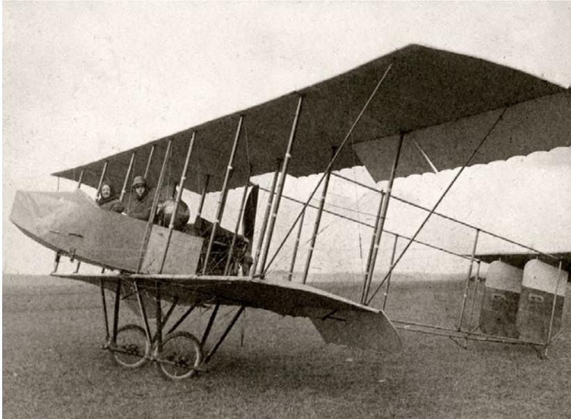
*A 1912 Farman HF.20 biplane with single acting ailerons hinged from the rear spar. The ailerons hang down when at rest and are pushed up into position when flying by the force of the air, being pulled down by cable to provide control.*
