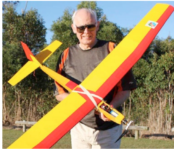
To enter the Millennium Cup, chop the nose off your favorite 2m glider and add an outrunner, as in this image showing David Lucas with a Drifter 2 converted to electric with a Scorpion outrunner.
