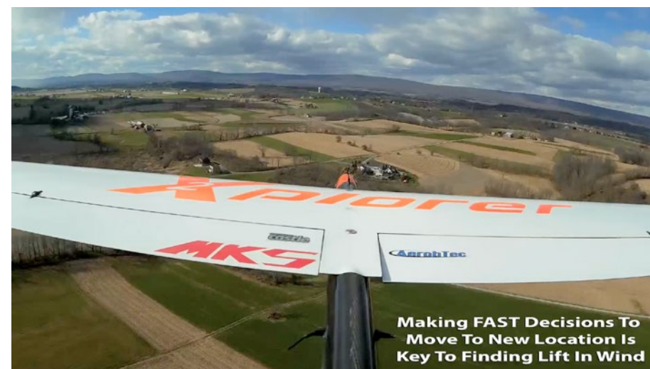
From Thermal Soaring Master Class 2: A tail-mounted camera shows flap position while searching for lift under windy conditions. In addition to verbal commentary, “subtitles” are often used to highlight specific points.
