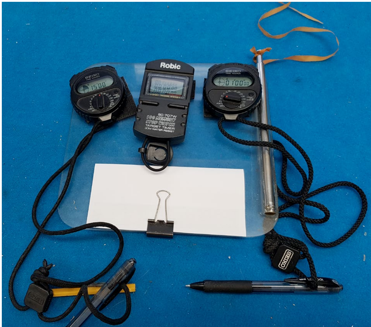
Three stopwatches - two Seiko Time Keeper models (left set for 15 minute countdown, right set to 1 minute count up) and a Robic SC-707W, an older transmitter aerial with light ribbon, clipped paper supply, and pencil and pen make up the author's personalized Timing Board.
