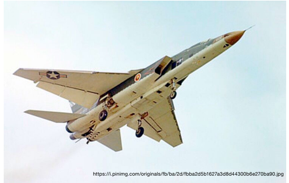
The “canoe” on the fuselage bottom held an array of sensors and cameras. Notice the huge flaps.
