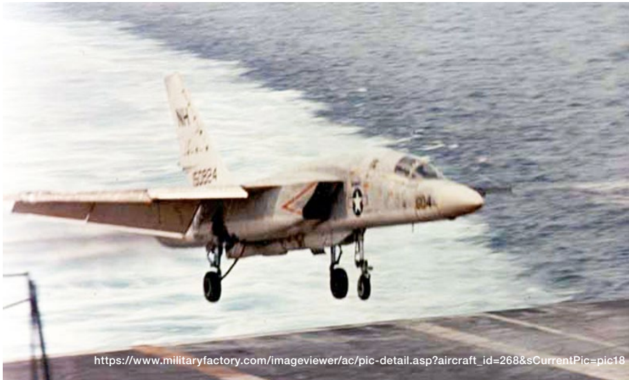
Coming over the edge of the carrier deck, note the flap deflection, leading edge slats and high angle of attack.
