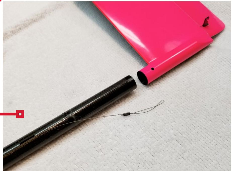
Pay attention to the detail in the online plans on where to install the pull cable keeper. The dimensions shown on the plane will make sure the keeper is installed on the wire so the keeper is past the end of the boom which makes threading boom and pull wire through the joiner and rear keepers easier to do.
