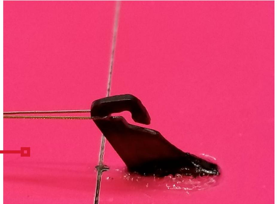
Where the A-tails come together at the top, two pins align the surfaces and then a piece of tape holds them together.
