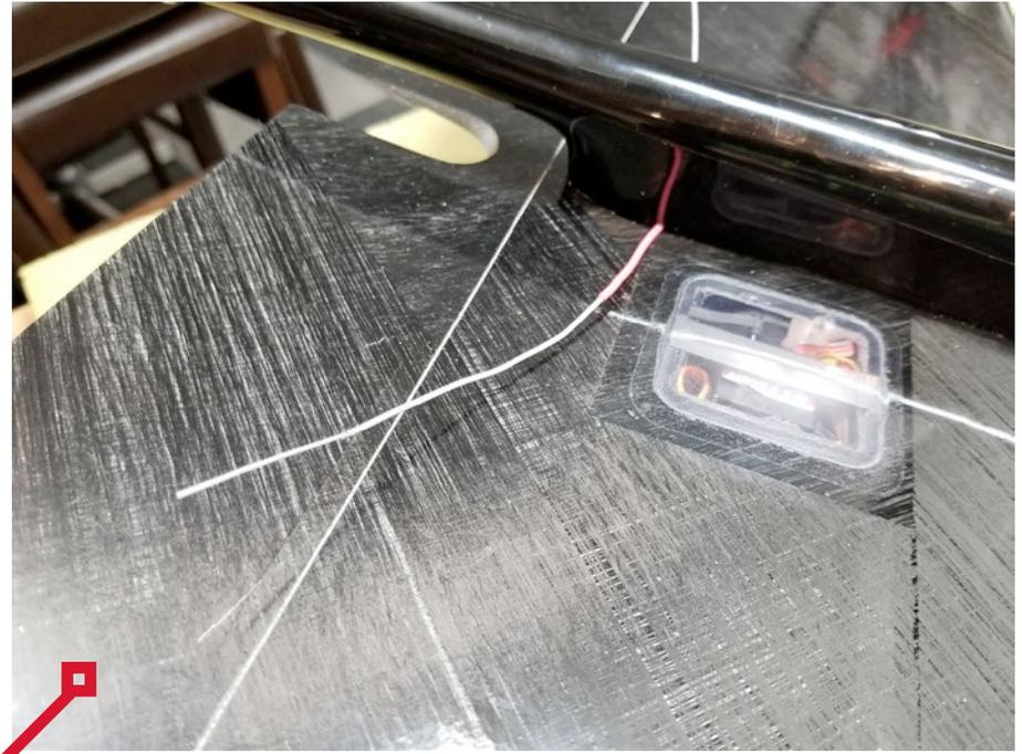
an eight channel Futaba receiver and it is a tight fit. I fly Spektrum and wound up using a Spektrum nine channel AR9310 with the case removed.
