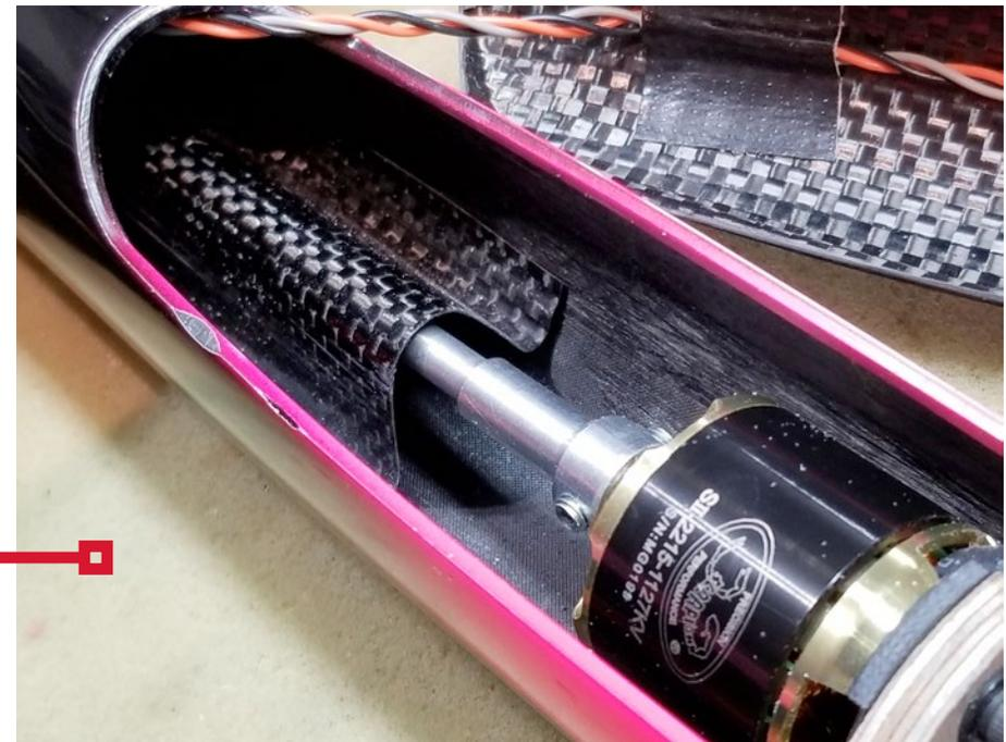
Vladimir also came up with an interesting ballast system. The ballast system is composed of lead blocks that slide on or off a wire keeper system. The blocks can be moved forward or backwards on the wire keeper to adjust the CG. The whole assembly slides into the pod and over the propeller drive shaft. Then you lock it in place with a screw. A full load of ballast weighs 17 ounces.
