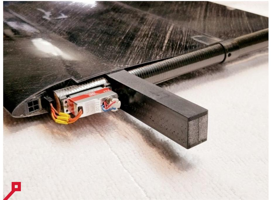
Third, there is a hole in the rear keeper. Align the hole in the boom with the hole in the rear keeper.
