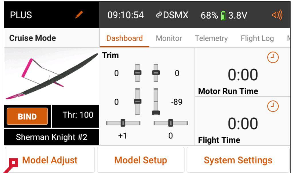
My radio of choice is the new iX12 from Spektrum. The Sailplane program for a 2-Flap, 4-Aileron wing works great and the color touch screen is easy to use. In Cruise Mode, I wound up with little if any differential on the inboard ailerons and about 2.0 : 1 for the tip ailerons. Aileron to Rudder mix was only 3/16th of an inch at full aileron stick deflection. In landing Mode, the Flap comes down to 80 degrees and inboard ailerons to 45 degrees. Tip ailerons droop a little in landing mode.
