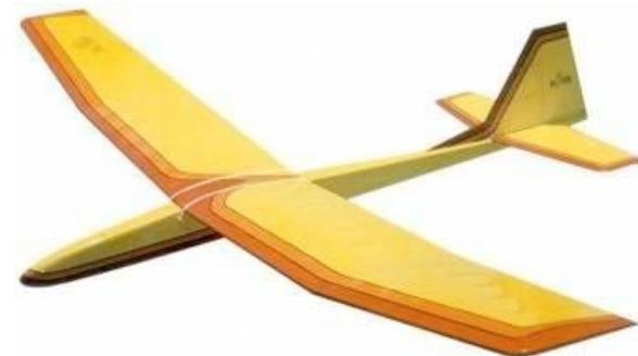
came with a plastic fuselage, power pod etc. that is allowed in the Fun Fly Class. Molded or carbon wing leading edges and booms are not allowed. Small changes to improve the glider's appearance are allowed and encouraged.
