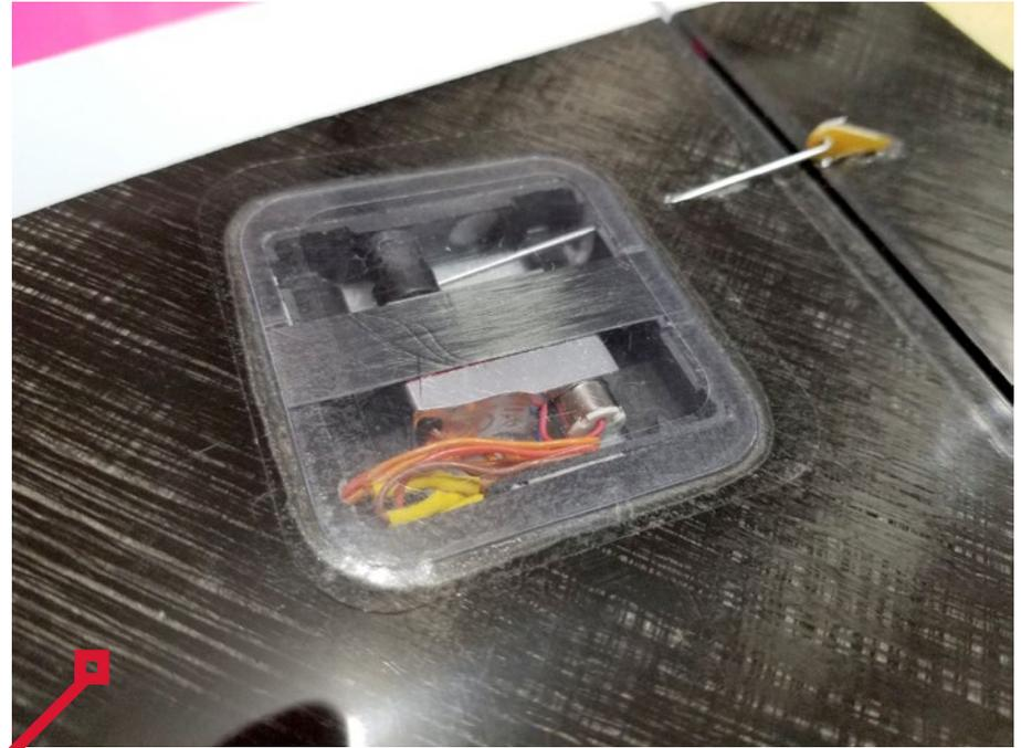
The linkage for the tip ailerons comes through the lower skin of the wing and connects to a short control horn on the tip aileron.
