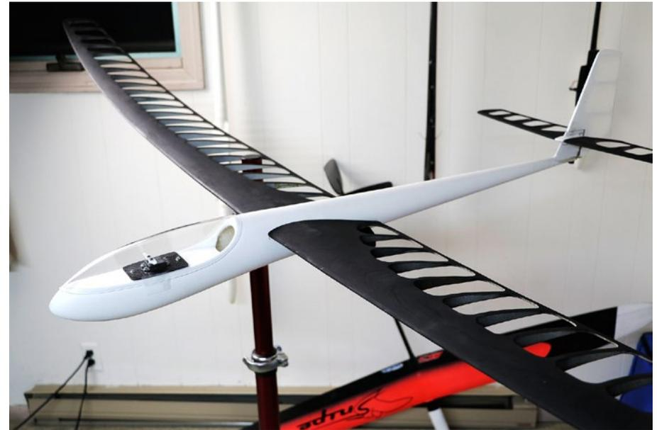
*The wings and stabs repaired and ready to cover. Sprayed the wood with flat black paint to hide the plywood which was stained orange from the original Monokote. I think a black stain would have worked better as the Ultracote covering adhesive interacted with the flat paint and caused blemishes.*
