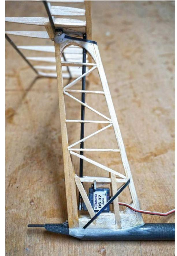
*Vertical fin showing servo location and carbon rod elevator transmission.*
