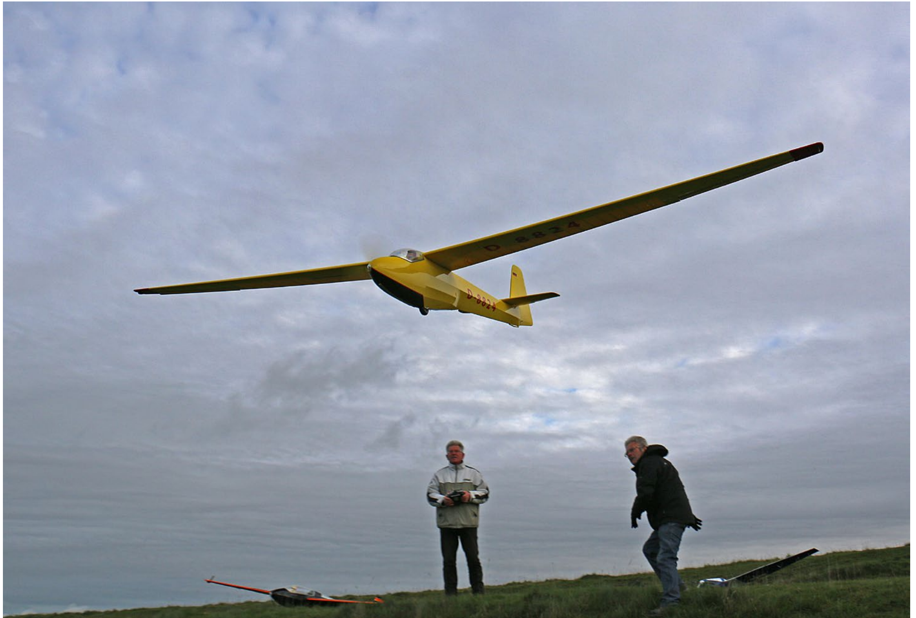
Zugvogel launch. It's often safer to launch a large model powered up.
