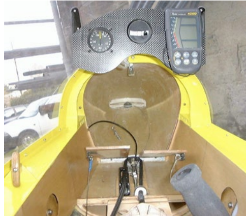
Cockpit detail. Note hand-slot for holding fuselage during foot-launch.
