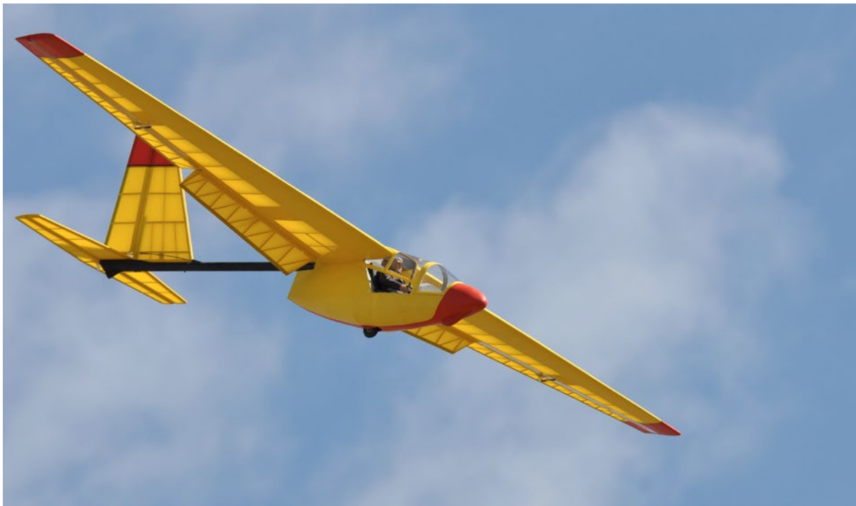
Lee Chaplin's 1/4 scale Carbon Dragon with separate flaps and ailerons on final.
