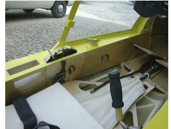
Cockpit detail. Note hand-slot for holding fuselage during foot-launch.
