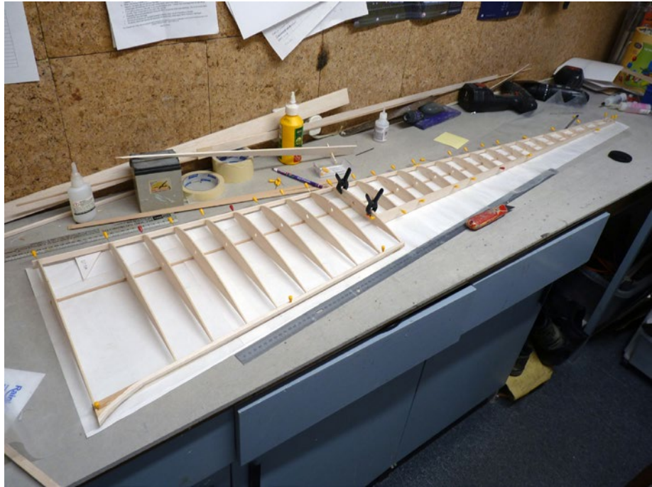
Figure 2. Wing at first built flat on the board.
