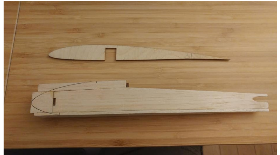
Fuselage box constructed completed. A bit of shaping is all that's needed to finish.
