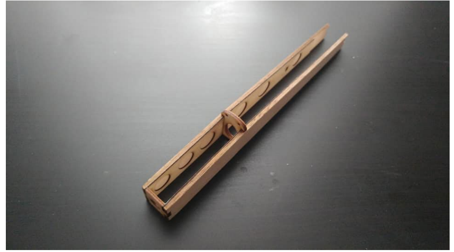
Fuselage construction started. Sides and doublers put together, front two bulkheads installed.
