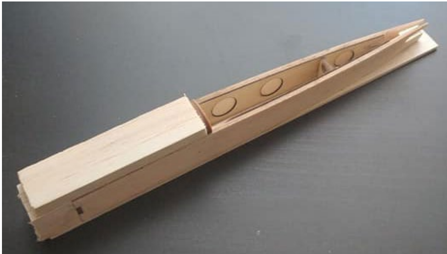
Nose block attached and hatch put into place, rear bulkhead installed and rear of fuselage brought into appropriate taper.
