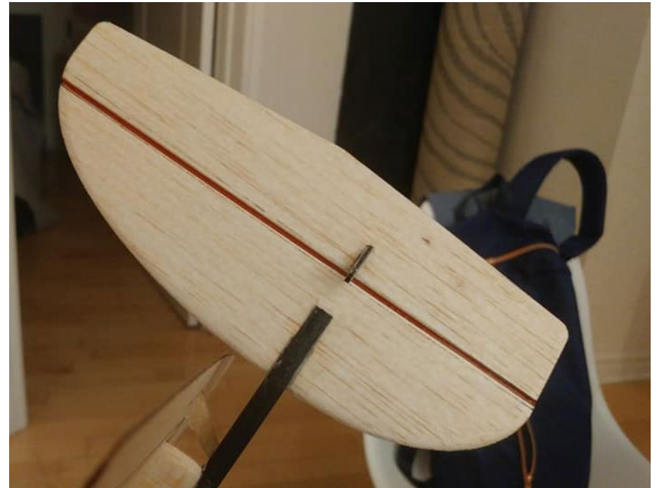
Vertical fin and rudder hinged and mounted.
