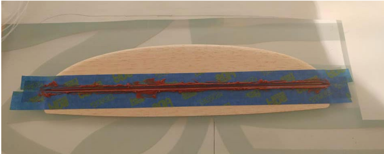
Making the flexible elevator hinge.
