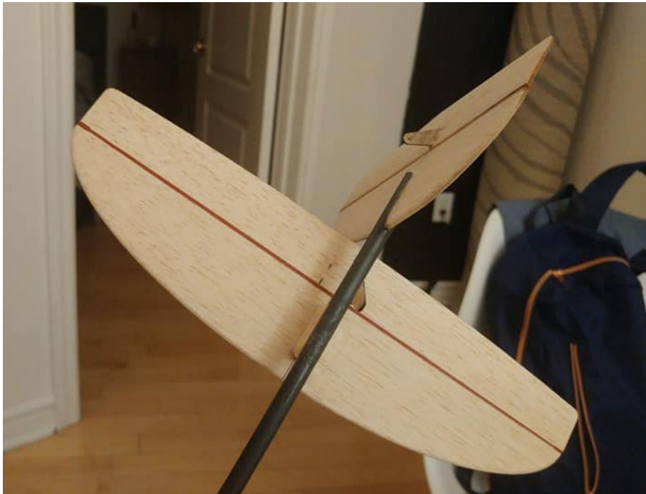
Stabilizer/elevator mounted to boom.
