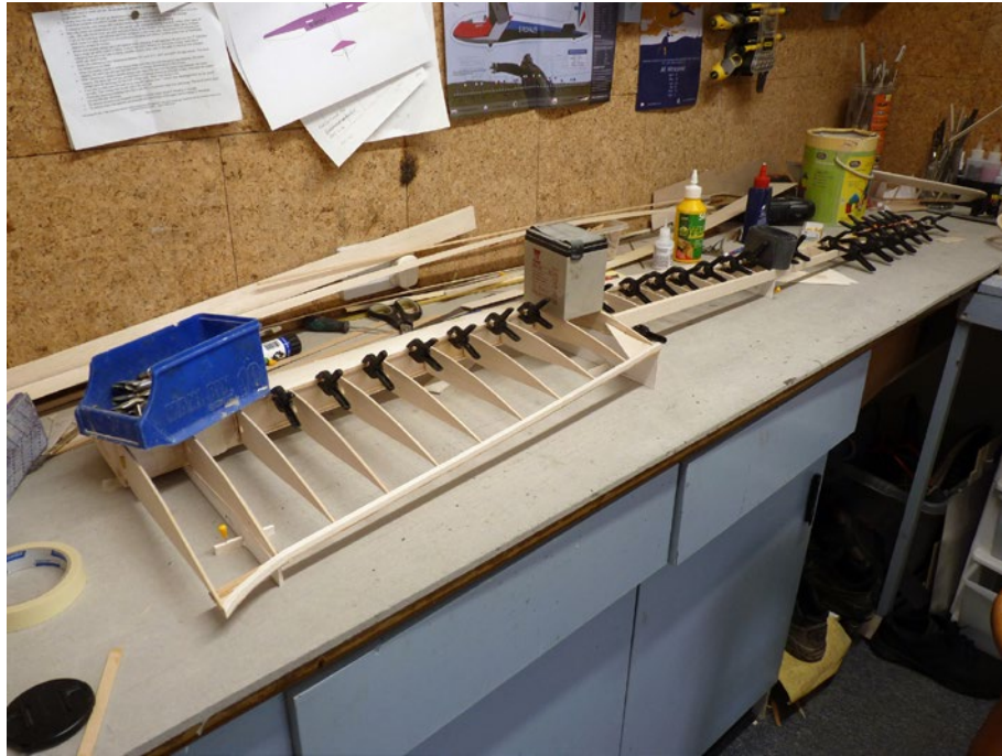
Figure 8. Top sheeting added.
