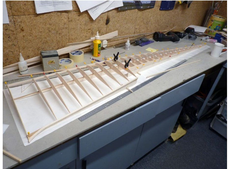
Figure 3. Wing laid up on jigg supports.
