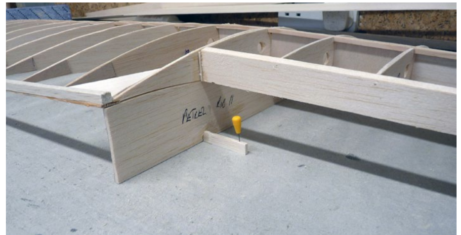
Figure 7. With the lower sheeting in place the wing is placed on the jiggging supports.
