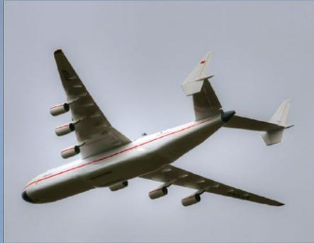
**Front cover:** Andy Meade's Antonov An-225 Mriya at Long Mynd, Shropshire Hills, Shropshire, England. This is a huge model: 6m span, 42 lbs. Made from veneered foam, then HobbyKing film over that. Radio gear includes 14 servos, two receivers, and four battery packs. Canon EOS 7D Mark II, ISO 160, 1/1600sec., f6.3, 324mm
