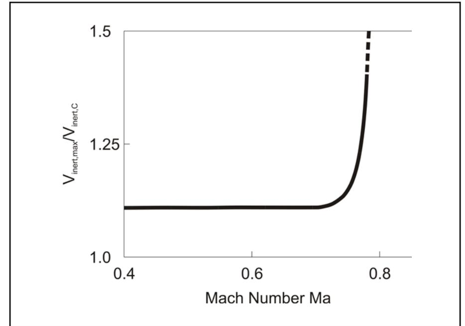
Figure 7. Effect of compressibility on the relation between  $V_{inert,max}$  and  $V_{inert,C}$ .
