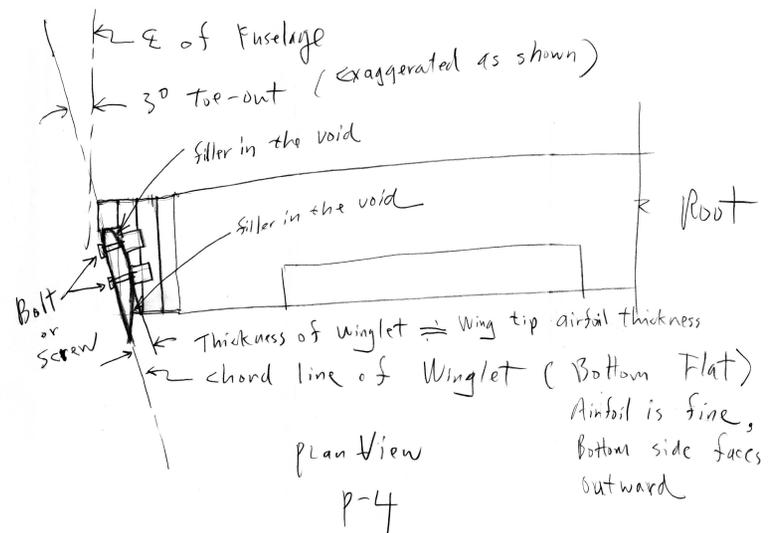
an inward lifting force is created in flight. The winglets are fiberglassed (only at the base) and covered with heat-shrink film.
