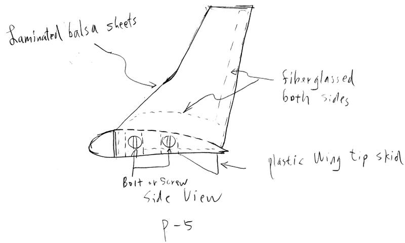
should be self-explanatory. The dimensions of the winglets: about 1/8-inch thick, about 2.5-inch at the base from LE to TE and about 3.5-inch from base to tip. The additional weight of winglets is nil for 4-meter size gliders.
