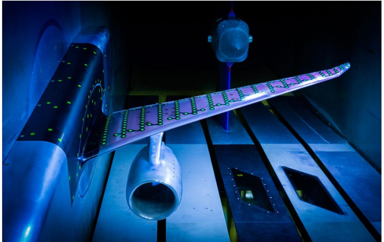
is ‘flutter,’ where the vibrations of an aircraft structure interact with the surrounding airflow in such a way that their amplitudes increase rapidly.
