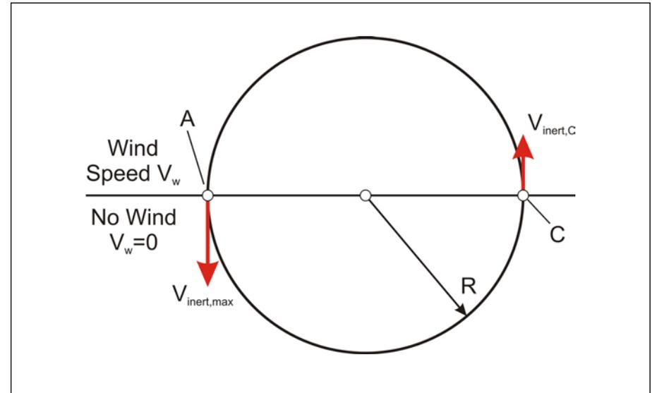
Figure 4. Modelling of dynamic soaring loop for dealing with maximum speed.
