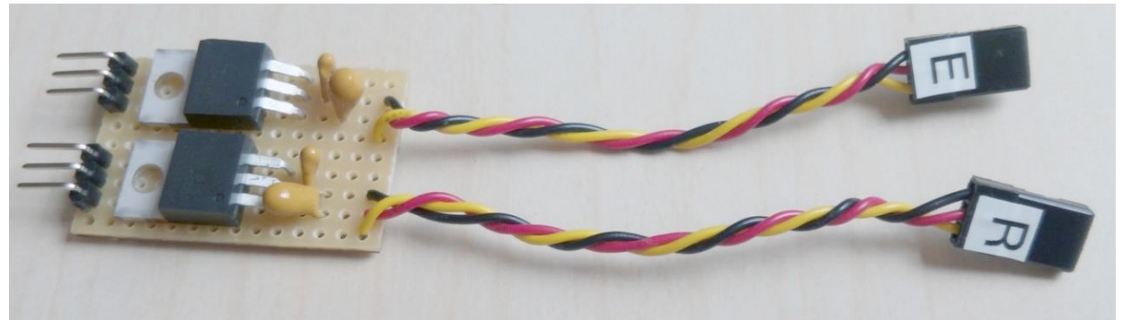
Two LM 2940 regulators on the same board
