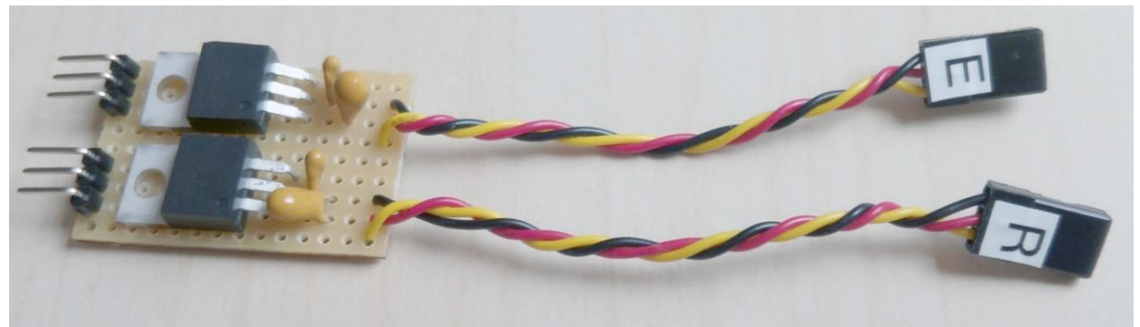
Two LM 2940 regulators on the same board
