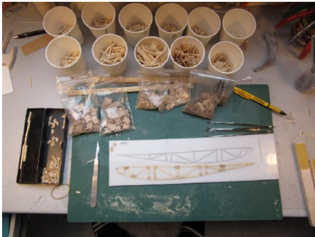
Wing rib production at full speed. In the foreground the milled jigs from Delrin. Behind that the gusset plates, about 2000in all ! All the wooden battens have been cut to size. (image: )
