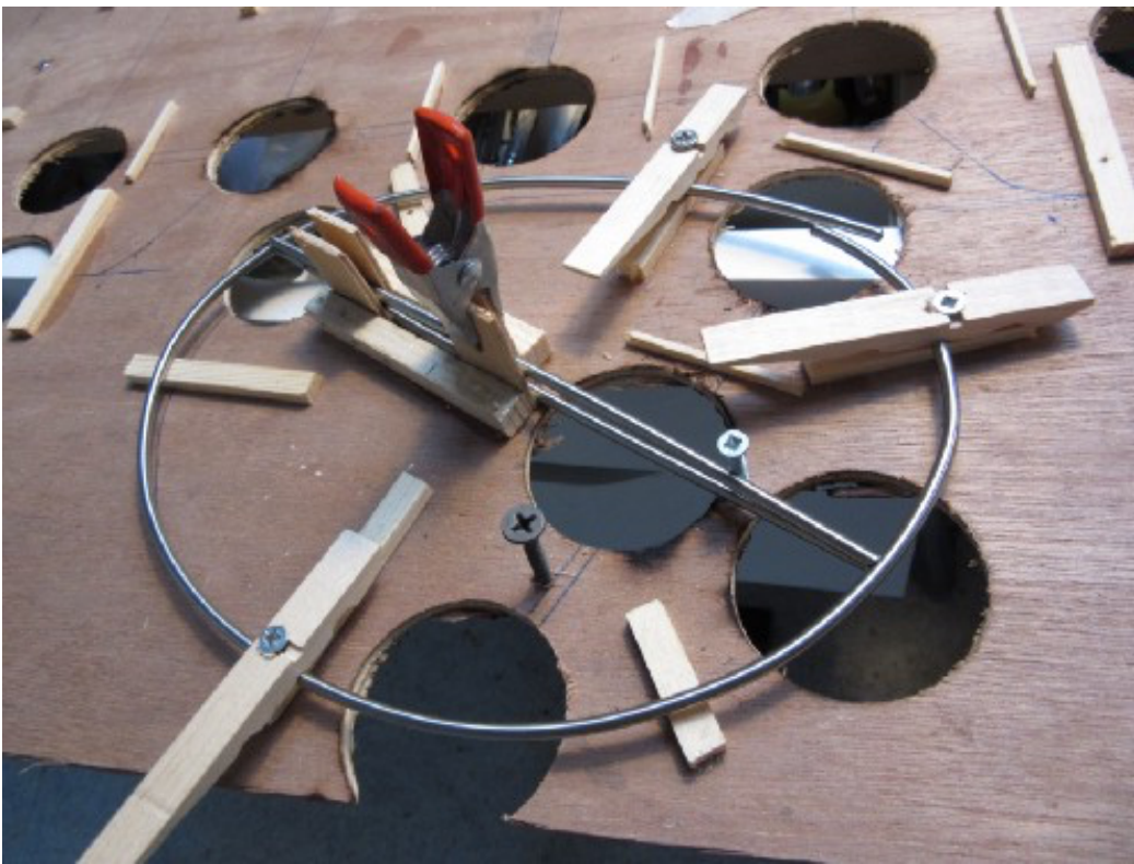
A rudder under construction. Because of the thin walled tube, one covered rudder weighs only about 30 gram. (image: )
