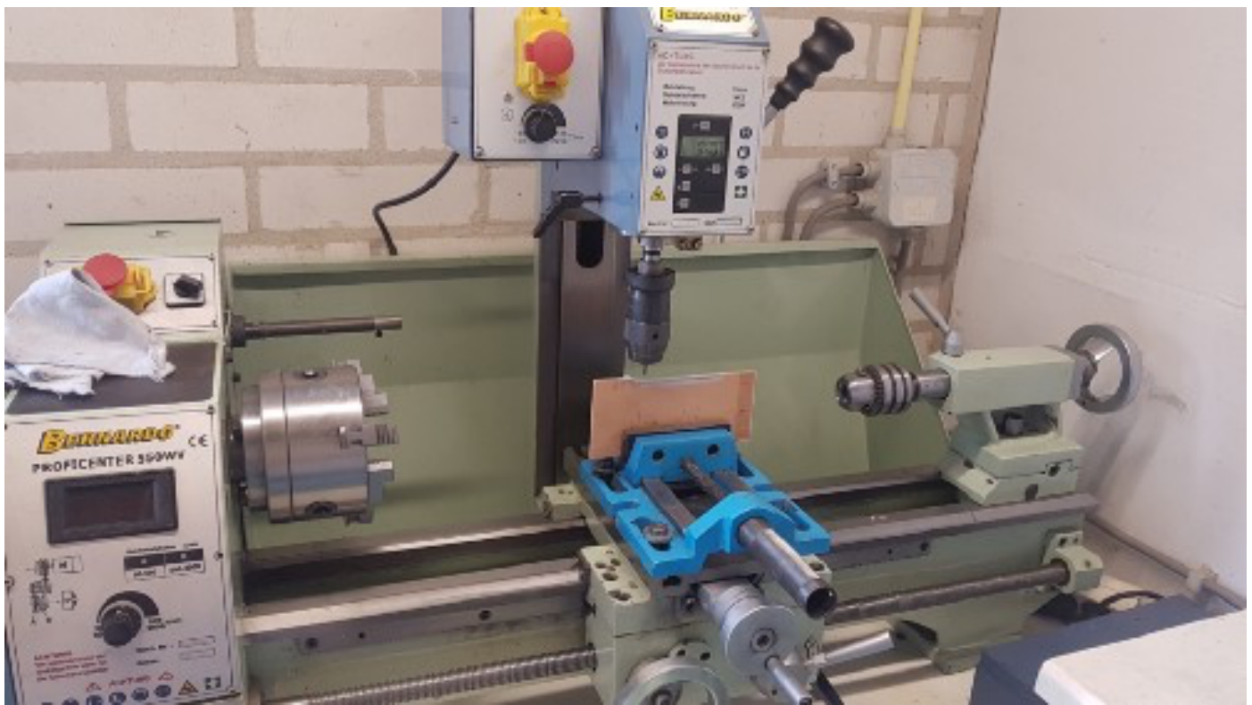
Photo 3: Imprint of the tip airfoil. Photo 4: Measuring on the milling column, with 0.01 mm resolution
