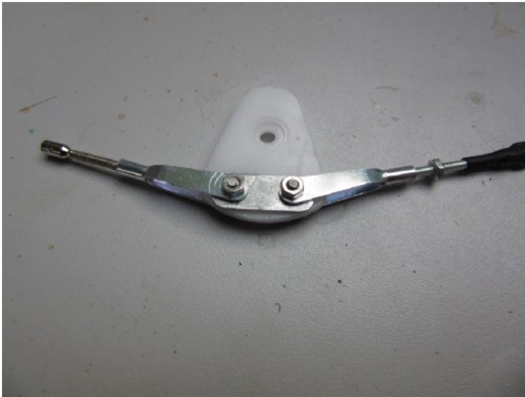
Detail of the modified servo sector plate. The quicklink is drilled out and is connected with an M3 bolt through a bush. This is a vital and heavy loaded part of the controls . At full throw the servo consumes 2A, at half throw it's 0.7 Amps. The servo is rated for 2.5 Amps. (image: )
