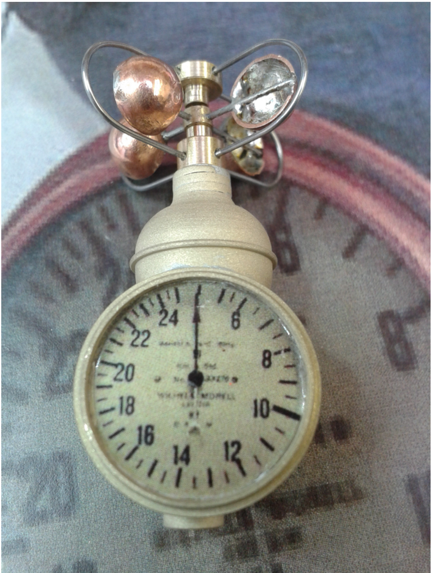
Left: The two instruments. The “anemometre Wilhelm Morell” rotates when the aircraft is flying! Middle: The
