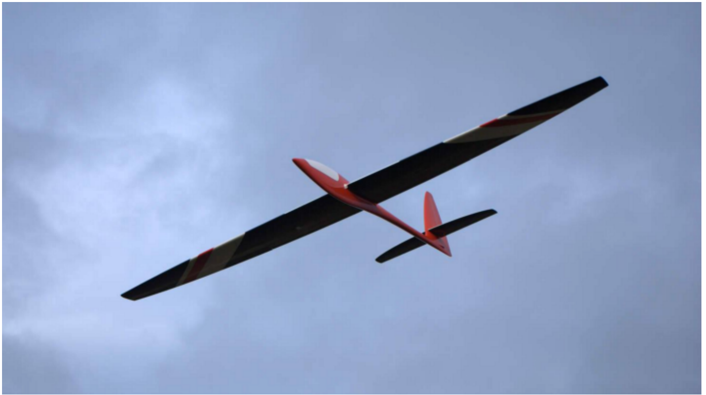
Photo 4: Aresti 80 on a low pass — note the wing shape to give good lift distribution.
