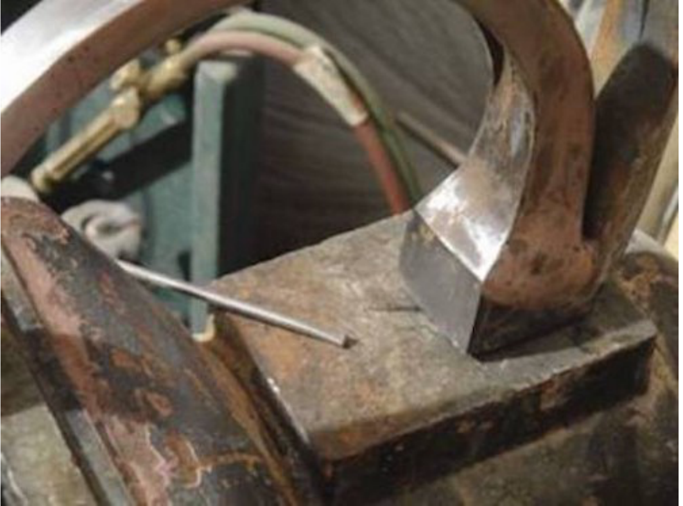
Left: After playing around a bit, I found that 1/8" stainless steel rod, anywhere from 8 to 10" long was just fine. I settled on 9" (half of the 18" rods I had laying around). Right: Next thing was to flatten one end and start making it curved.
