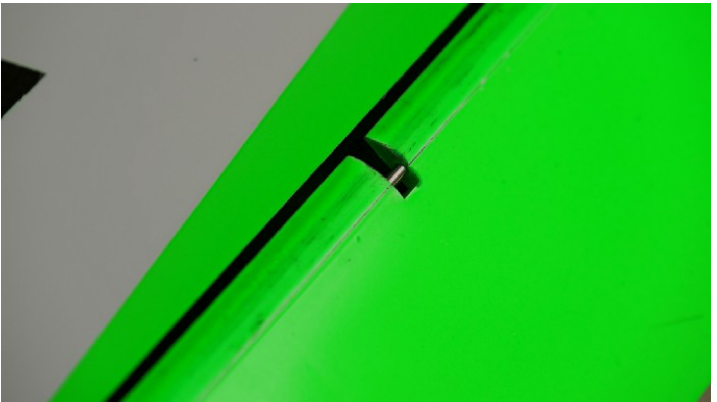
Photo 4: Removable LDS axis on the control surface side
