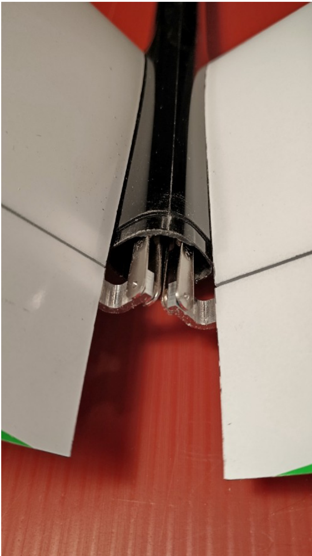
Photo 5: Elevator is using standard metal clevises, easy to remove with a screw driver
