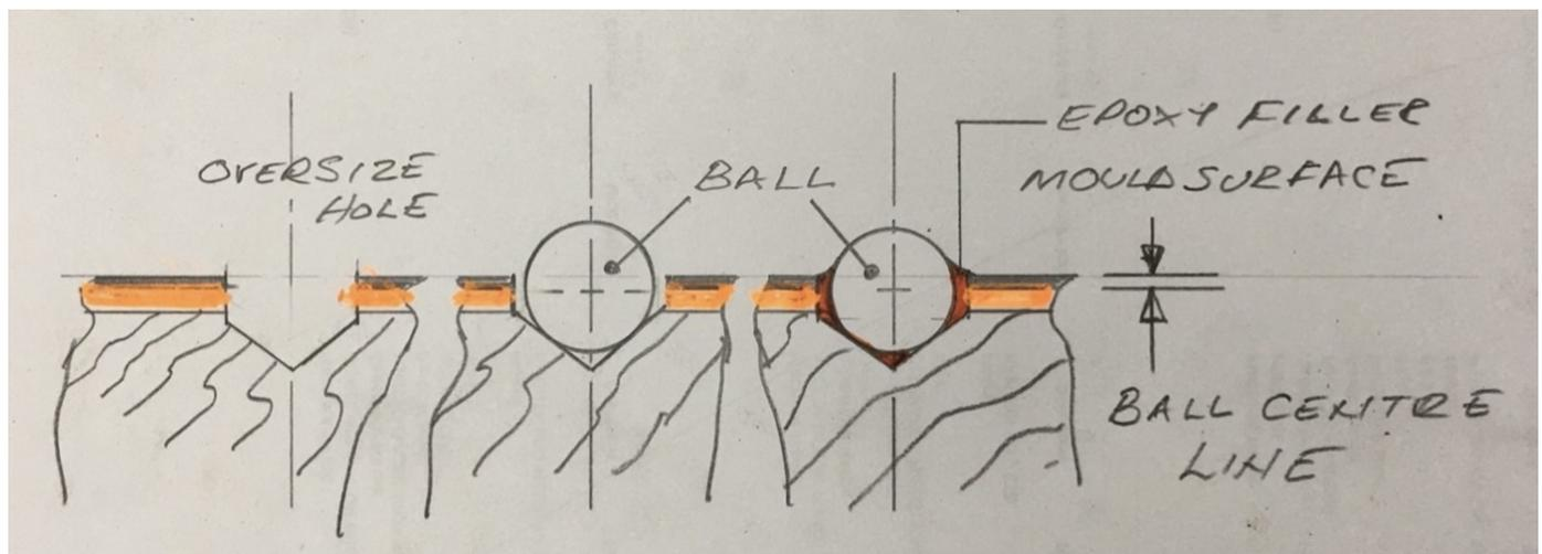
Shallow holes are drilled into the mould surface to allow the balls to settle just below the centre line. Then epoxy is applied to secure them.
