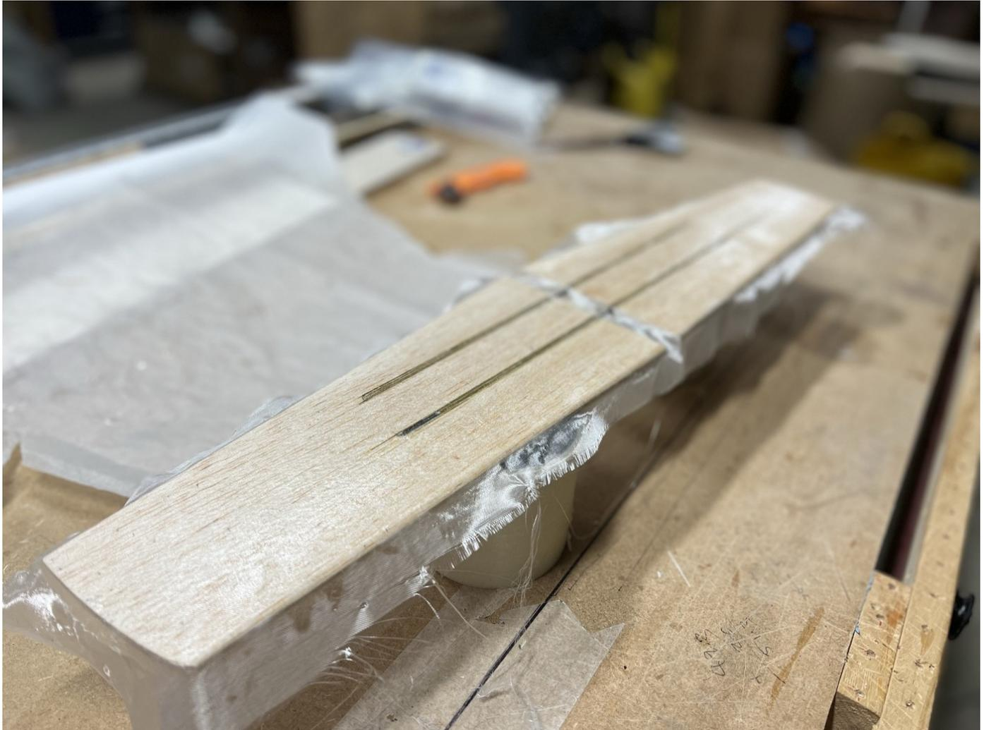
25g/m<sup>2</sup> glass and epoxy top and bottom surface for protection and a little stiffening.
