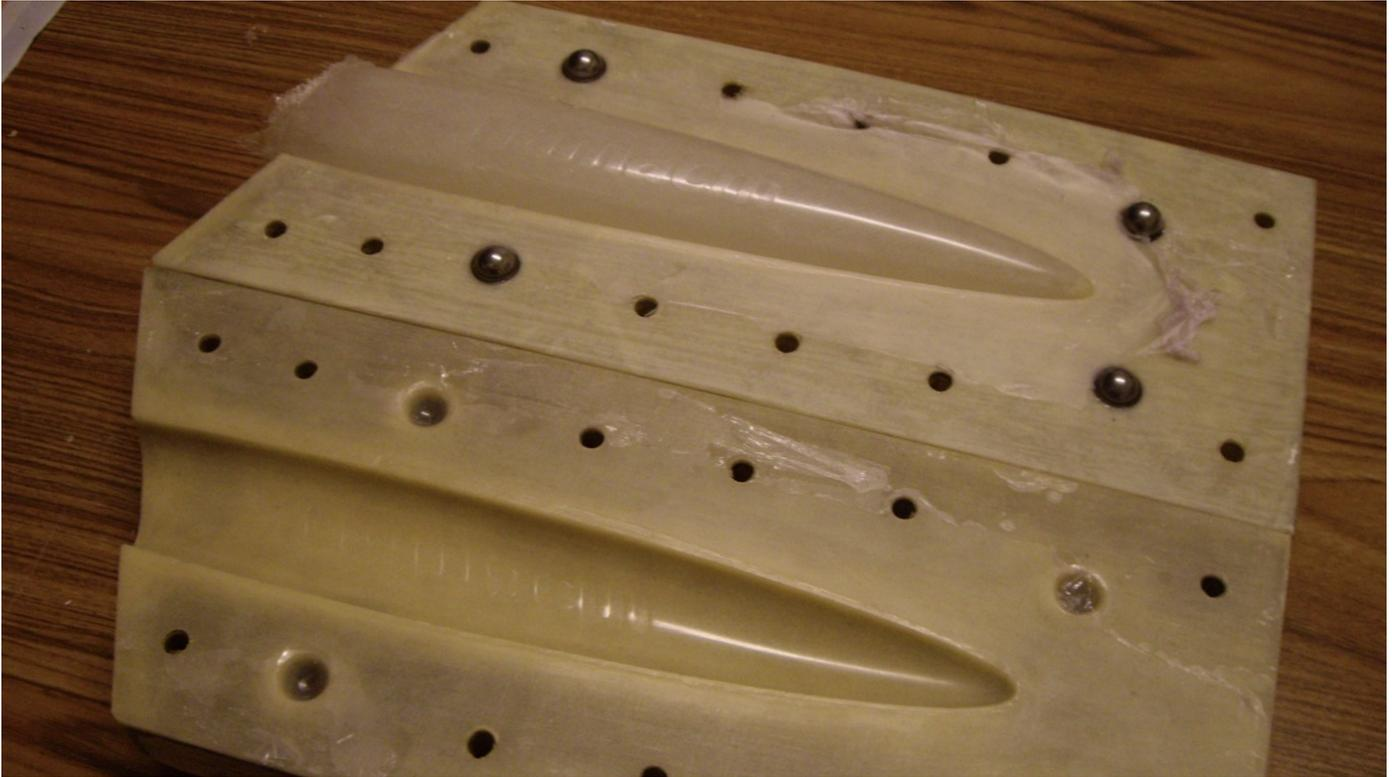
Here the moulds have just been separated from the plug. Note the PVA release agent residue around the edges.
