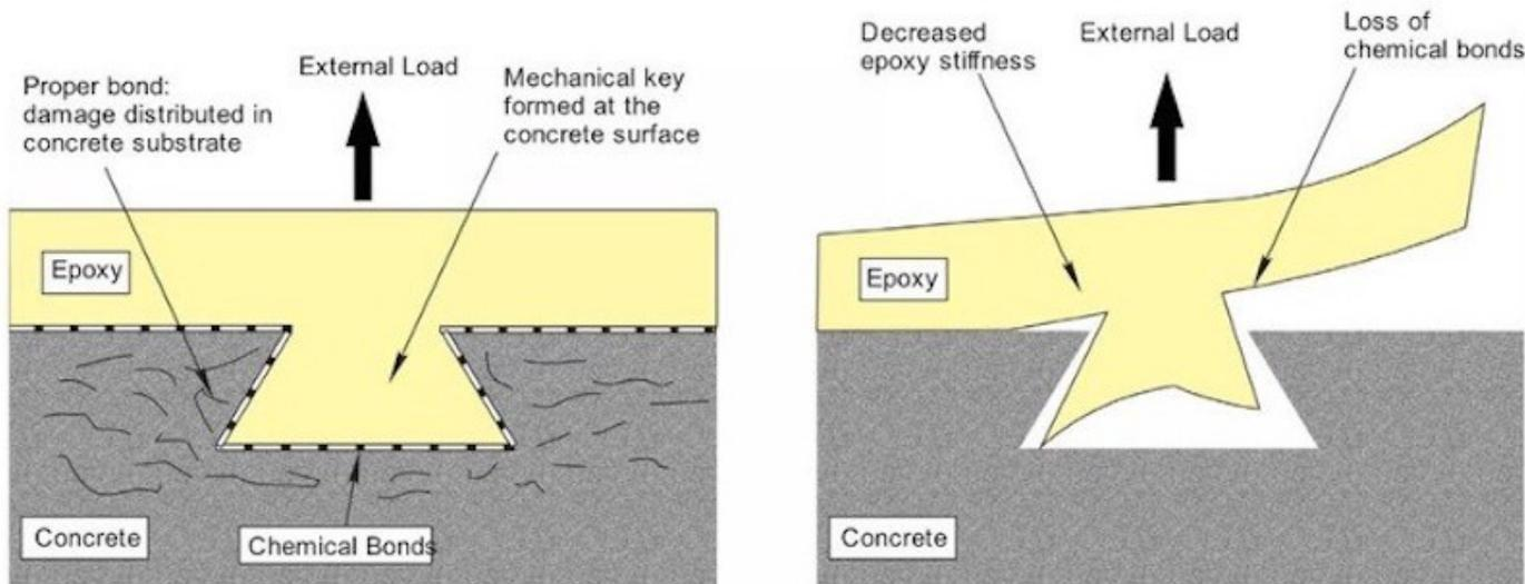
Here is a simple adhesion diagram in this case joining epoxy to concrete but in fact it does not matter too much what the substrates are the effects are the same. (image: Jovan Tatar et al)
