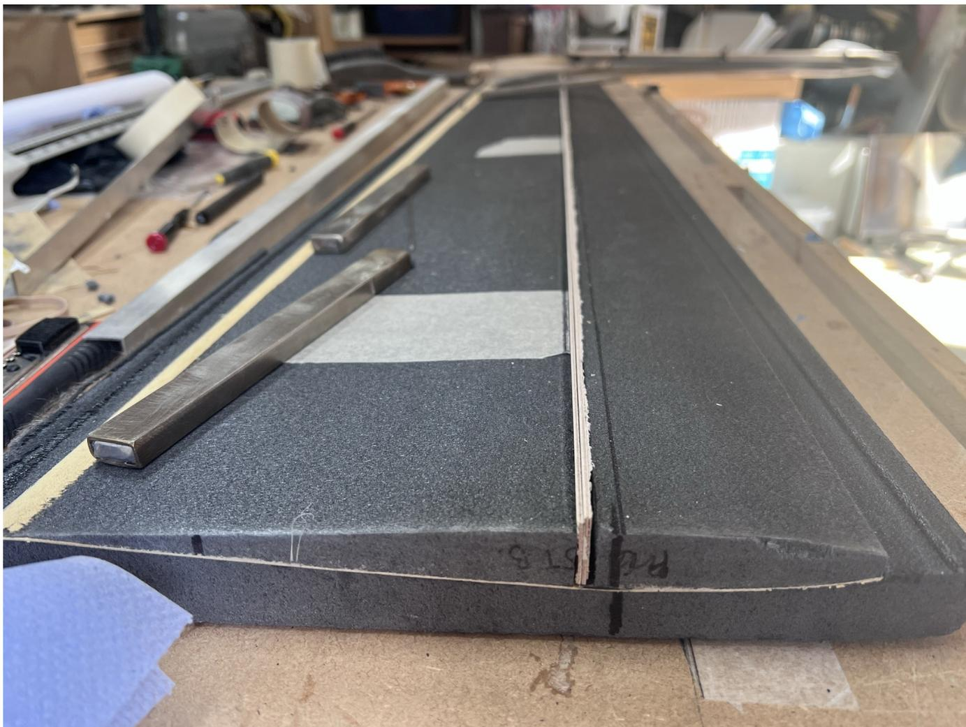
Slowly excavate the foam all the way down to the skin/carbon spar cap. Fit your spar and ensure its secured with a good epoxy joint.
