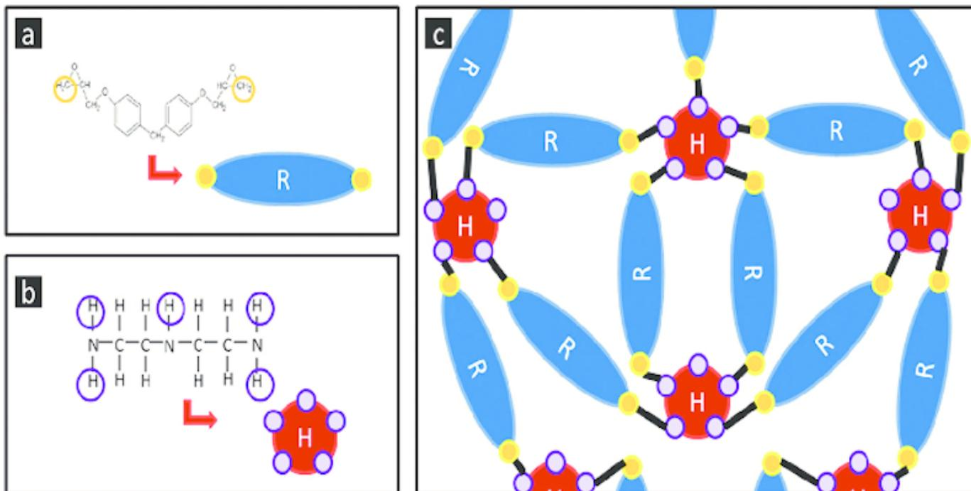
Here is a diagram of the crosslinking that occurs when epoxy substrates are chemically joined for a primary bond. (image: Jinjun Zhang et al)
