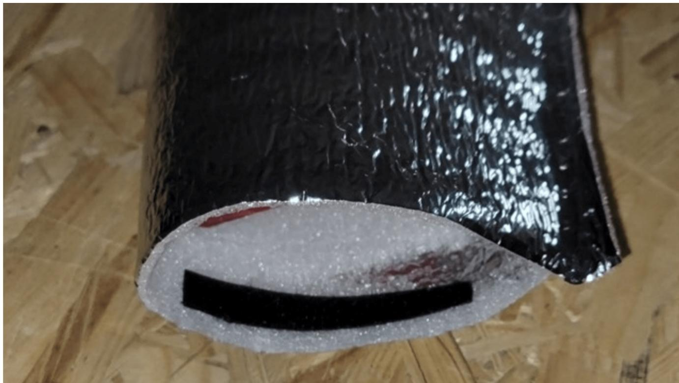
The hook-and-loop method used to seal up the enclosure when the part is inside.
