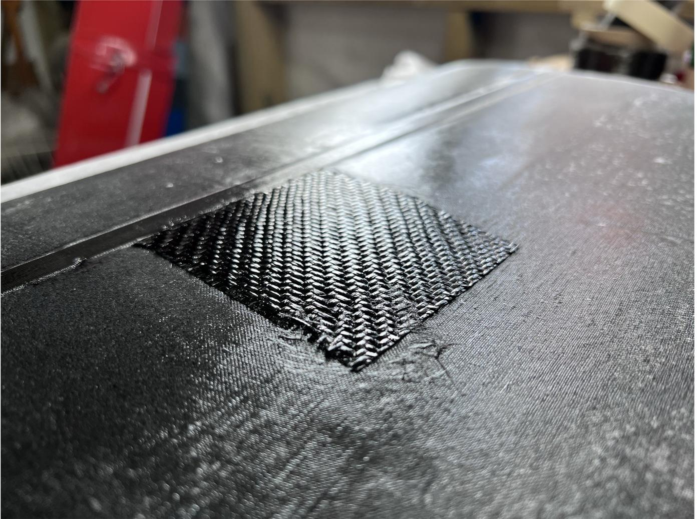
Well wetted, carbon strip visible, carbon reinforcements where the servos will be.
