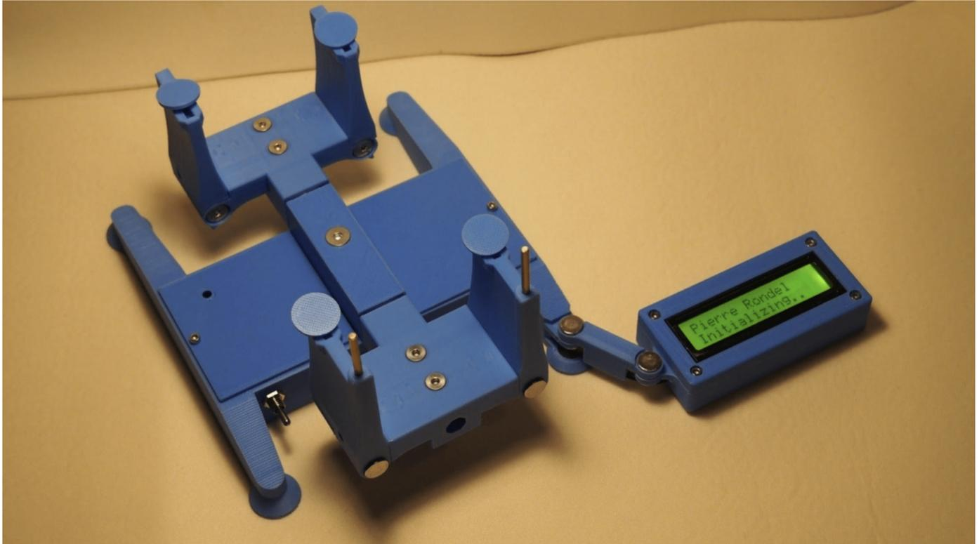
"A good F3F competition plane deserves a good CG setting, which requires the appropriate tool." While not absolutely required to determine your aircraft's centre of gravity, anything which makes it easier and more accurate is an asset. See Resources, below for a link to Pierre Rondel's Digital CG Balancer article. (image/quote: Pierre Rondel)
