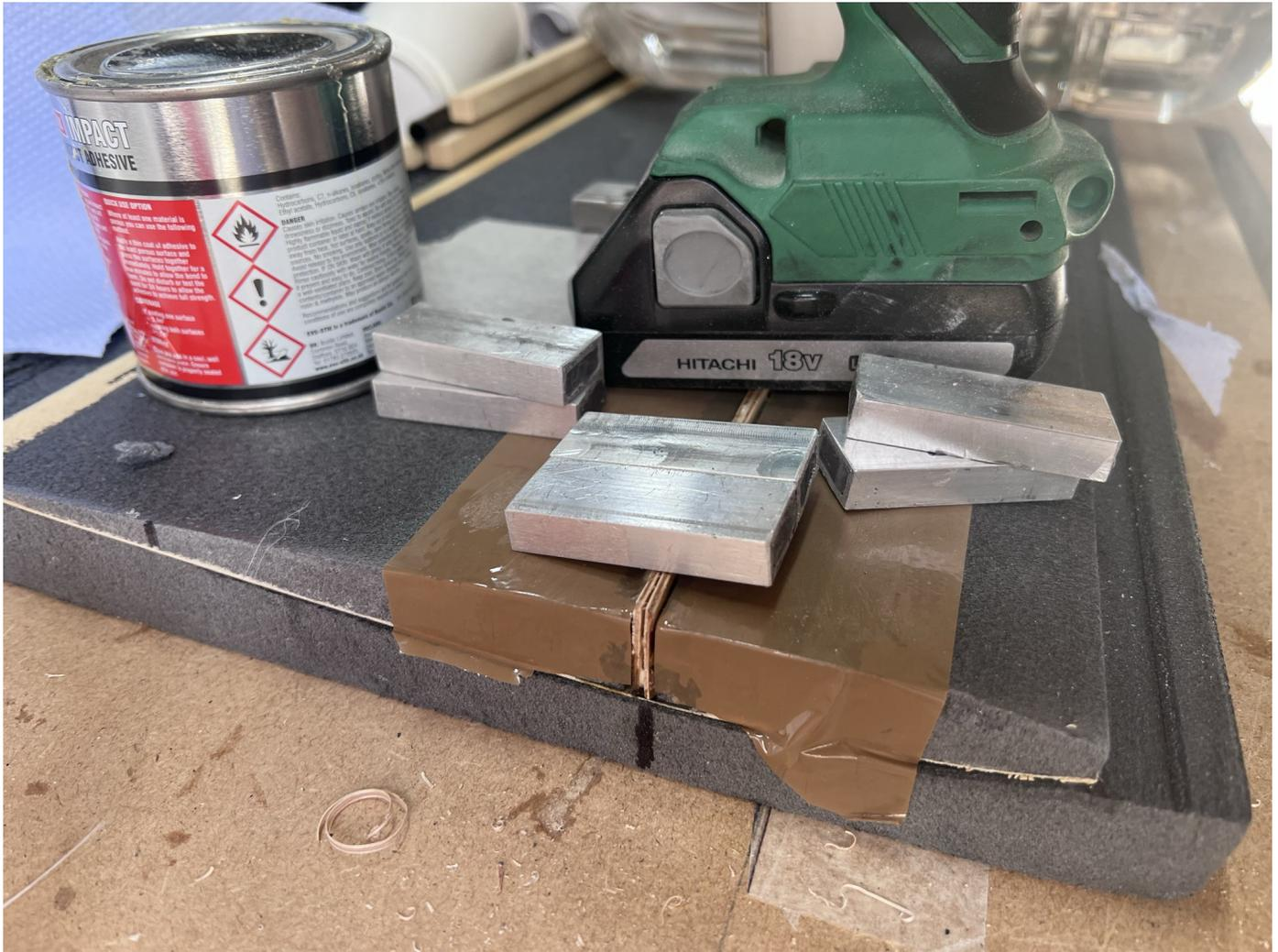
Slot the spar in and wait for the epoxy to cure. Weight down to keep it all tight against the carcass.
