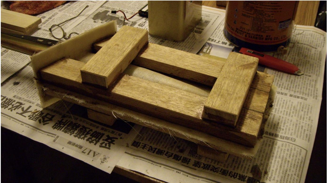
Wow...the nose cone mould is complete now and separated from the plug.
