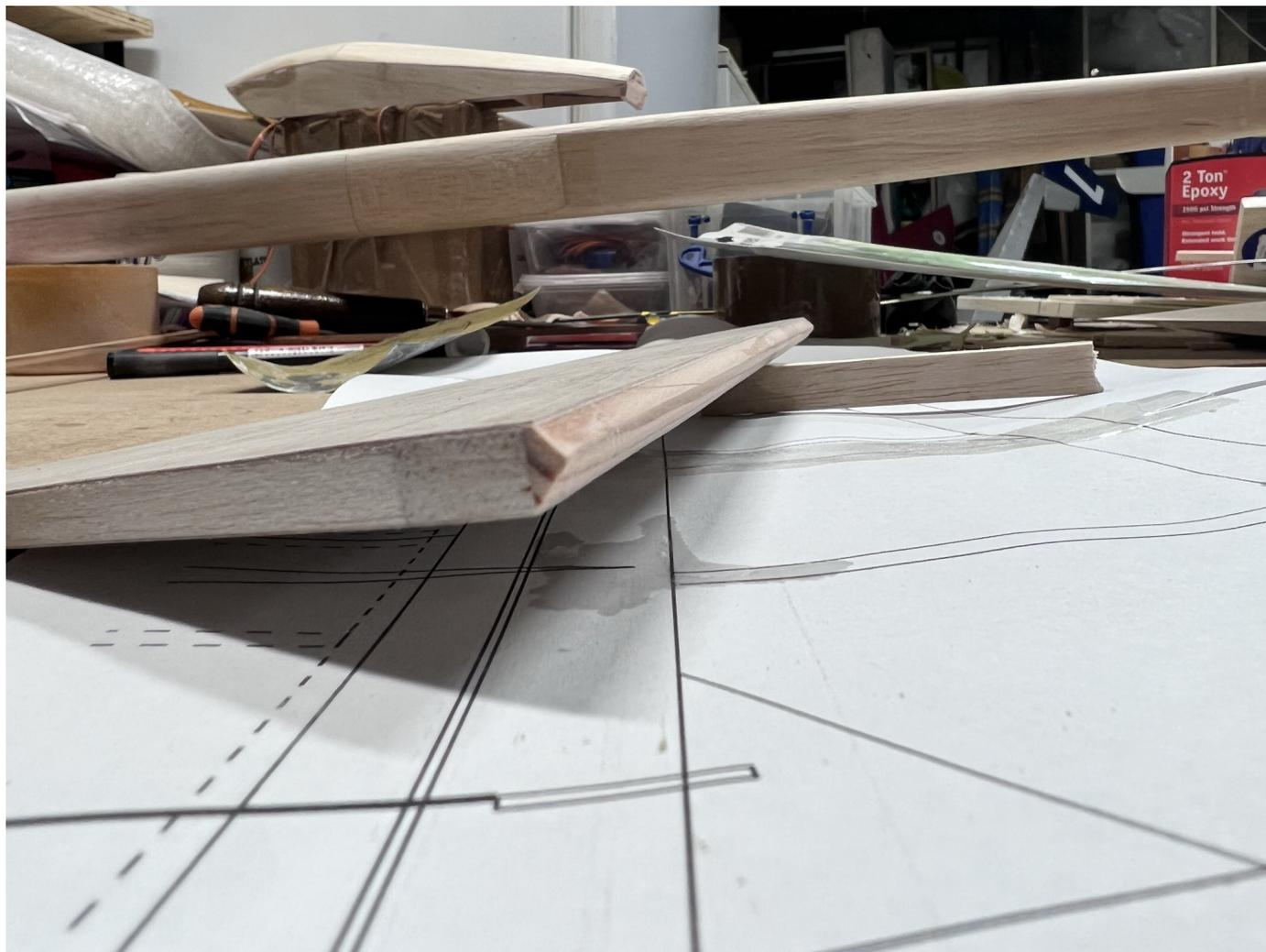
Skinned with 0.6mm ply. The hardwood post gets a bevel to allow for movement once hinged.
