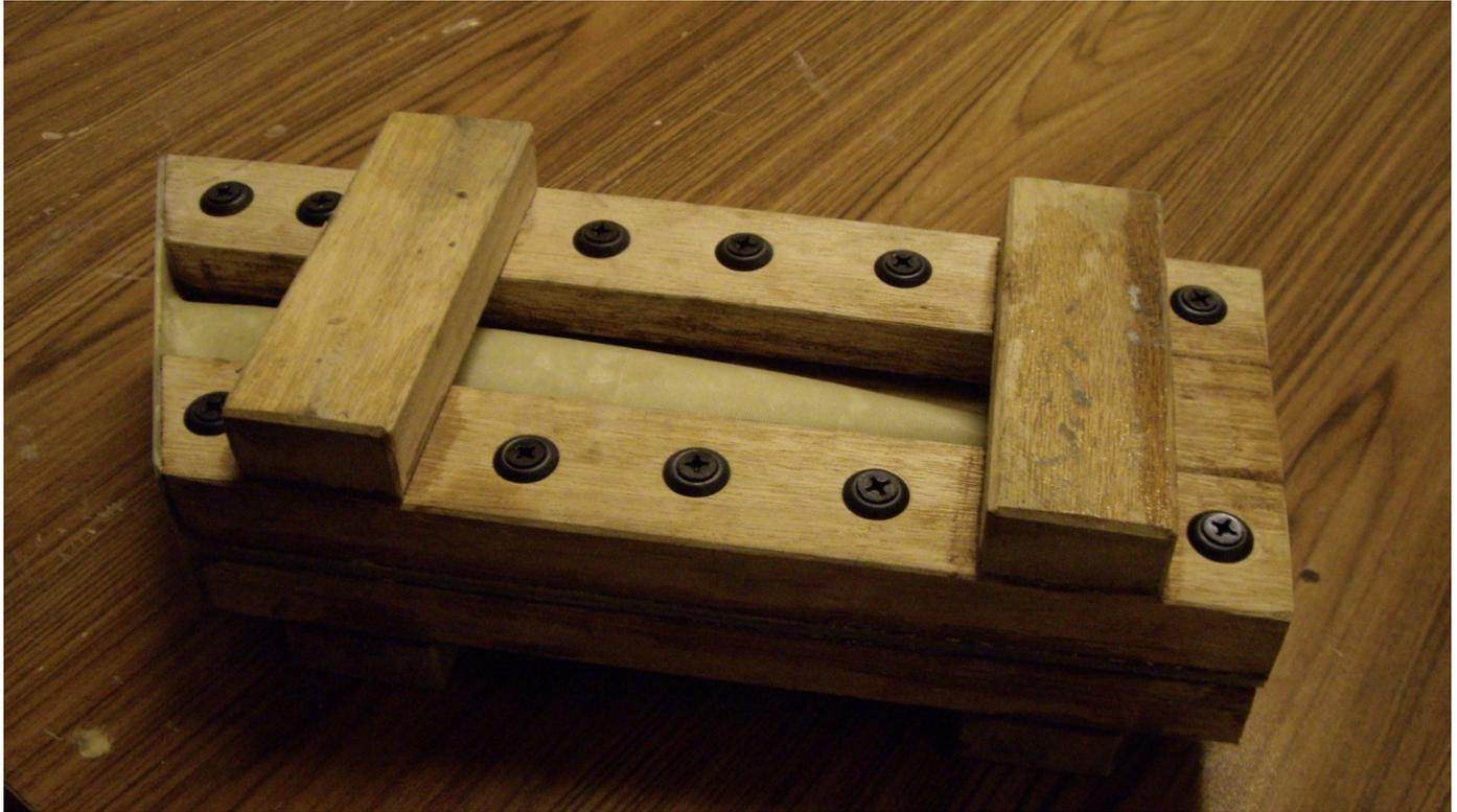
Here the outside ragged glass edges have been trimmed and rounded and the clamping crews inserted.
