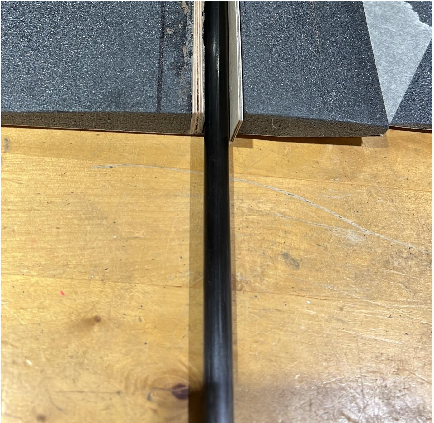
Mark the joiner rebates, excavate and rough fit the joiner tube. Walls fitted the same way as the spars.
