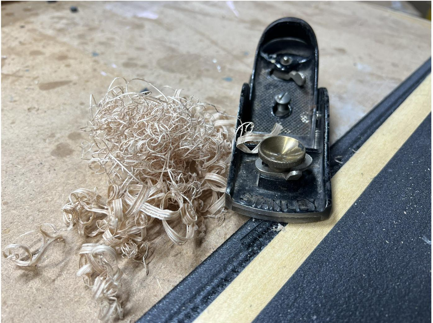
Trim back to flush with a sharp block plane — ‘wafer-thin’, just like Mr. Creosote likes.
