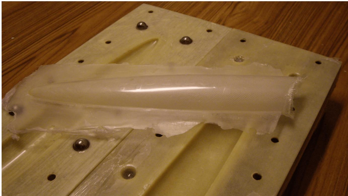
A finished Shinobi nose cone fresh out of the completed nose cone mould.
