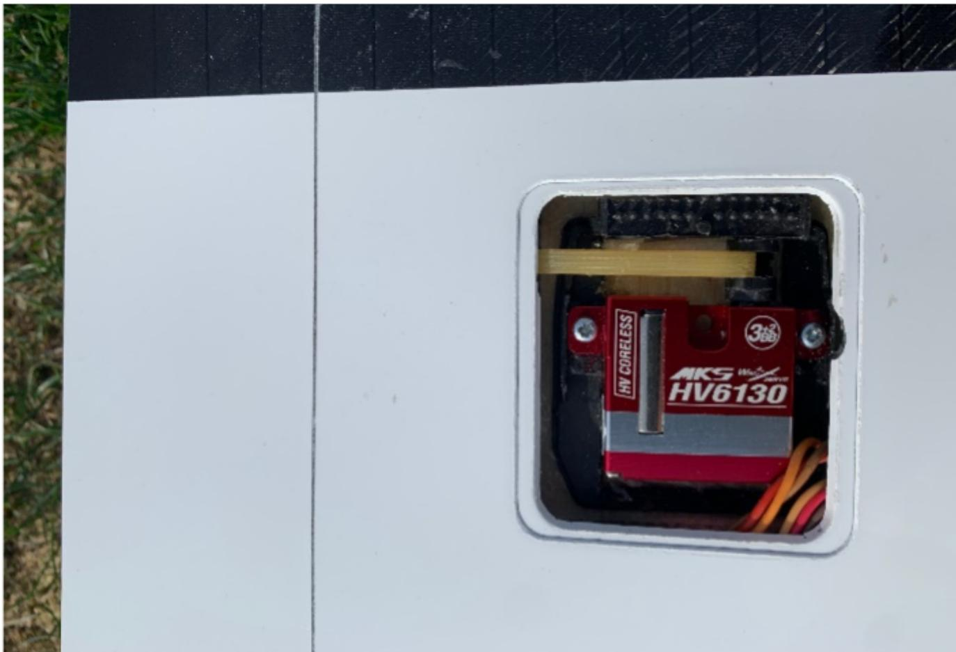
Twister uses an Integrated Drive System (IDS) in wing to eliminate the drag of external control horns.
