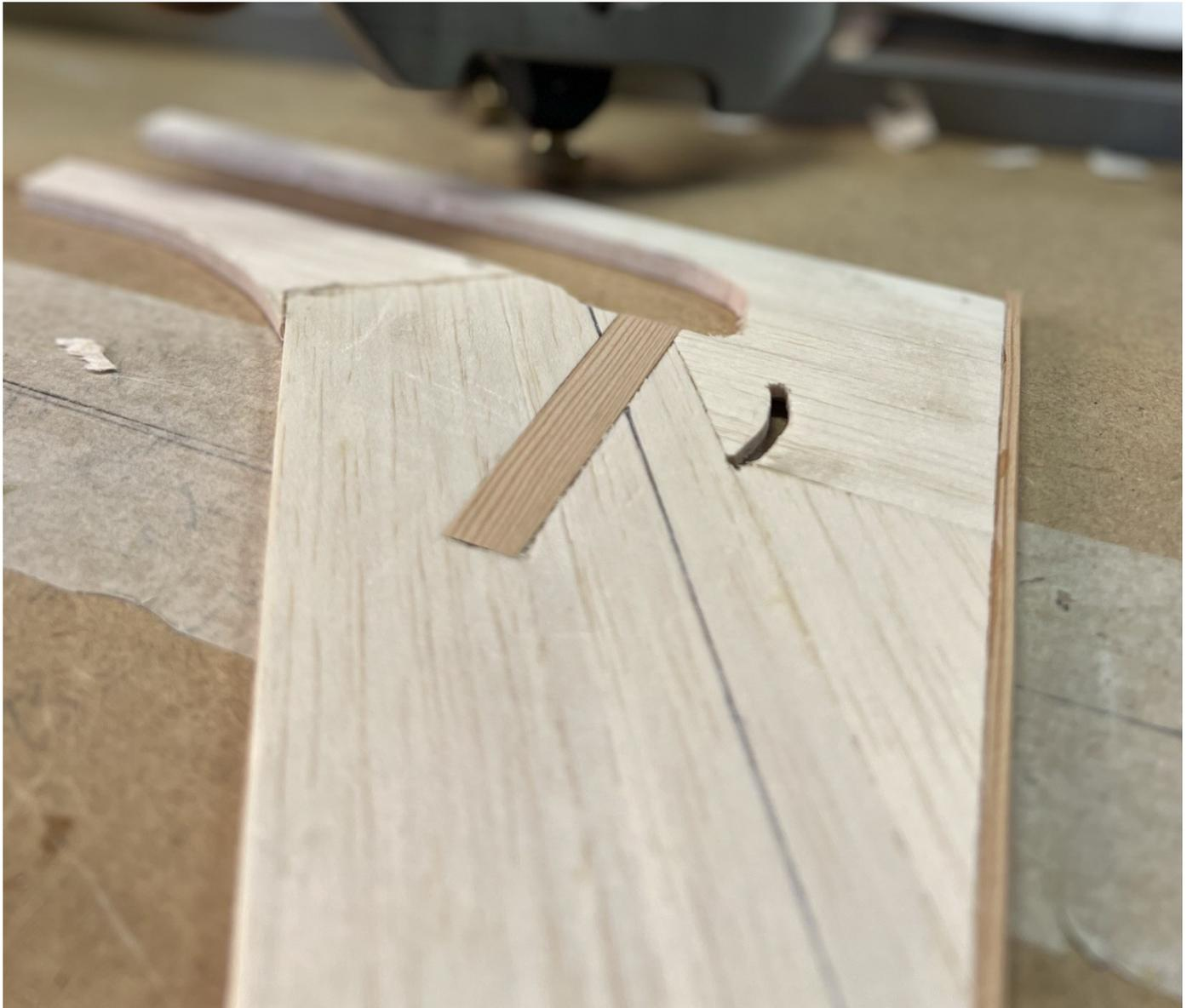
Recessing the spruce upright for the hinge to sit in. The hinge will also be sleeved with brass tube as bearing—there shall be no slop!
