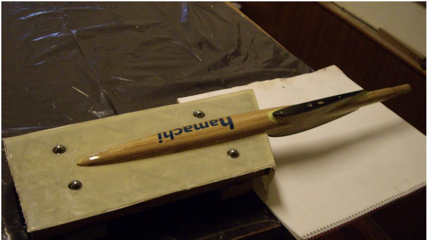
Here the alignment balls have been inserted into the holes and the surrounding gaps are filled with epoxy.
