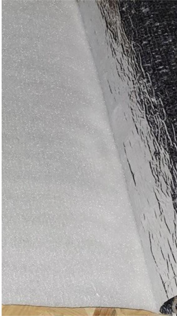
The material is labelled *SmartSHIELD, 3mm, 24in x 25ft Reflective Foam Core Insulation roll, Radiant Barrier, Commercial Grade, Pure Aluminum* (see *Resources*, below, for link) The one side you don't need — the 'inner' side, next to the part the bag encloses — can easily be peeled off. This was easier to do than with the previous product I tested.
