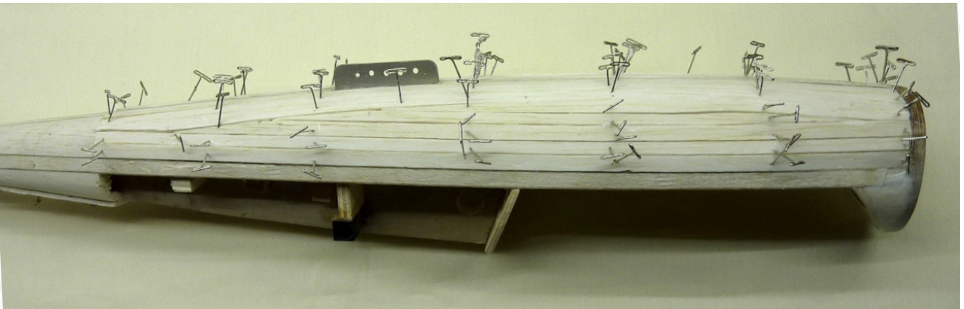
Filled and sanded with two coats of Eze-Kote , before glassing:
