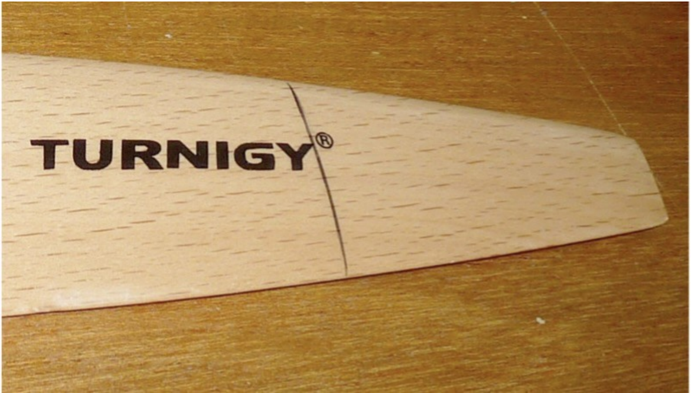
Picture 2: I marked the 75% point out from the centre. Here the diameter was 380mm. (credit: Peter Scott)
