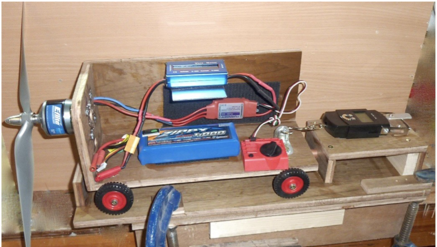
Picture 1: Test rig for motors employing the Martin Phillips design featured in RCM&E. (credit: Peter Scott)
