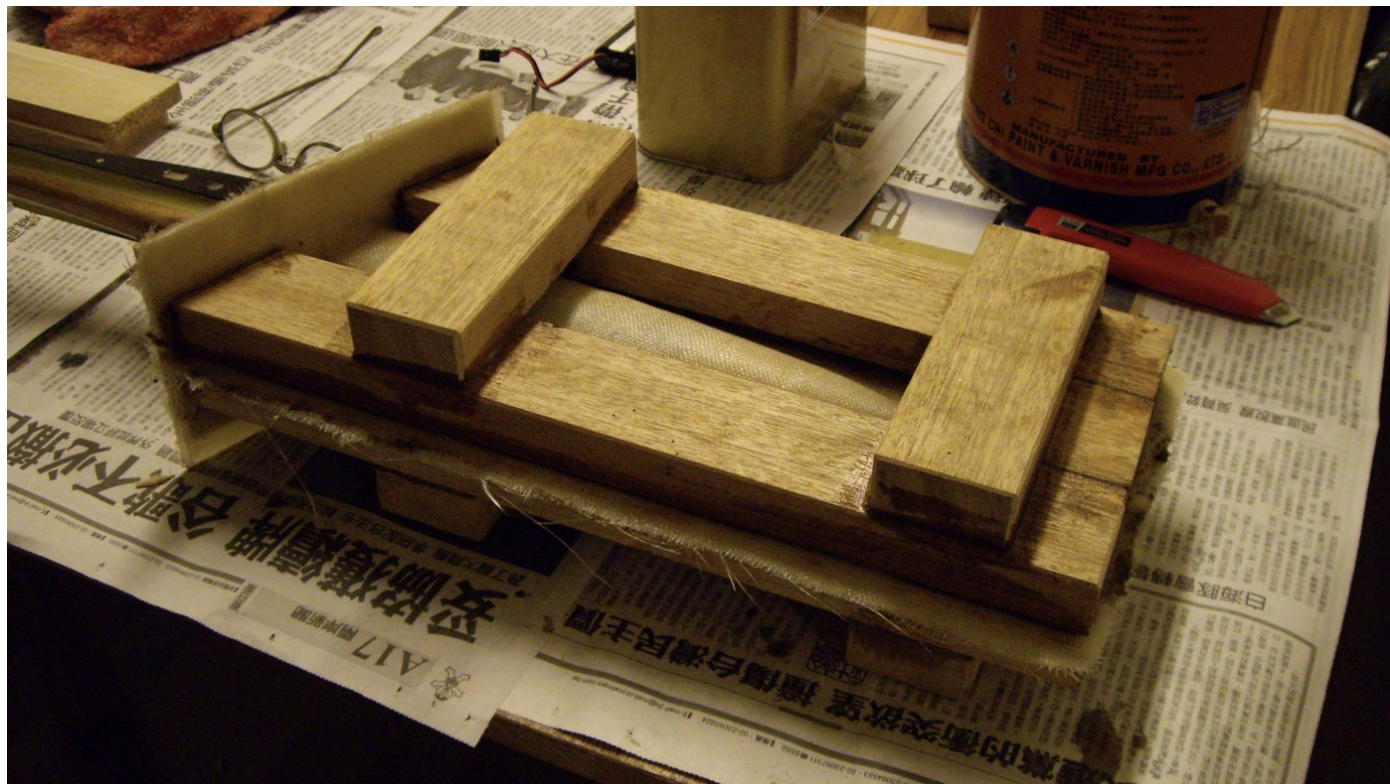
Nosecone mould, untrimmed — note the needle-sharp glass fibres.
