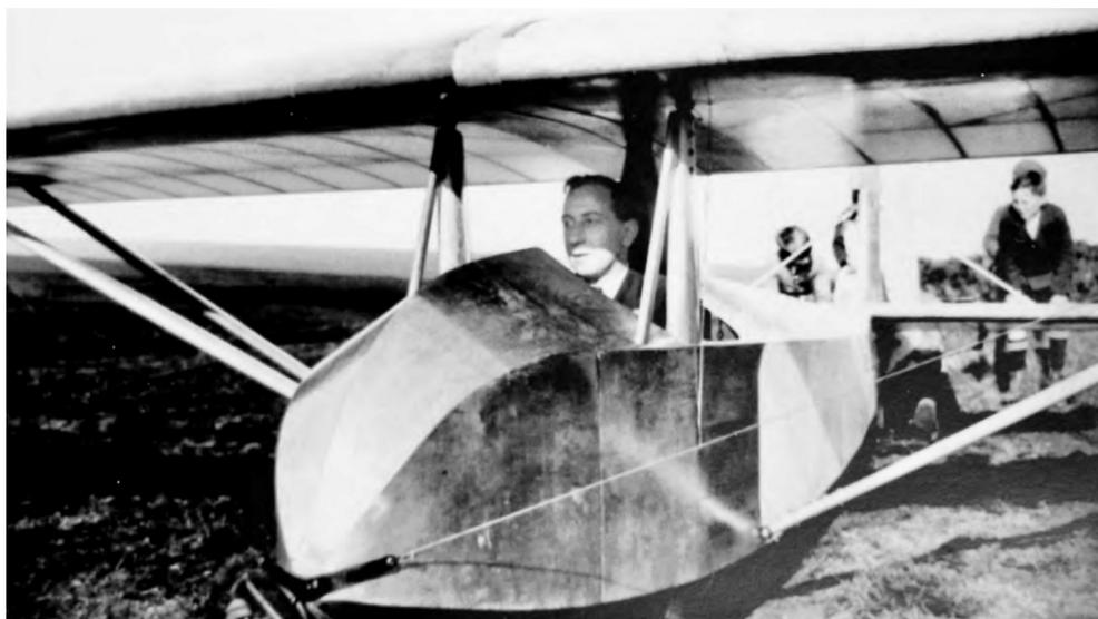
“Slingsby prepares for a bungee launch in his first sailplane, the British Falcon. The steel ring attached to the rubber rope is on the open hook at the nose. Ground crew hold the tail until the rope is stretched sufficiently to launch the sailplane. (Slingsby collection)” (caption: Martin Simons)
