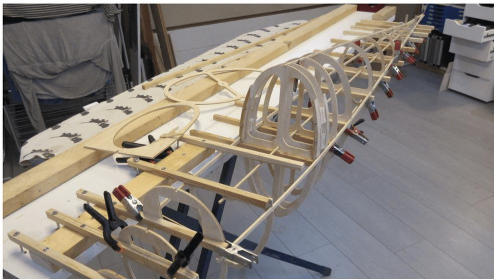
Frames set up on the temporary support battens, right-side up.
