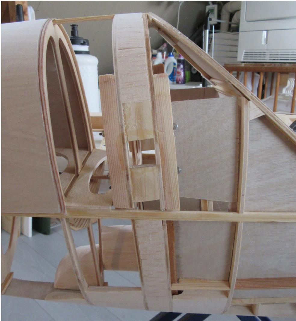
Reinforcement at the wing joiner.
