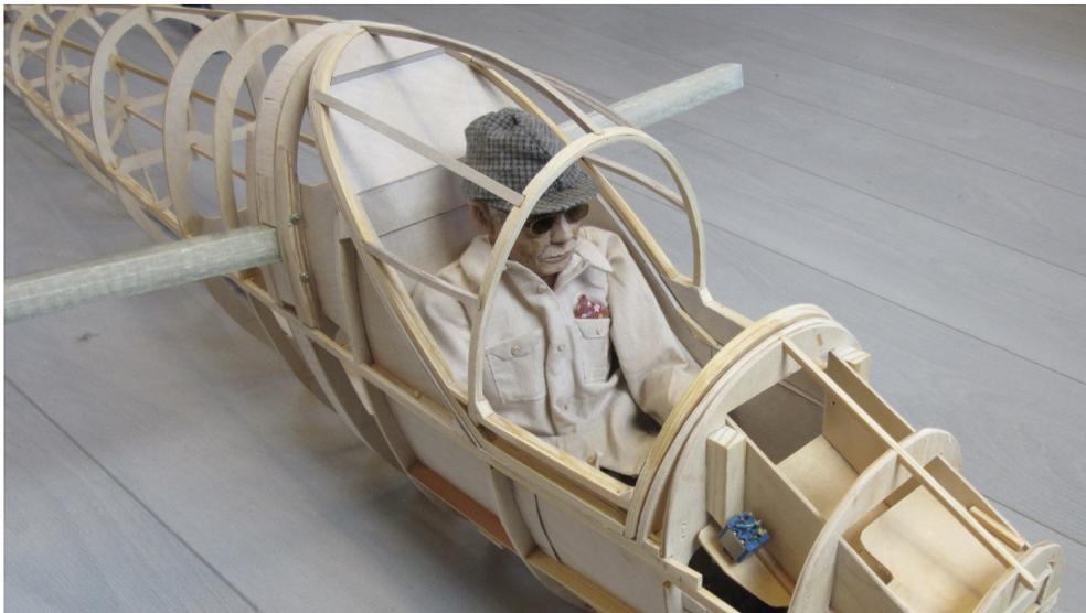
The pilot fits well. On the inside I made a lot of plywood reinforcements.
