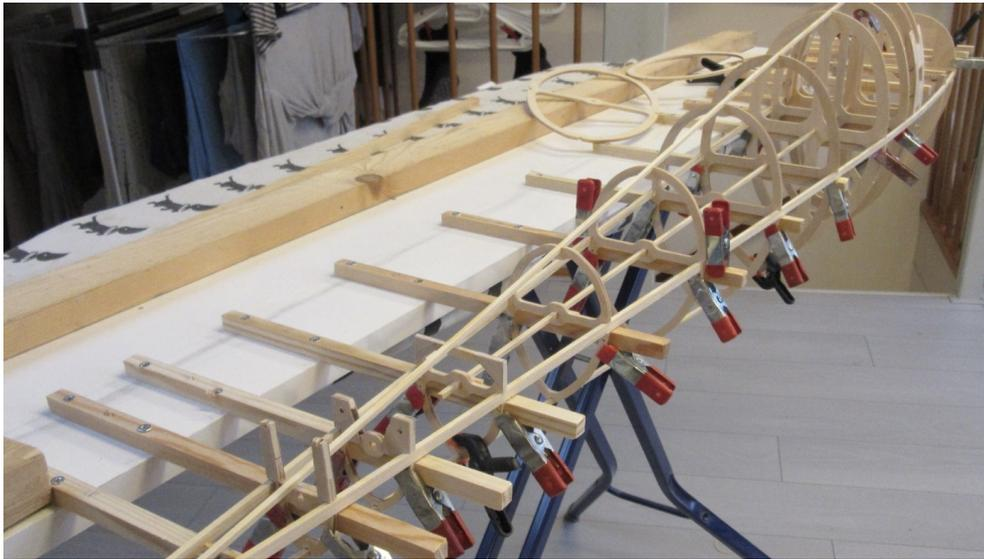
Frames set up, they rest on the central temporary support battens. See also key photo above for a similar view, but with the fuselage right-side up.
