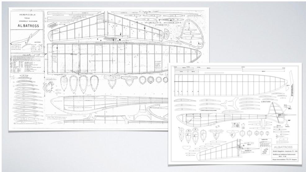
The original Albatross plans from Aeropiccola on the left, and the beautiful new drawings by Roberto Viti from which a DXF can be generated for laser cutting of the parts.
