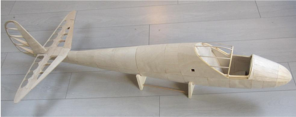
Fuselage and stabiliser almost ready with the wing fairing still to be made.
