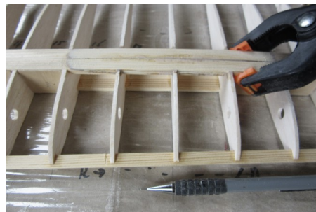
Left: Top spar sawn through and chamfered. | Centre: I glued a thin auxiliary spar under it, to get a stable situation. | Right: New pieces of spar glued in with thickened epoxy, chamfered 1:10.
