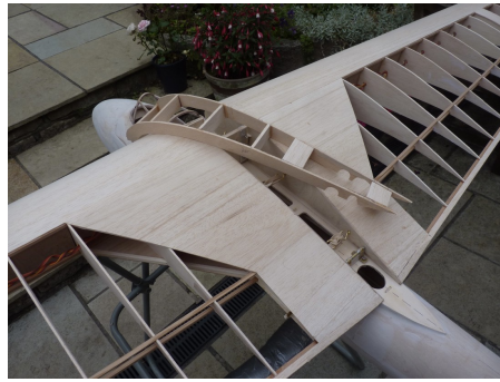
Left: Early stage of wing construction: fitting the sub spars to form an I-beam. | Centre: Details of the wing joiner box. | Right: Making up the inter-wing fairing.
