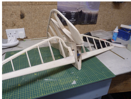
Left: Planking and filling completed, with the temporary formers in the cockpit removed and the interior glassed. | Centre: The rudder is built 'in the hand'. | Right: The complete tail unit prior to fitting.
