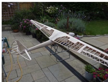
Left: Smoothing the fit of the fairing with car body filler. | Centre: Wing nearing completion. | Right: The Rhönadler airframe, complete & ready for covering.
