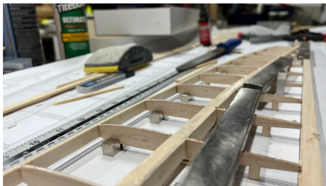
Cube magnets hold the rib stand-offs/legs square.
