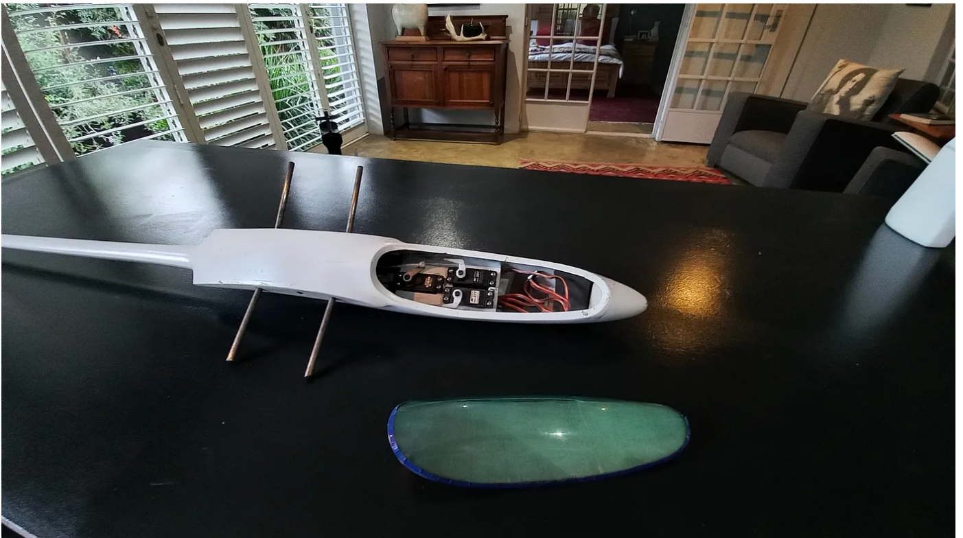
Here you can see the heavy duty 6mm wing joiners in the South African version of the Brillant. (credit: Jan Sime)
