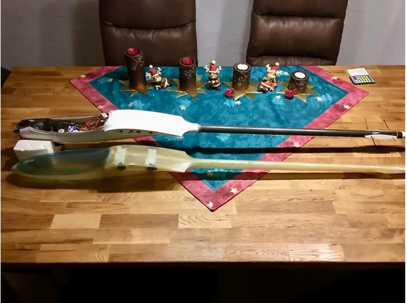
Fishing rod tail boom in the back, laminated version with integrated tail boom in the front. (credit: Abbakus / RC-Network.de)
