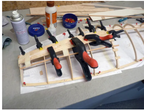
Left: The basic structure of the first of the fuselage half-shells is where it begins. | Centre: The front half of the fuselage is planked with 1.5mm ply: tedious but strong! | Right: The second half is built over the first, making sure to keep it all straight.
