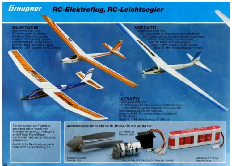
Left: Silentius 86 was a quality Graupner kit. (credit: author) | Right: The 1989 Graupner catalogue showed that the Mosquito, Ultra-Fly and Silentius 86 now had a common drive-train based on the geared Speed 600 and seven 1.4Ah NiCads. (credit: Graupner)
