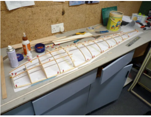
Left: The basic structure of the first of the fuselage half-shells is where it begins. | Centre: The front half of the fuselage is planked with 1.5mm ply: tedious but strong! | Right: The second half is built over the first, making sure to keep it all straight.
