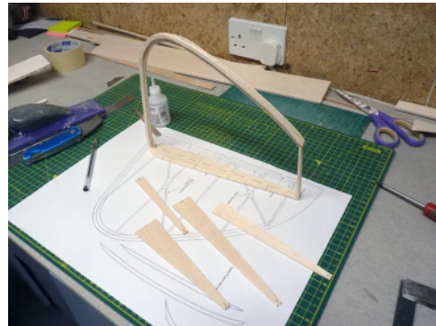
Left: Tailplane complete. | Centre: First stages of the fin construction. | Right: Setting up the rudder cable guides before sheeting the rear of the fuselage.
