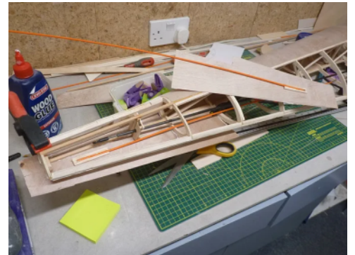
Left: Tailplane complete. | Centre: First stages of the fin construction. | Right: Setting up the rudder cable guides before sheeting the rear of the fuselage.
