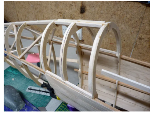
Left: The basic structure of the first of the fuselage half-shells is where it begins. | Centre: The front half of the fuselage is planked with 1.5mm ply: tedious but strong! | Right: The second half is built over the first, making sure to keep it all straight.
